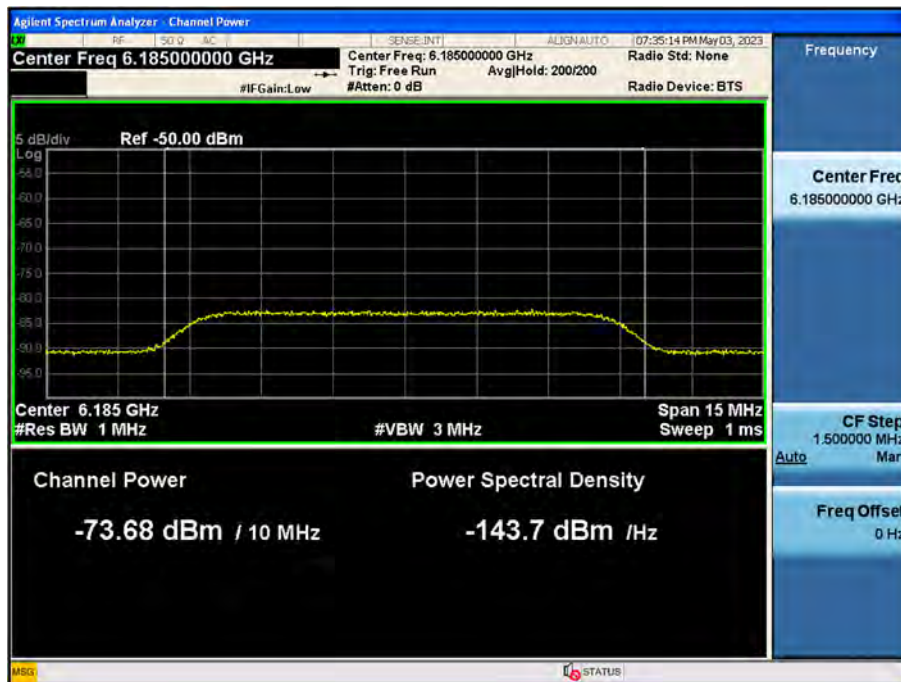
802.11ax HE160 Ch.47(6185 MHz) Detection Level
