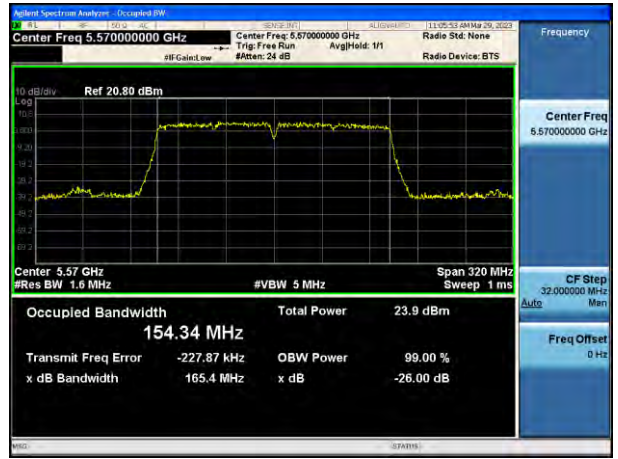
802.11ac_VHT160 UNII 2A BAND 26 dB Bandwidth (CH 114)
