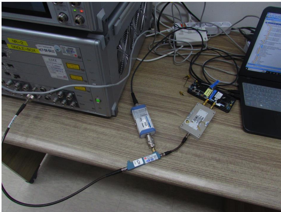
Test setup photo-3 (7-1(b) 5G Sub 6 setup)
