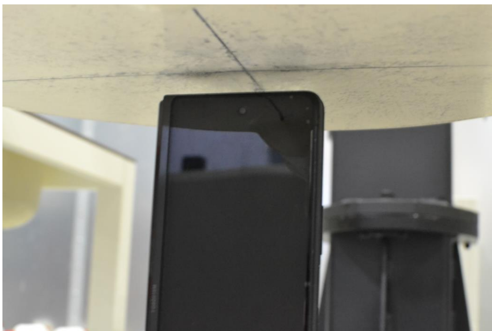
SAR Test Setup Photo 10– Closed Configuration (Handset) Top Edge at 10 mm
