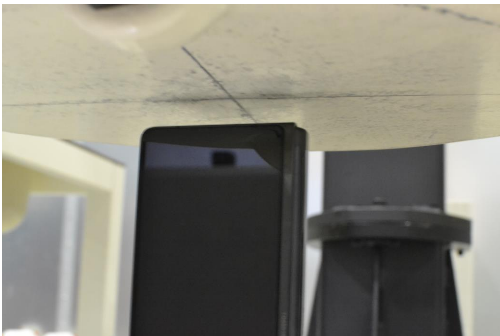
SAR Test Setup Photo 12– Closed Configuration (Handset) Bottom Edge at 12 mm
