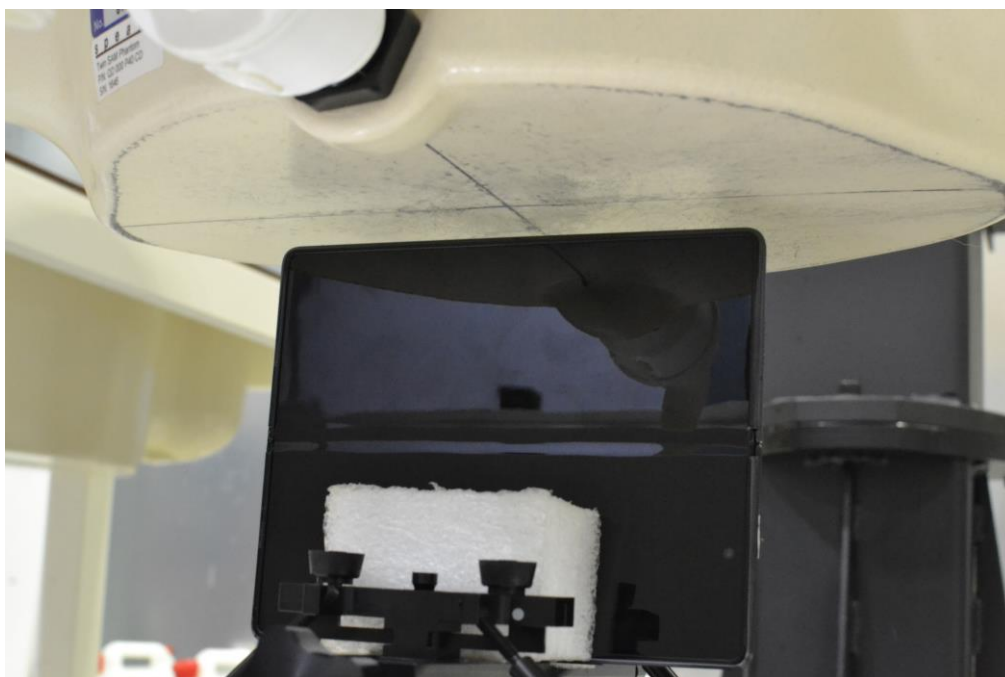
SAR Test Setup Photo 32– Open Configuration (UMPC) Left Edge at 10 mm
