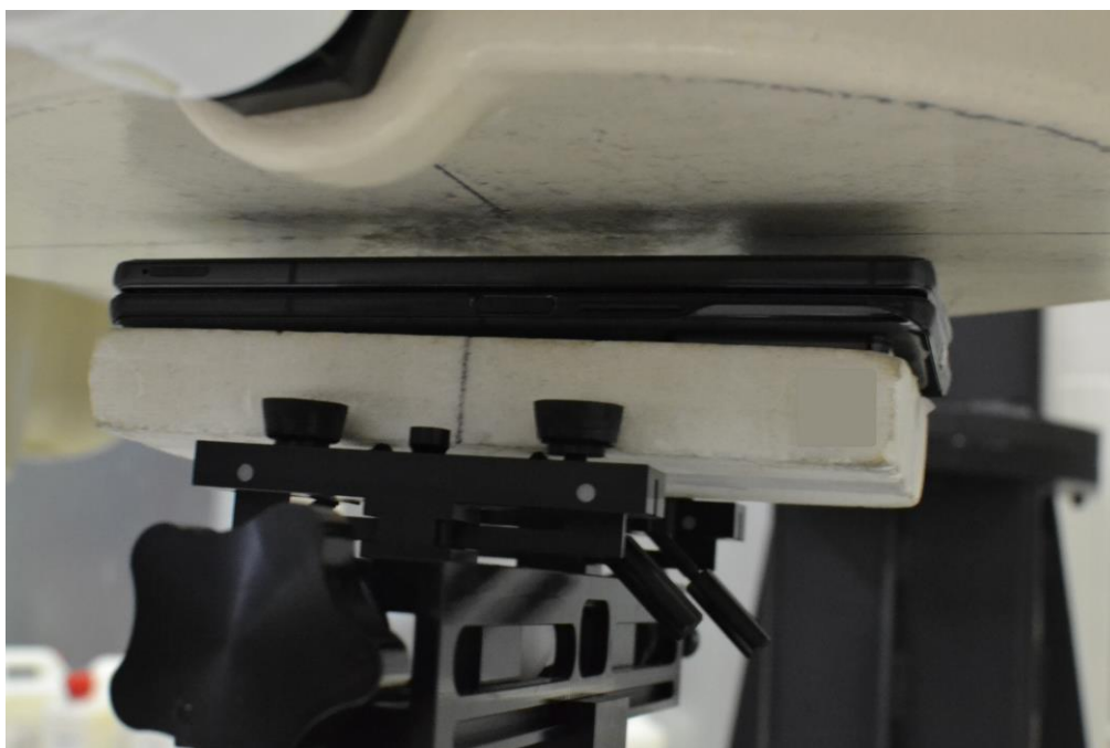
SAR Test Setup Photo 8– Closed Configuration (Handset) Front Side at 10 mm
