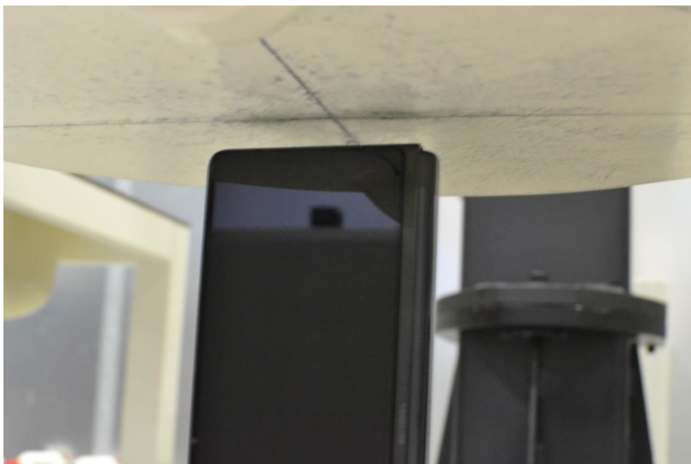
SAR Test Setup Photo 13– Closed Configuration (Handset) Bottom Edge at 10 mm
