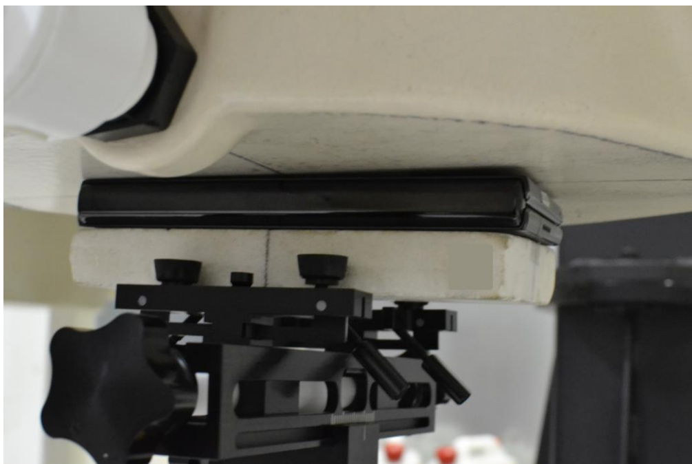
SAR Test Setup Photo 7– Closed Configuration (Handset) Back Side at 0 mm
