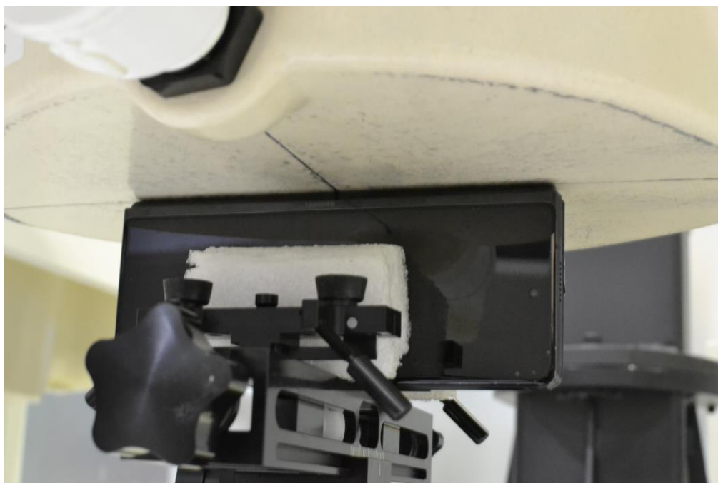
SAR Test Setup Photo 18– Closed Configuration (Handset) Left Edge at 0 mm
