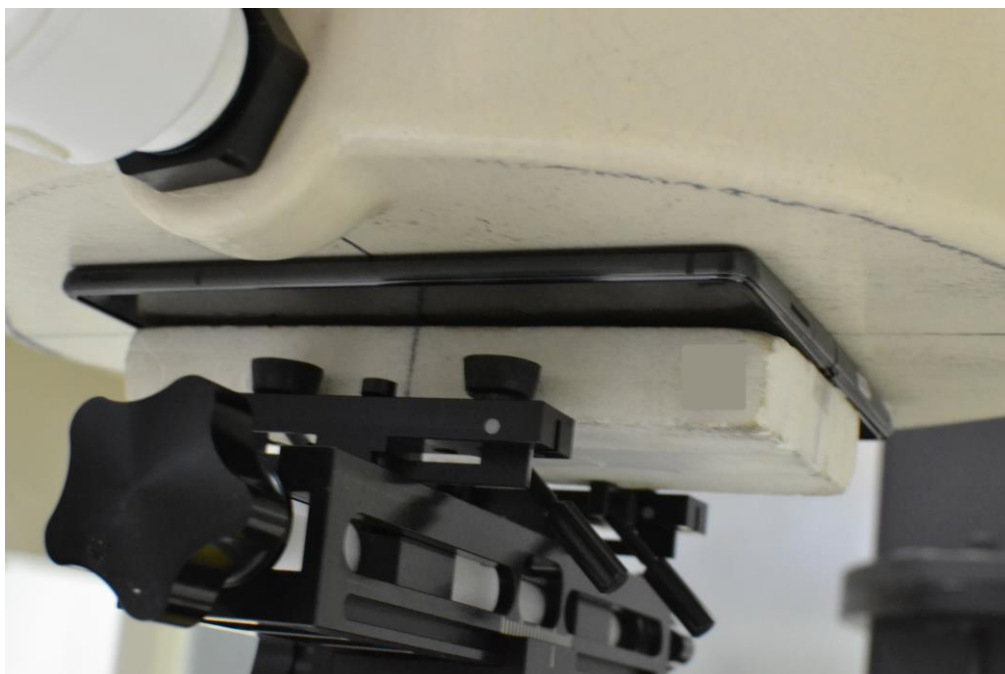
SAR Test Setup Photo 21– Open Configuration (UMPC) Back Side at 0 mm
