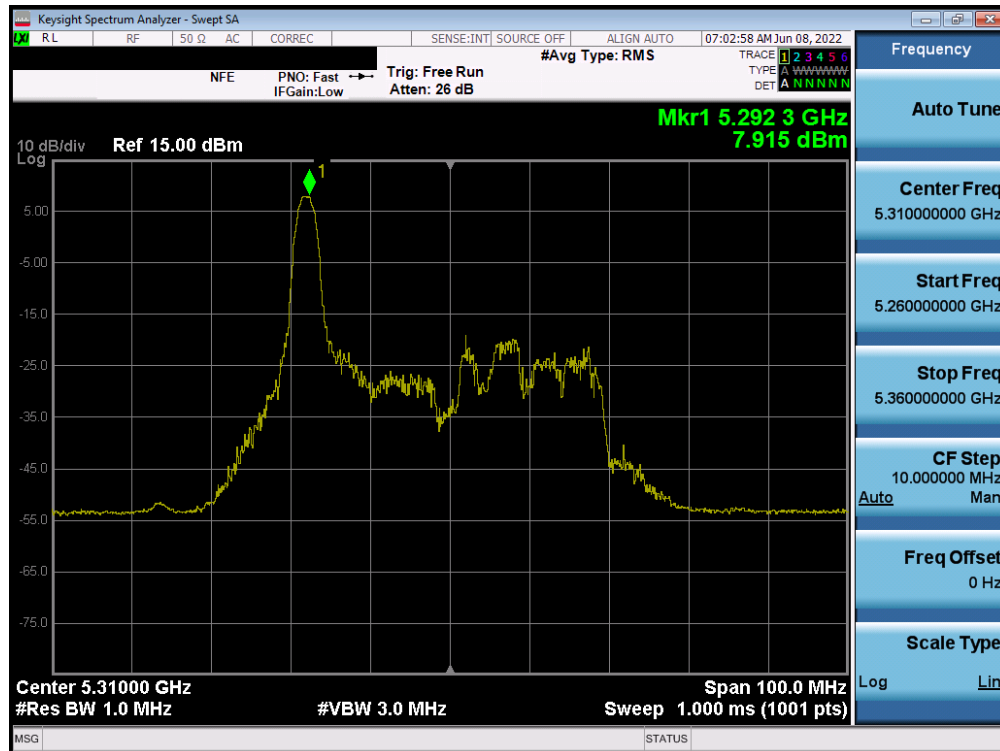
Plot 7-169. Power Spectral Density Plot SISO ANT1 (40MHz BW 802.11ax – 26 Tones (UNII Band 2A) – Ch. 62)
