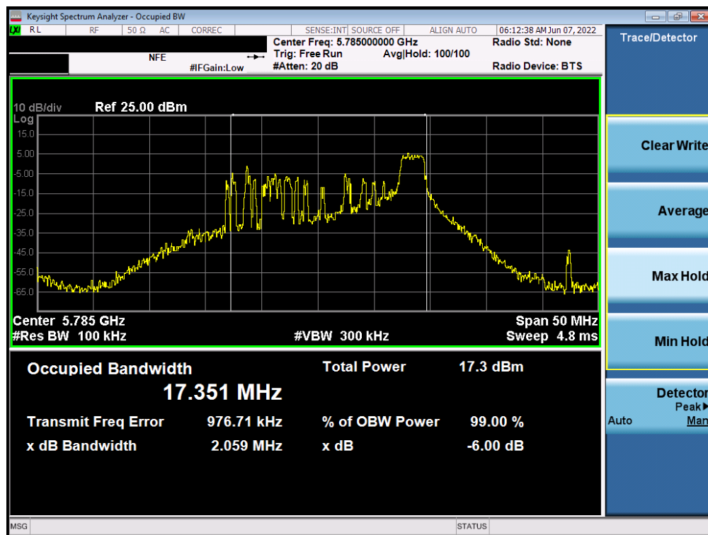
Plot 7-130. 6dB Bandwidth Plot ANT2 (20MHz BW 802.11ax – 26 Tones (UNII Band 3) – Ch. 157)
