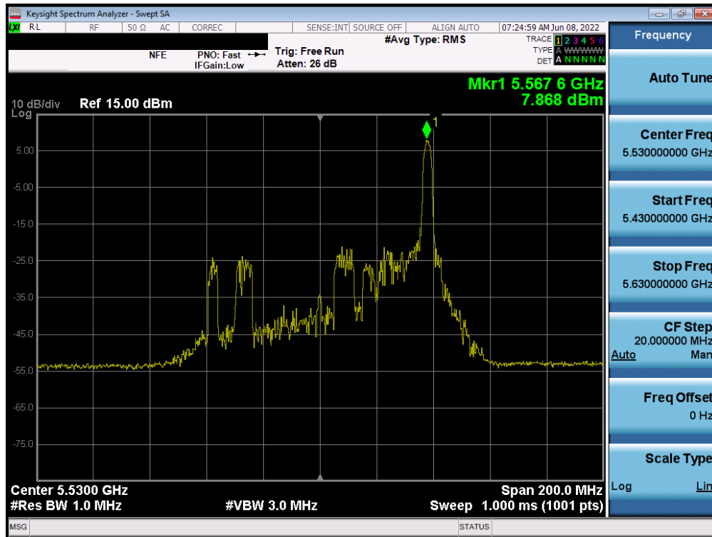
Plot 7-177. Power Spectral Density Plot SISO ANT1 (80MHz BW 802.11ax – 26 Tones (UNII Band 2C) – Ch. 106)
