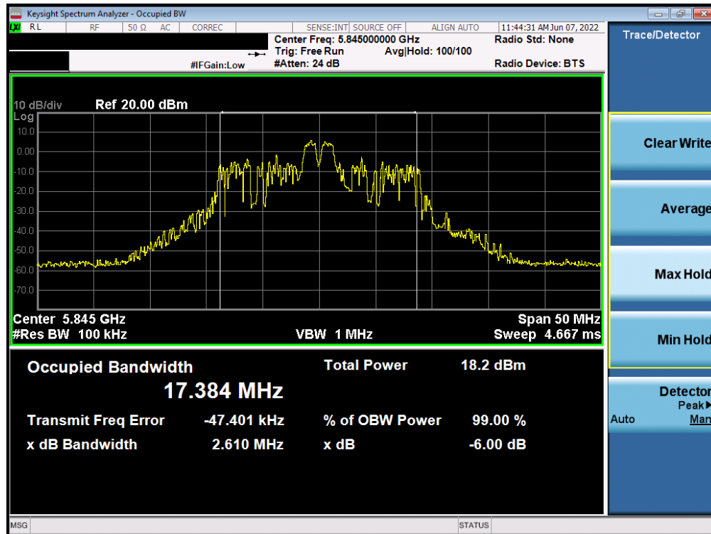
Plot 7-135. 6dB Bandwidth Plot ANT2 (20MHz BW 802.11ax – 26 Tones (UNII Band 3/4) – Ch. 169)
