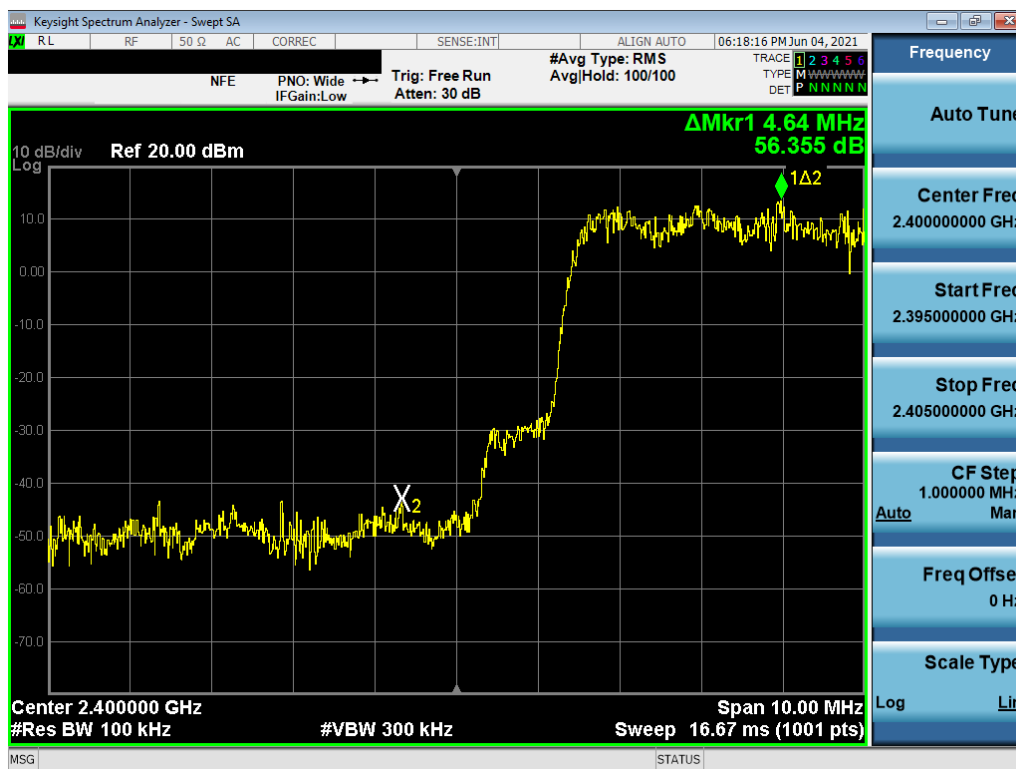
Plot 7-123. Band Edge Plot (Bluetooth with Hopping Enabled, iPA, 3 Mbps – Ch.0) – ANT1
