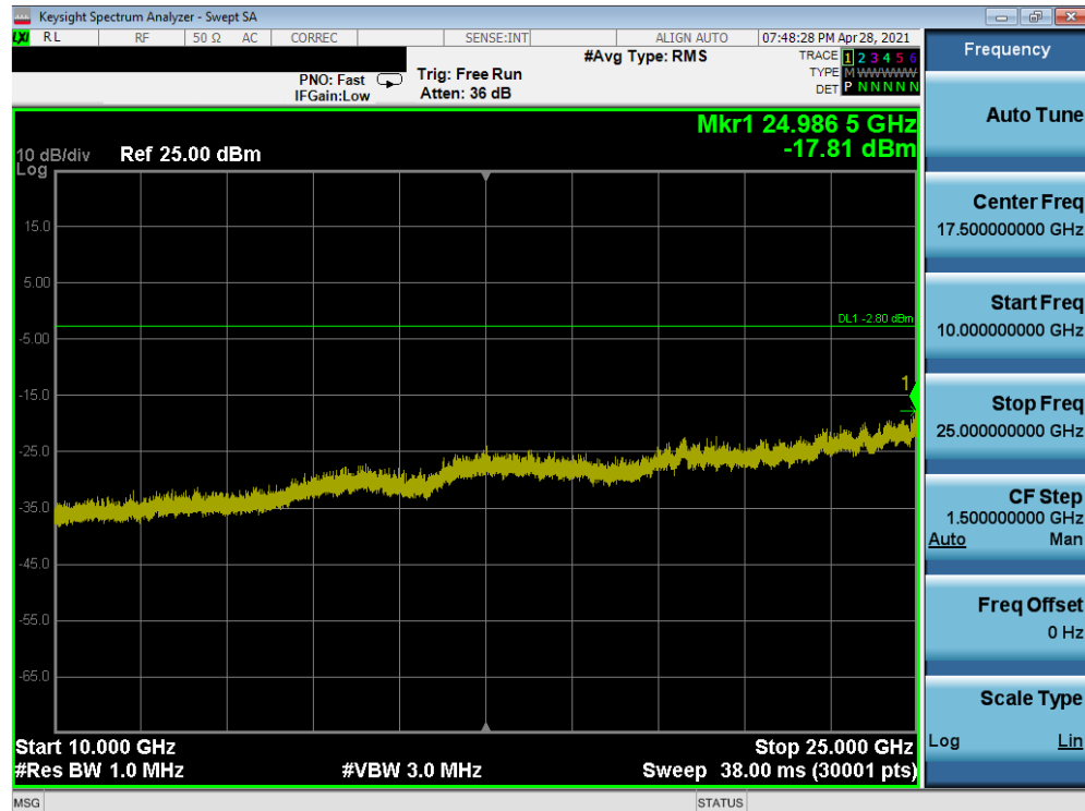
Plot 7-158. Conducted Spurious Plot (Bluetooth, 1Mbps – Ch. 78, ePA) – ANT1
