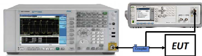
Figure 7-6. Test Instrument & Measurement Setup
