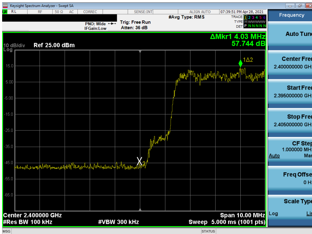
Plot 7-119. Band Edge Plot (Bluetooth with Hopping Enabled, ePA, 3 Mbps – Ch.0) – ANT1
