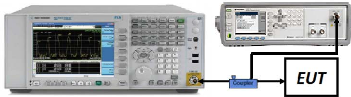
Figure 7-4. Test Instrument & Measurement Setup
