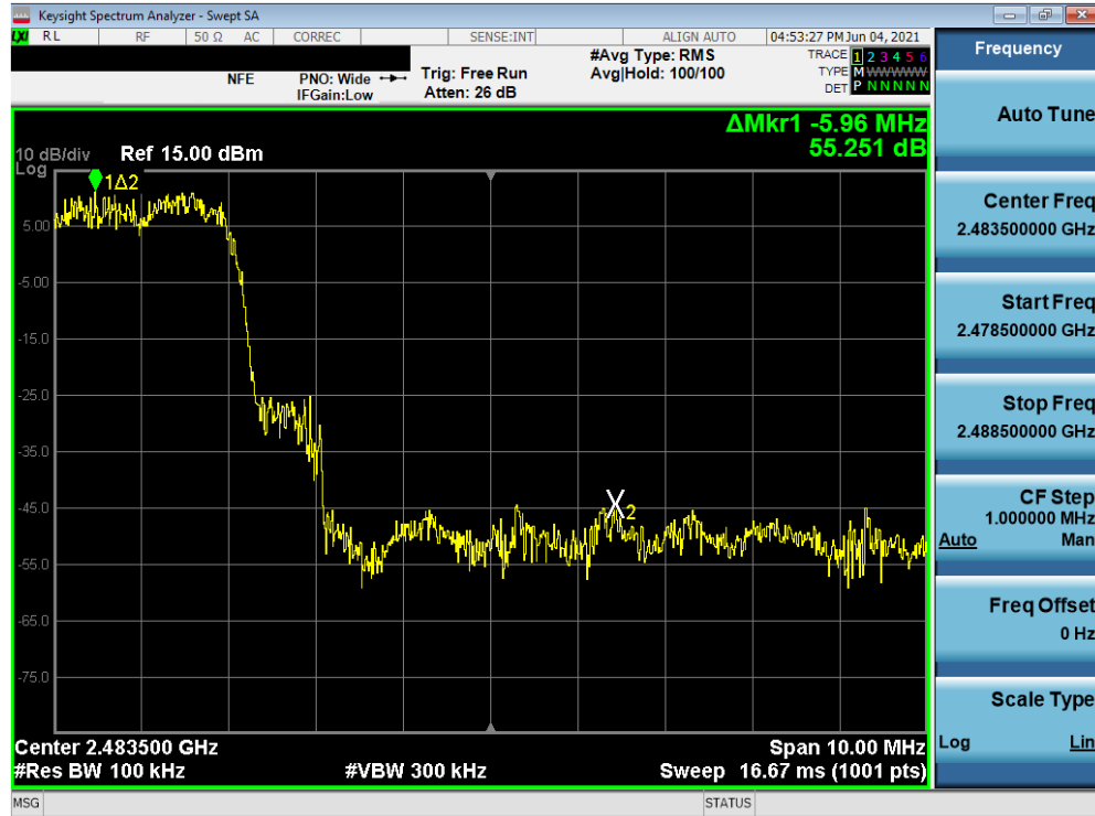
Plot 7-116. Band Edge Plot (Bluetooth with Hopping Enabled, iPA, 3 Mbps – Ch.78) – ANT0
