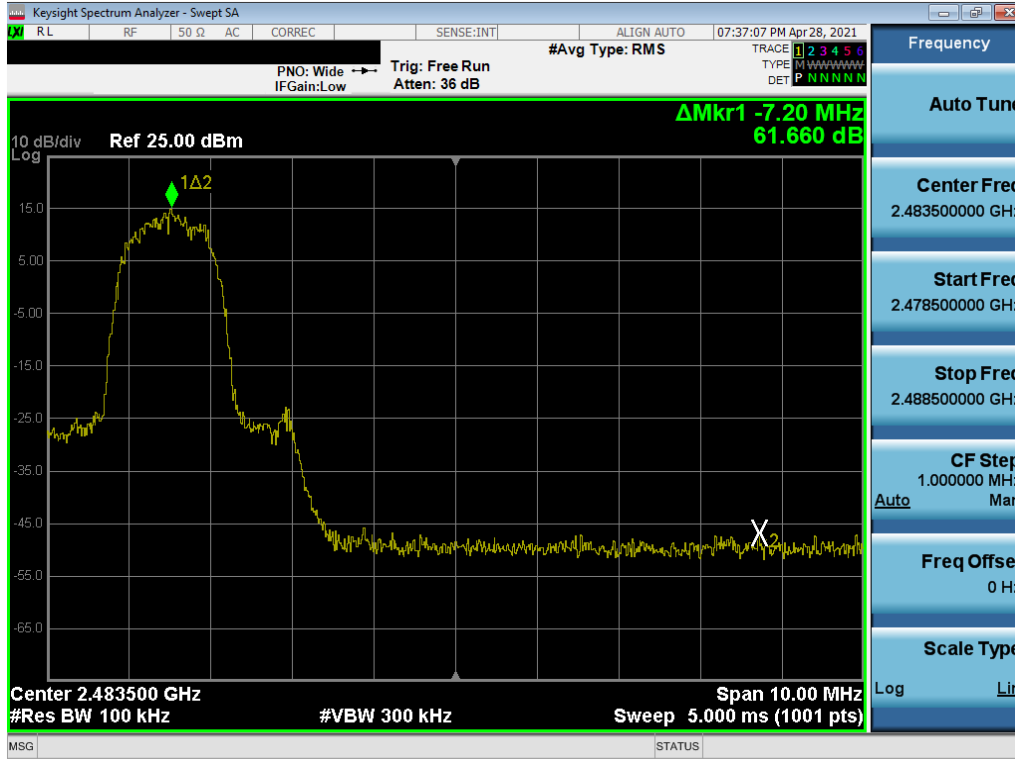
Plot 7-118. Band Edge Plot (Bluetooth with Hopping Disabled, ePA, 3 Mbps – Ch. 78) – ANT1
