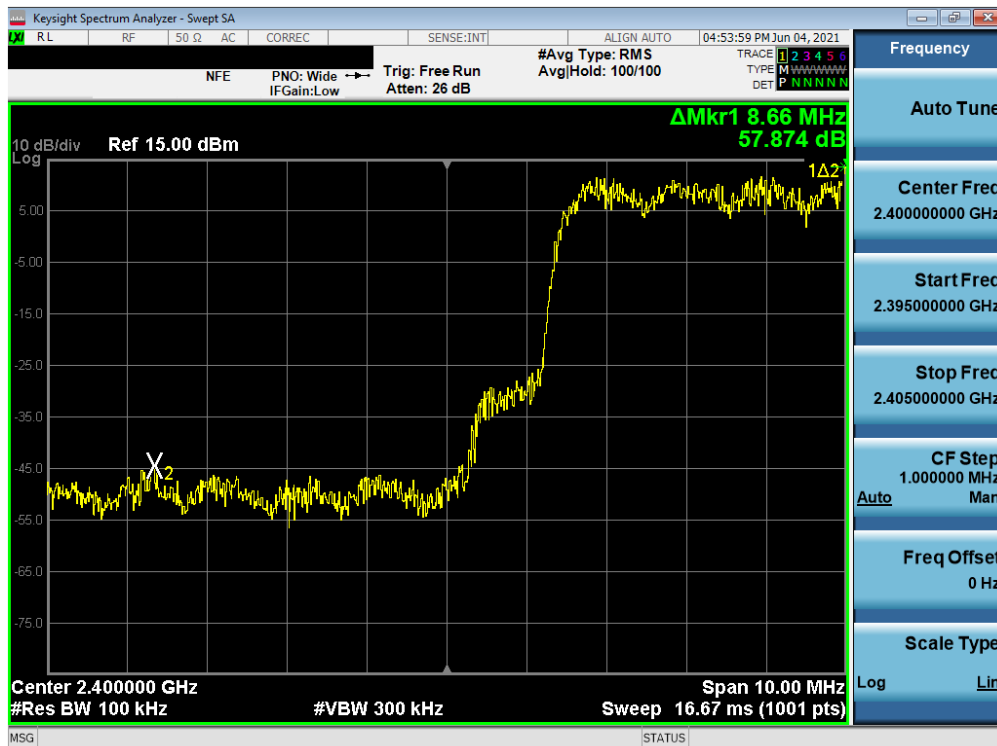
Plot 7-115. Band Edge Plot (Bluetooth with Hopping Enabled, iPA, 3 Mbps – Ch. 0) – ANT0
