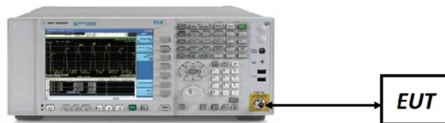
Figure 7-4. Test Instrument & Measurement Setup
