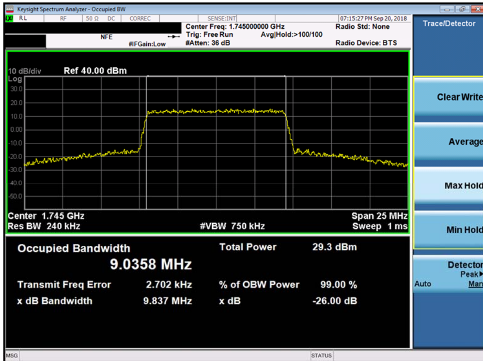
Plot 7-36. Occupied Bandwidth Plot (Band 4 - 10.0MHz 64-QAM - Full RB Configuration)
