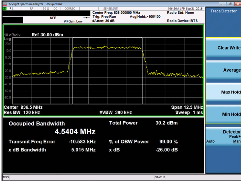
Plot 7-21. Occupied Bandwidth Plot (Band 5 - 5.0MHz 64-QAM - Full RB Configuration)
