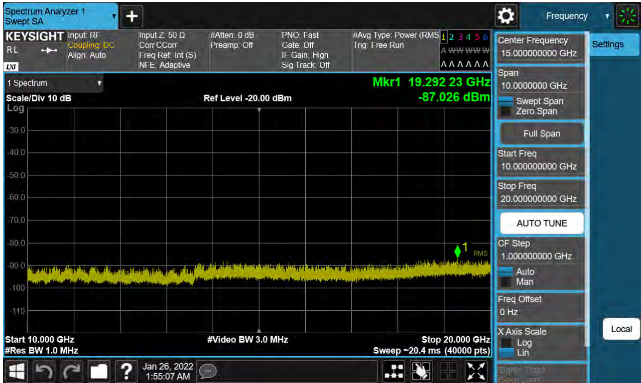
Sub6 n66. Conducted Spurious Plot_2 (349000ch_5 MHz_BPSK_ RB 1_1)
