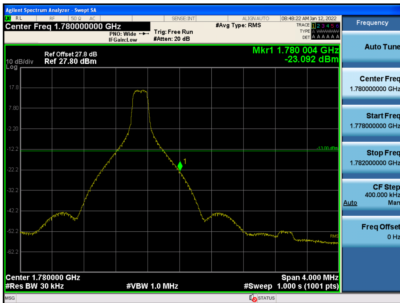
Sub6 n66. Upper Band Edge Plot (15 M BW Ch.354500 BPSK_RB1_Offset 78) -1
