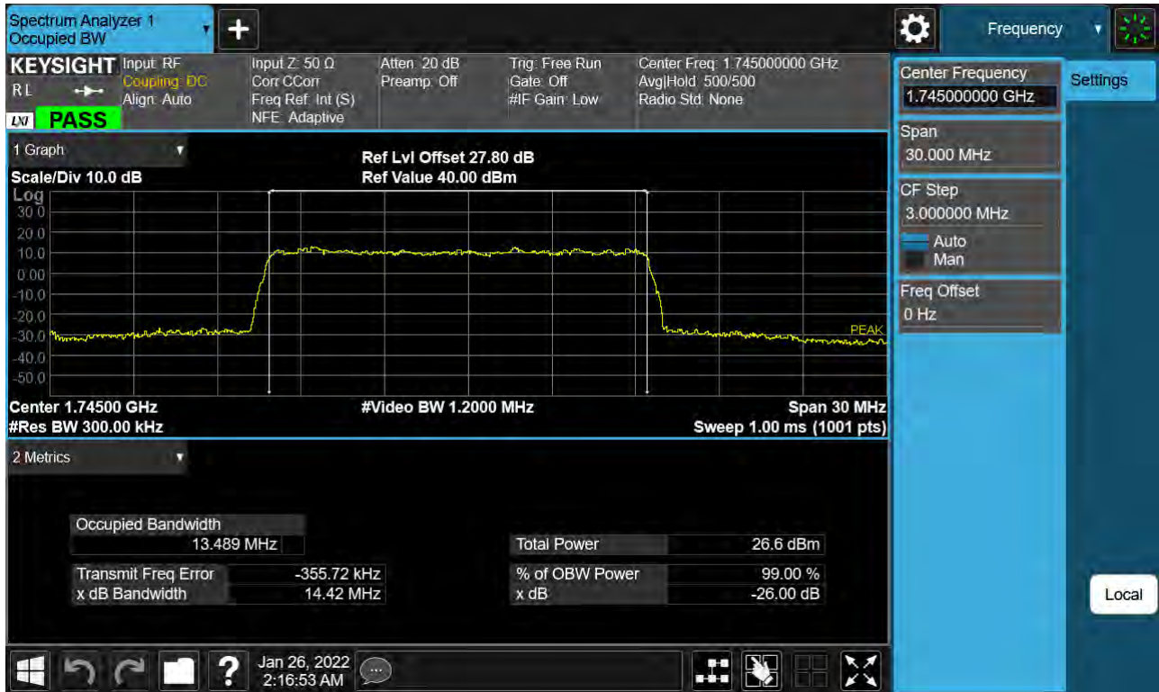
Sub6 n66. Occupied Bandwidth Plot (15 M BW Ch.349000 256QAM Full RB)
