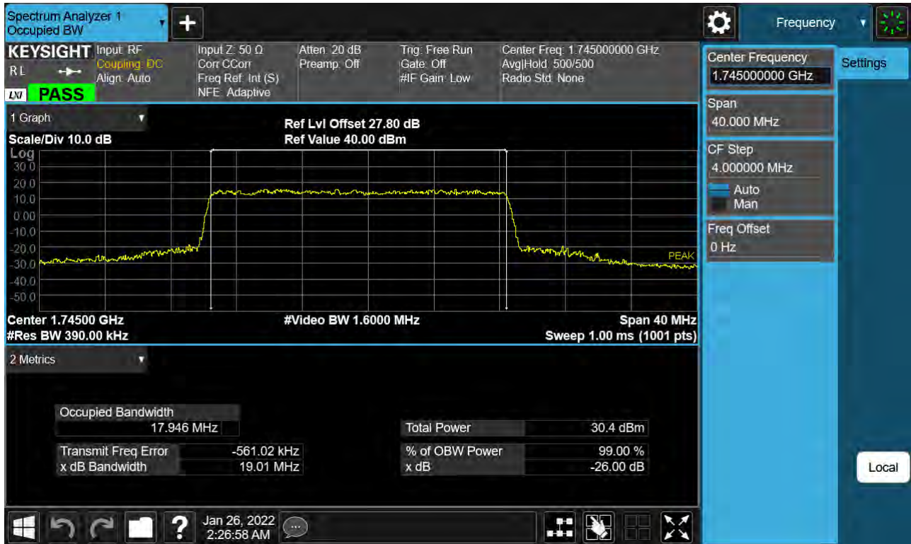
Sub6 n66. Occupied Bandwidth Plot (20 M BW Ch.349000 QPSK Full RB)
