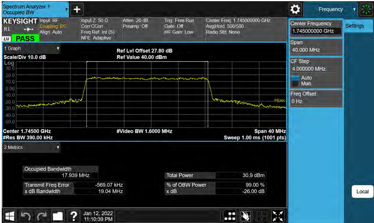
Sub6 n66. Occupied Bandwidth Plot (20 M BW Ch.349000 16QAM Full RB)
