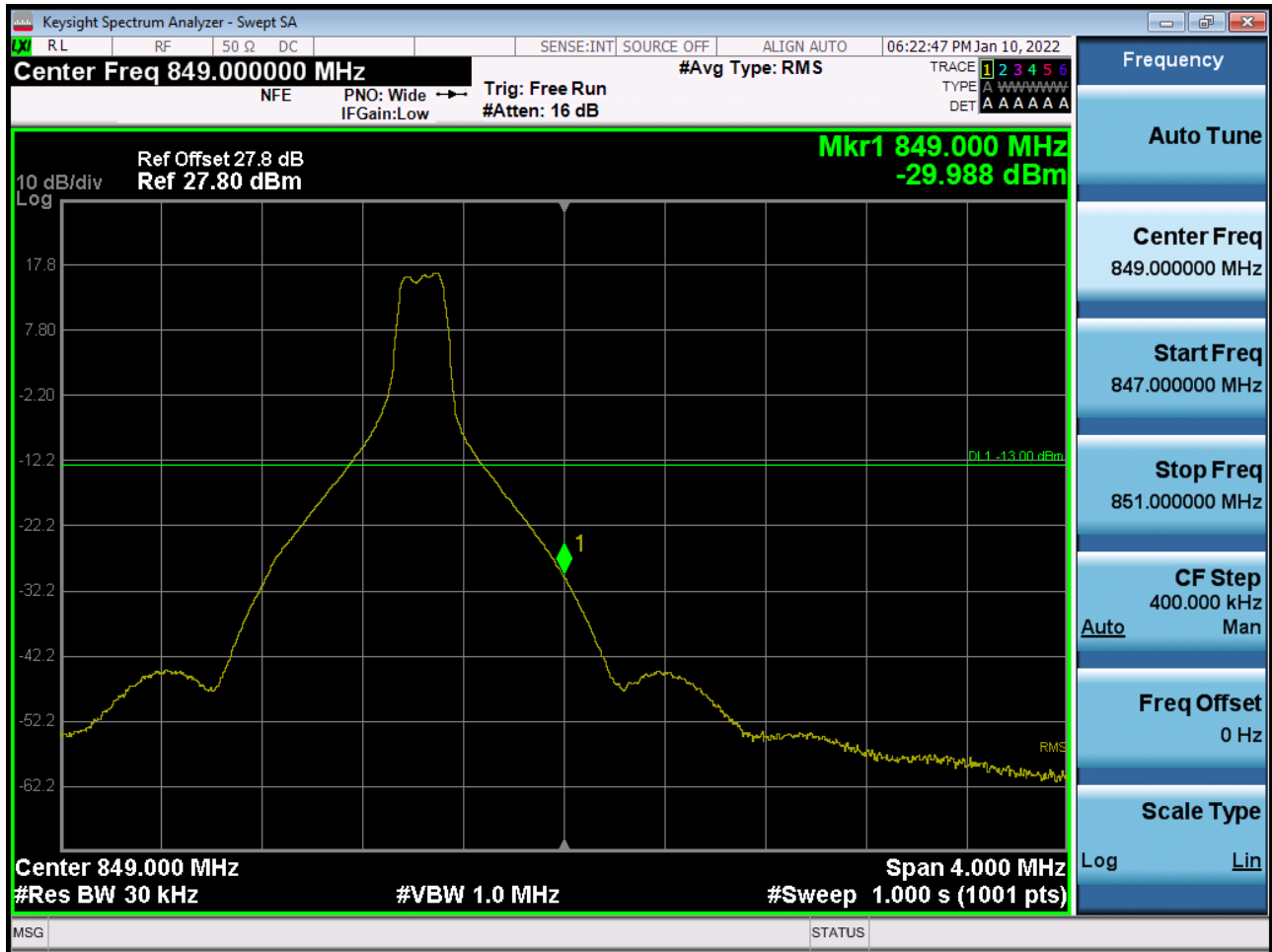
Sub6 n5. Upper Band Edge Plot (20 M BW Ch.167800 BPSK_RB1_Offset 105)
