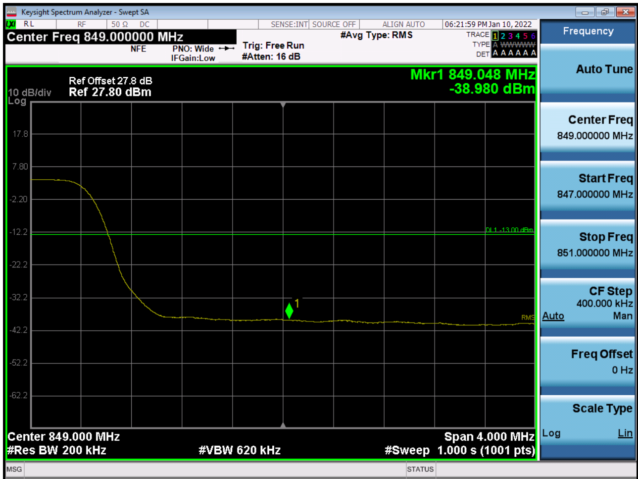
Sub6 n5. Upper Band Edge Plot (20 M BW Ch.167800 BPSK_RB100_Offset 0)
