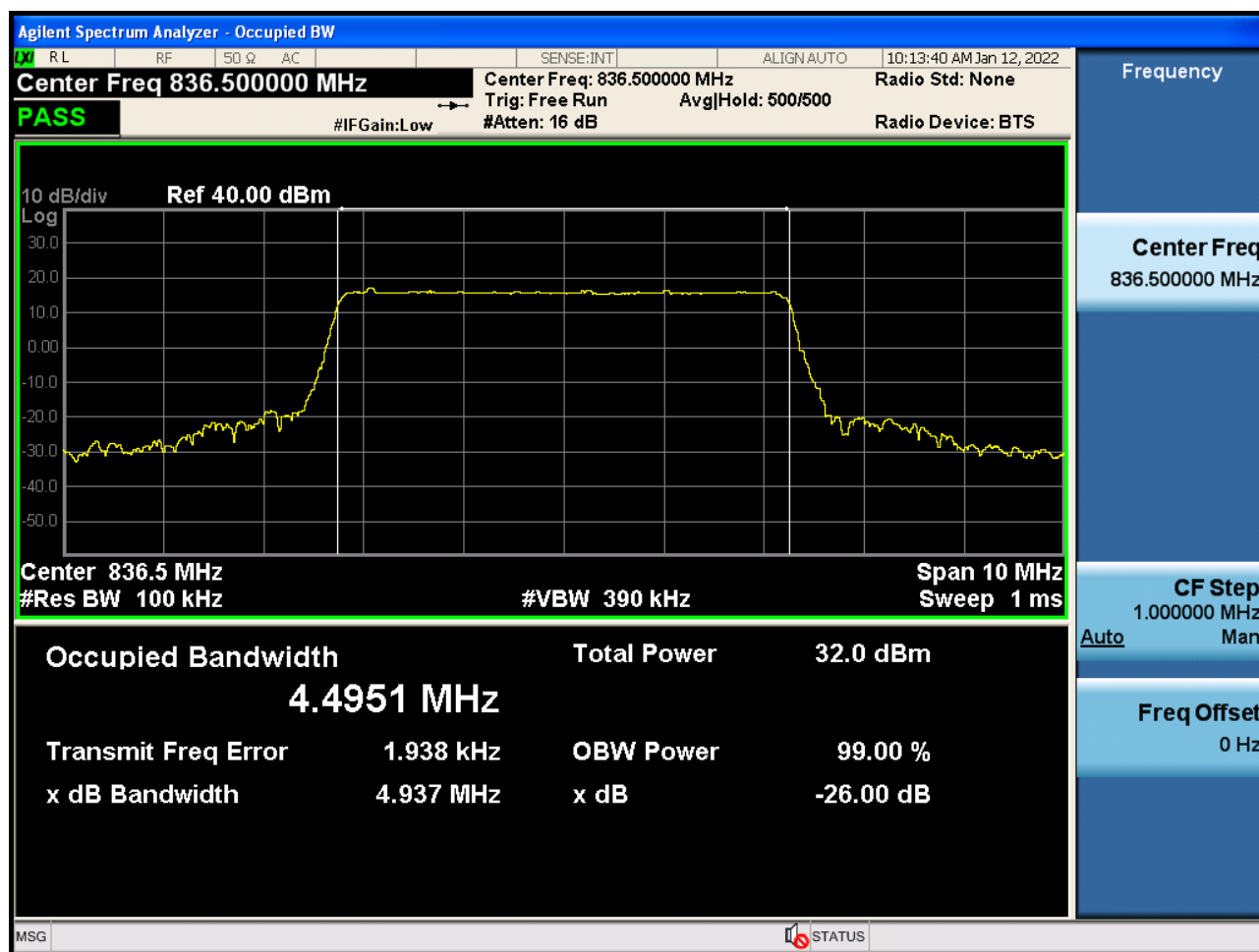
Sub6 n5. Occupied Bandwidth Plot (5 M BW Ch.167300 QPSK_ Full RB _0)
