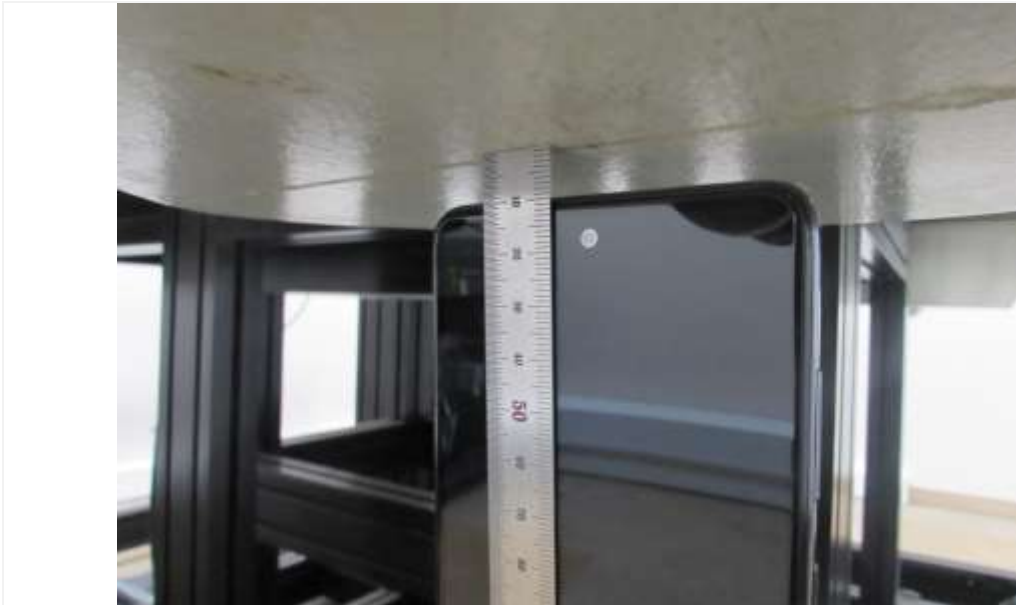
Distance of 10 mm from the EUT
