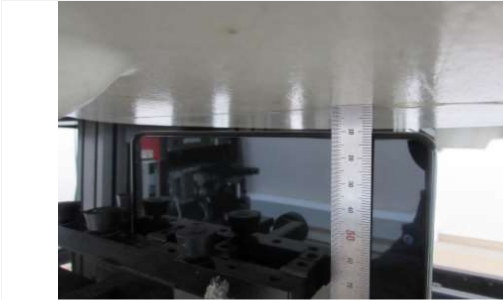
Distance of 10 mm from the EUT
