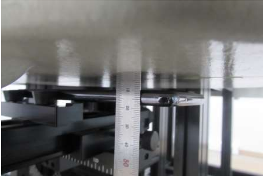
Distance of 10 mm from the EUT
