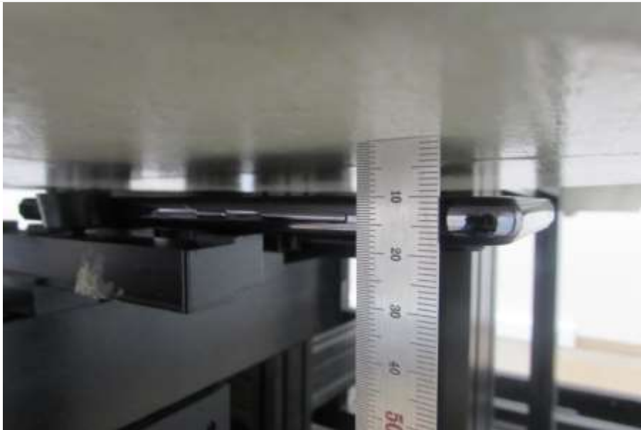
Distance of 10 mm from the EUT
