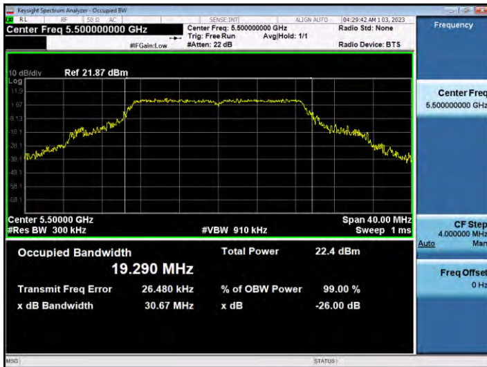
802.11ac_VHT20 UNII 2C BAND 26 dB Bandwidth(CH 100)
