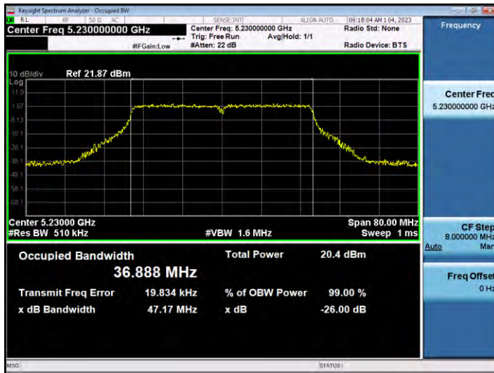
802.11n_HT40 UNII 2C BAND 26 dB Bandwidth(CH 102)
