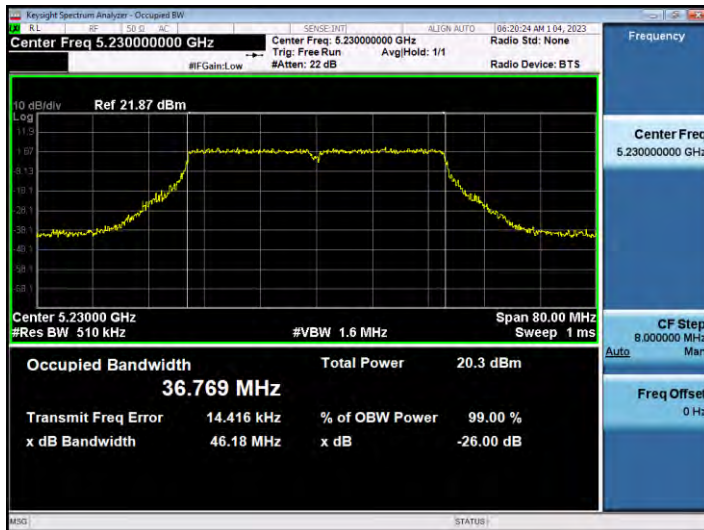
802.11ac_VHT40 UNII 2C BAND 26 dB Bandwidth(CH 102)
