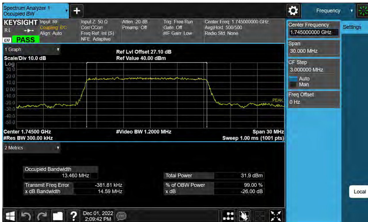
Sub6 n66. Occupied Bandwidth Plot (15 M BW Ch.349000 BPSK Full RB)
