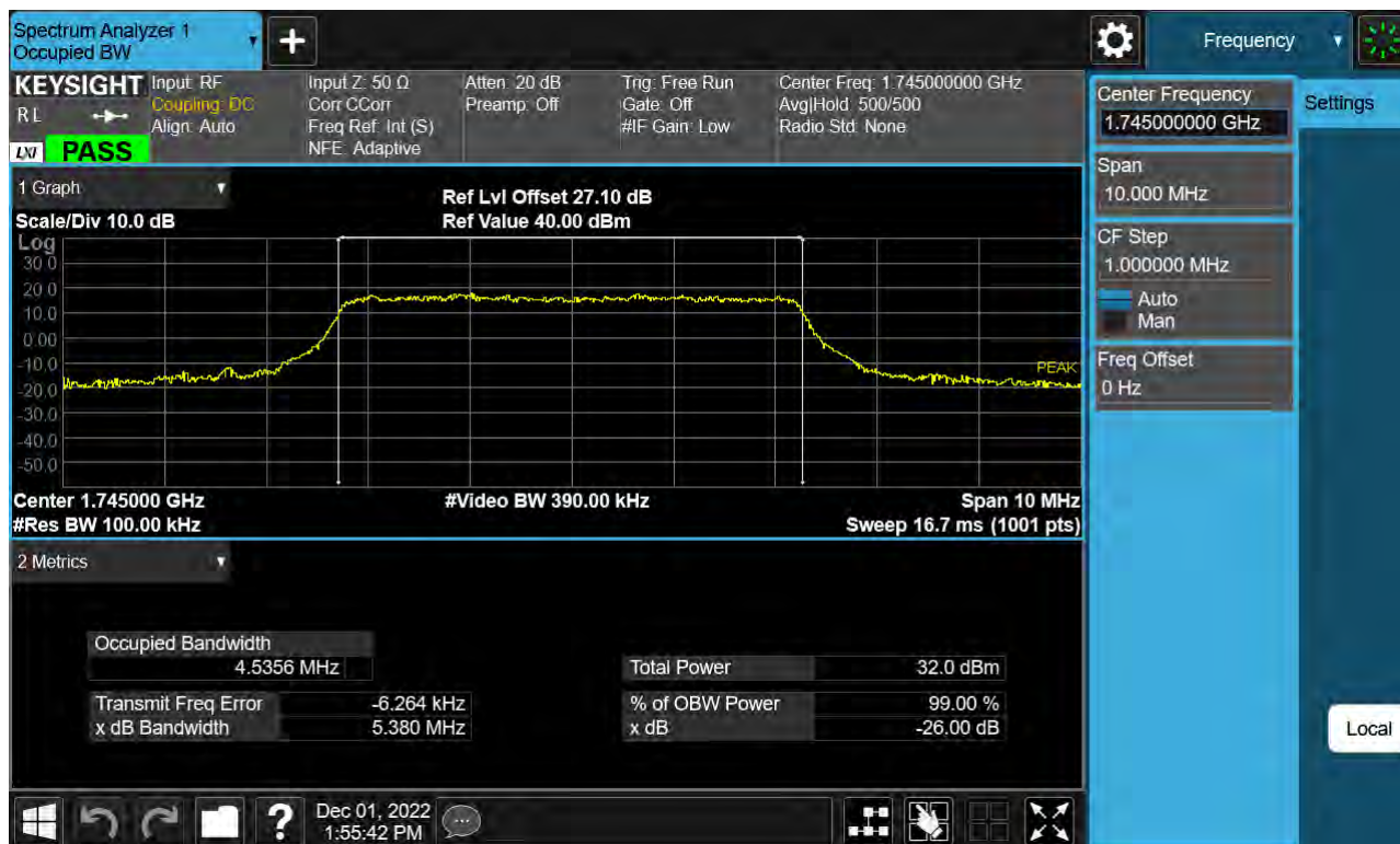
Sub6 n66. Occupied Bandwidth Plot (5 M BW Ch.349000 16QAM Full RB)
