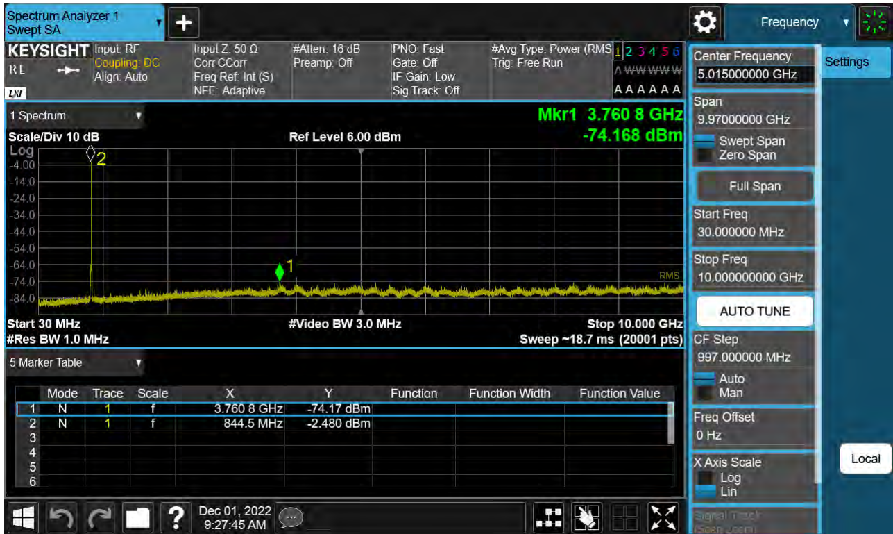
Sub6 n5. Conducted Spurious Plot (169300ch_5 MHz_BPSK_RB 1_1)
