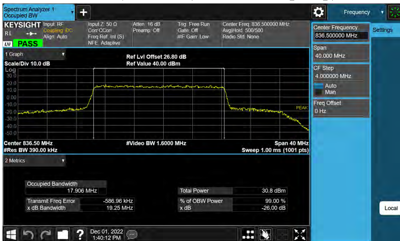
Sub6 n5. Occupied Bandwidth Plot (20 M BW Ch.167300 64QAM_ Full RB _0)
