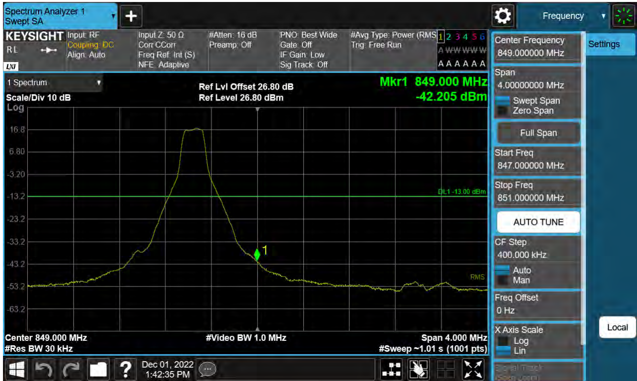
Sub6 n5. Upper Band Edge Plot (20 M BW Ch.167800 BPSK_RB1_Offset 105)
