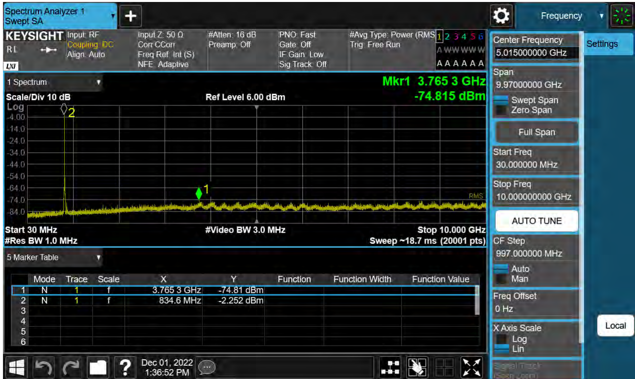
Sub6 n5. Conducted Spurious Plot (168300ch_15 MHz_BPSK_RB 1_1)
