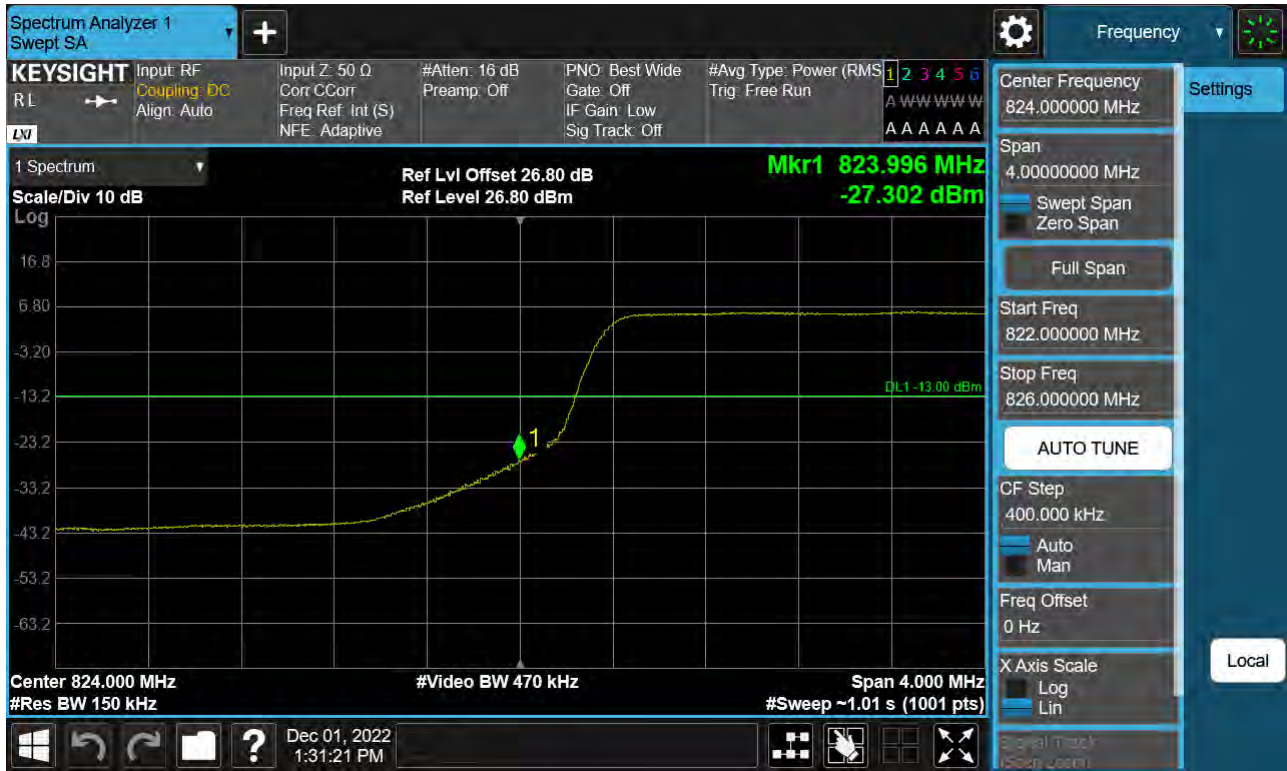
Sub6 n5. Lower Band Edge Plot (15 M BW Ch.166300 BPSK_RB75_Offset 0)
