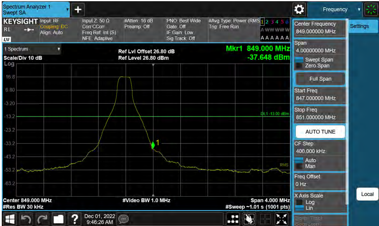
Sub6 n5. Upper Band Edge Plot (10 M BW Ch.168800 BPSK_RB1_Offset 51)
