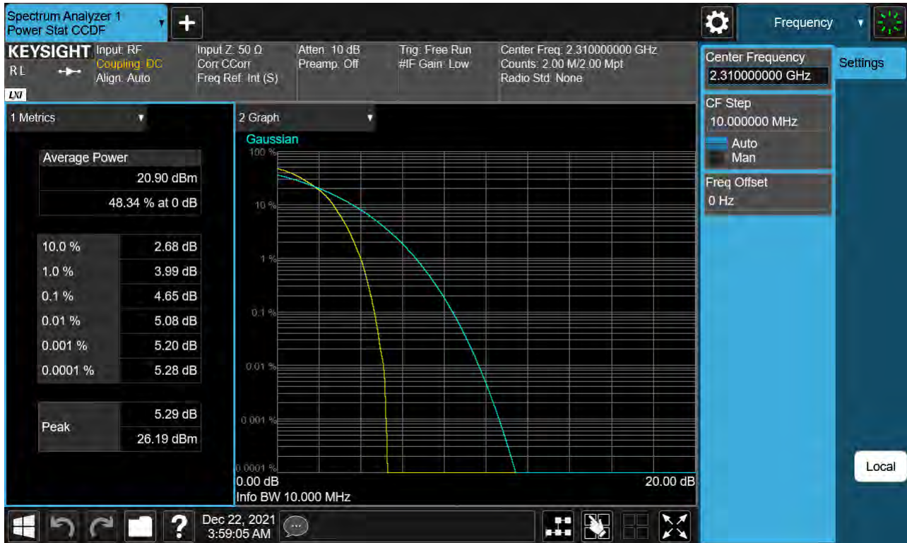
Sub6 n30. PAR Plot (10M BW_Ch.462000_64QAM_RB50_0)
