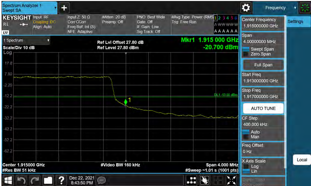
Sub6 n25(2). Upper Band Edge Plot (5 M BW Ch.382500 BPSK_ Full RB) -1
