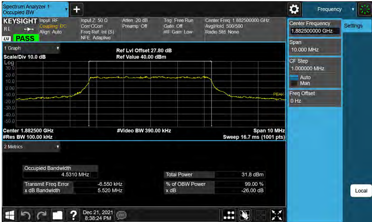
Sub6 n25(2). Occupied Bandwidth Plot (5 M BW Ch.376500 QPSK_ Full RB_0 )
