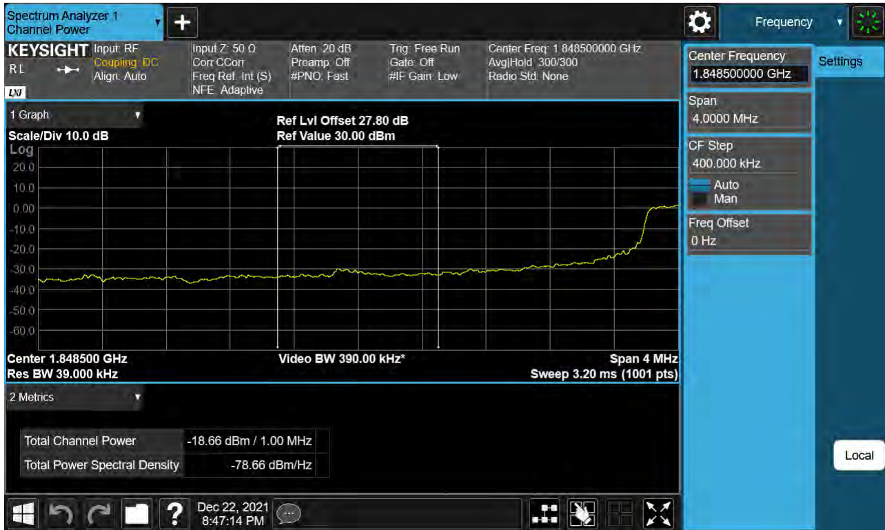
Sub6 n25(2). Lower Extended Band Edge Plot (10 M BW Ch.371000 BPSK_ Full RB) -2
