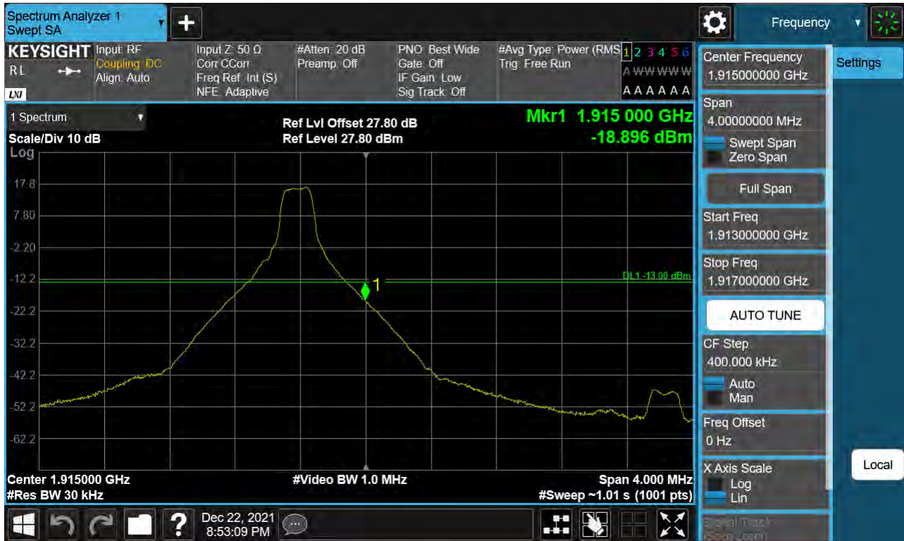
Sub6 n25(2). Upper Band Edge Plot (10 M BW Ch.382000 BPSK_RB1_Offset 51)
