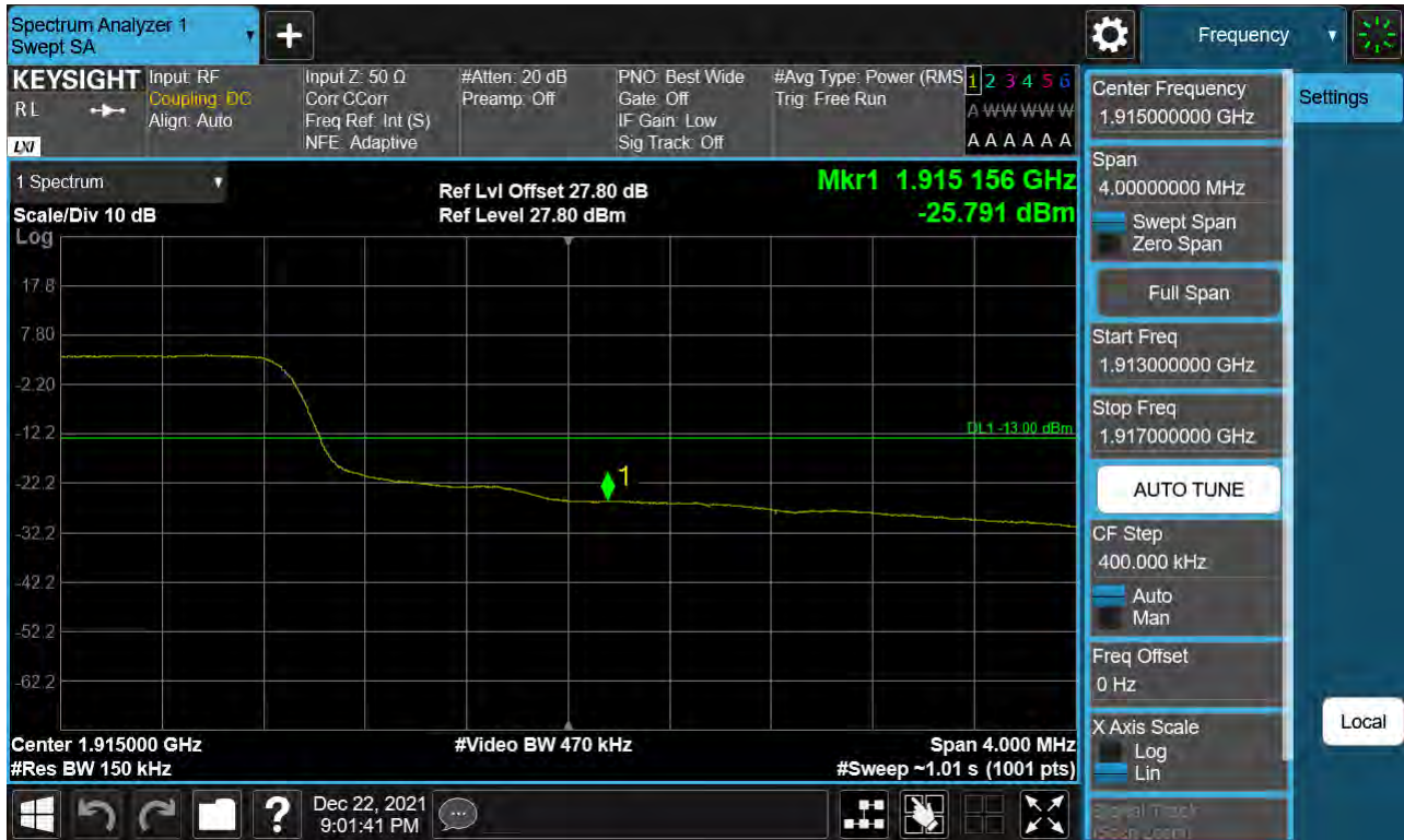
Sub6 n25(2). Upper Band Edge Plot (15 M BW Ch.381500 BPSK_ Full RB) -1
