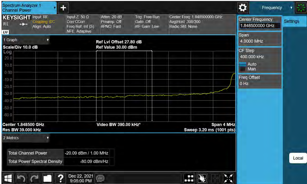
Sub6 n25(2). Lower Extended Band Edge Plot (20 M BW Ch.372000 BPSK_ Full RB) -2
