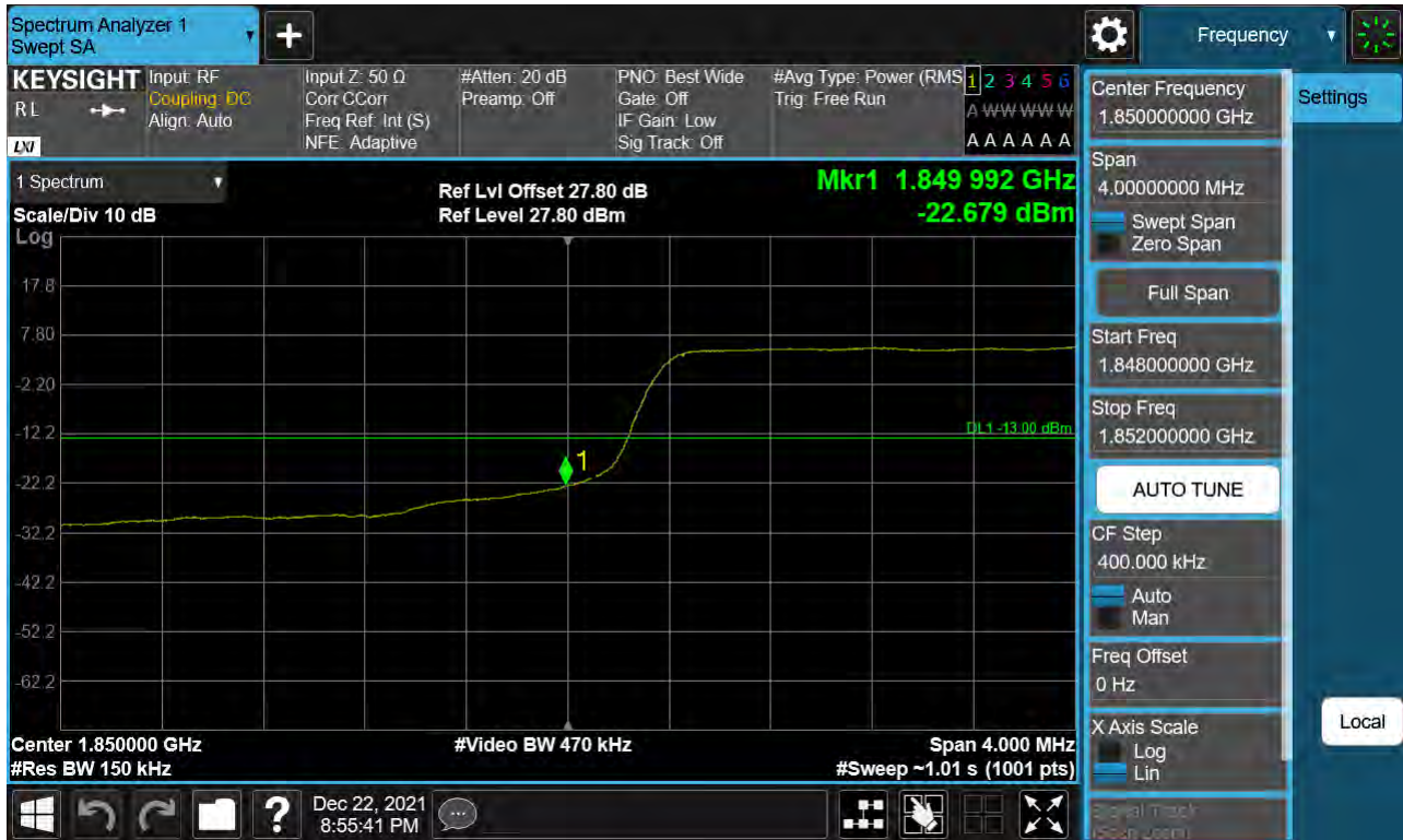
Sub6 n25(2). Lower Band Edge Plot (15 M BW Ch.371500 BPSK_ Full RB) -1
