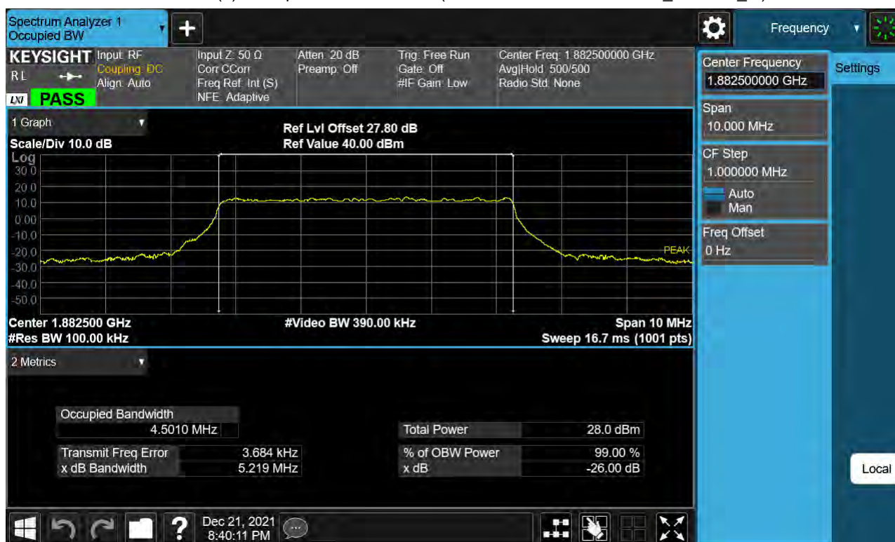
Sub6 n25(2). Occupied Bandwidth Plot (5 M BW Ch.376500 256QAM_ Full RB _0 )
