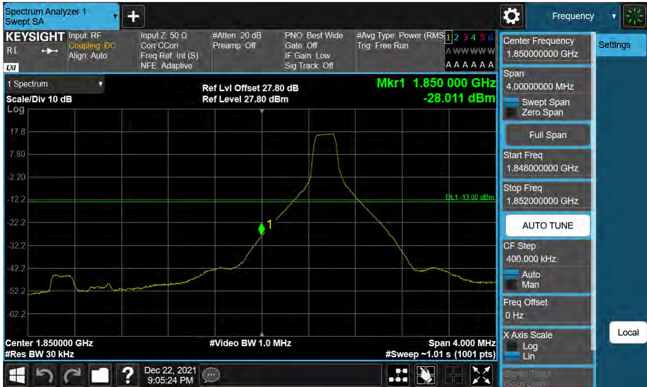
Sub6 n25(2). Lower Band Edge Plot (20 M BW Ch.372000 BPSK_RB1_Offset 0)
