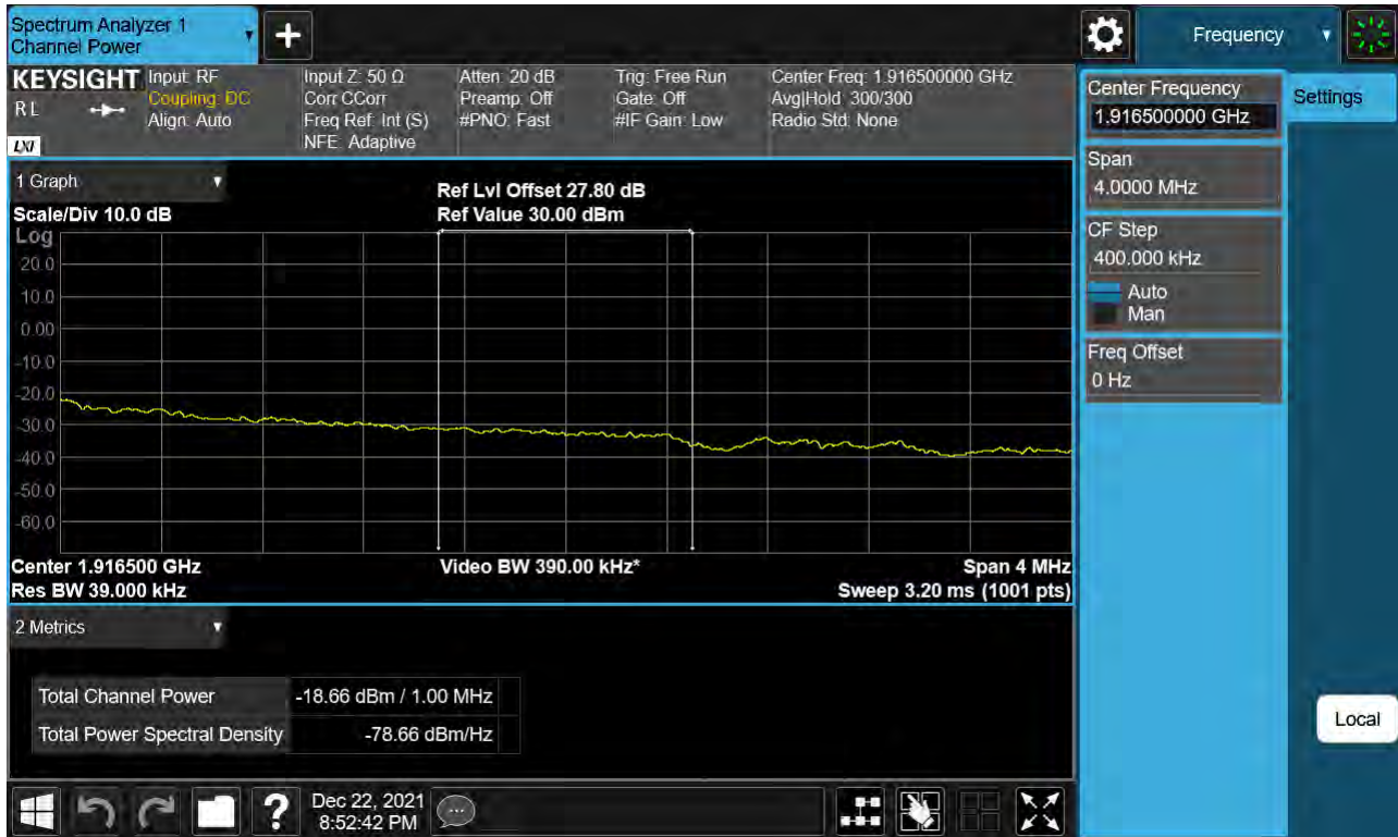
Sub6 n25(2). Upper Extended Band Edge Plot (10 M BW Ch.382000 BPSK_ Full RB) -2
