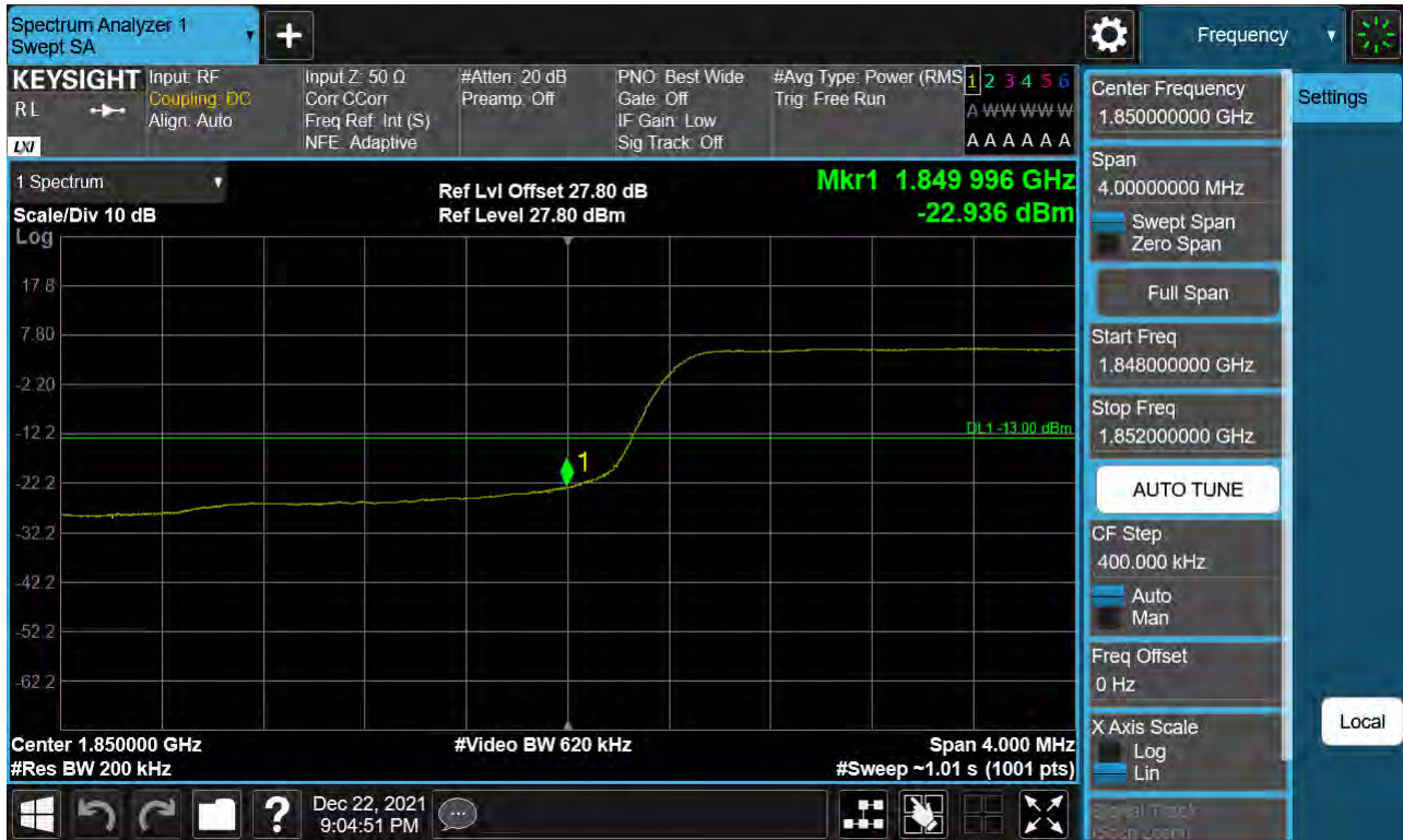
Sub6 n25(2). Lower Band Edge Plot (20 M BW Ch.372000 BPSK_ Full RB) -1
