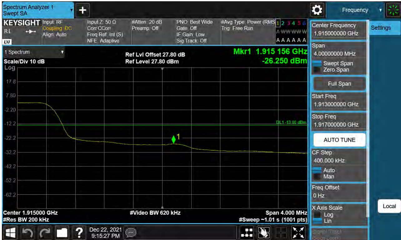
Sub6 n25(2). Upper Band Edge Plot (20 M BW Ch.381000 BPSK_ Full RB) -1
