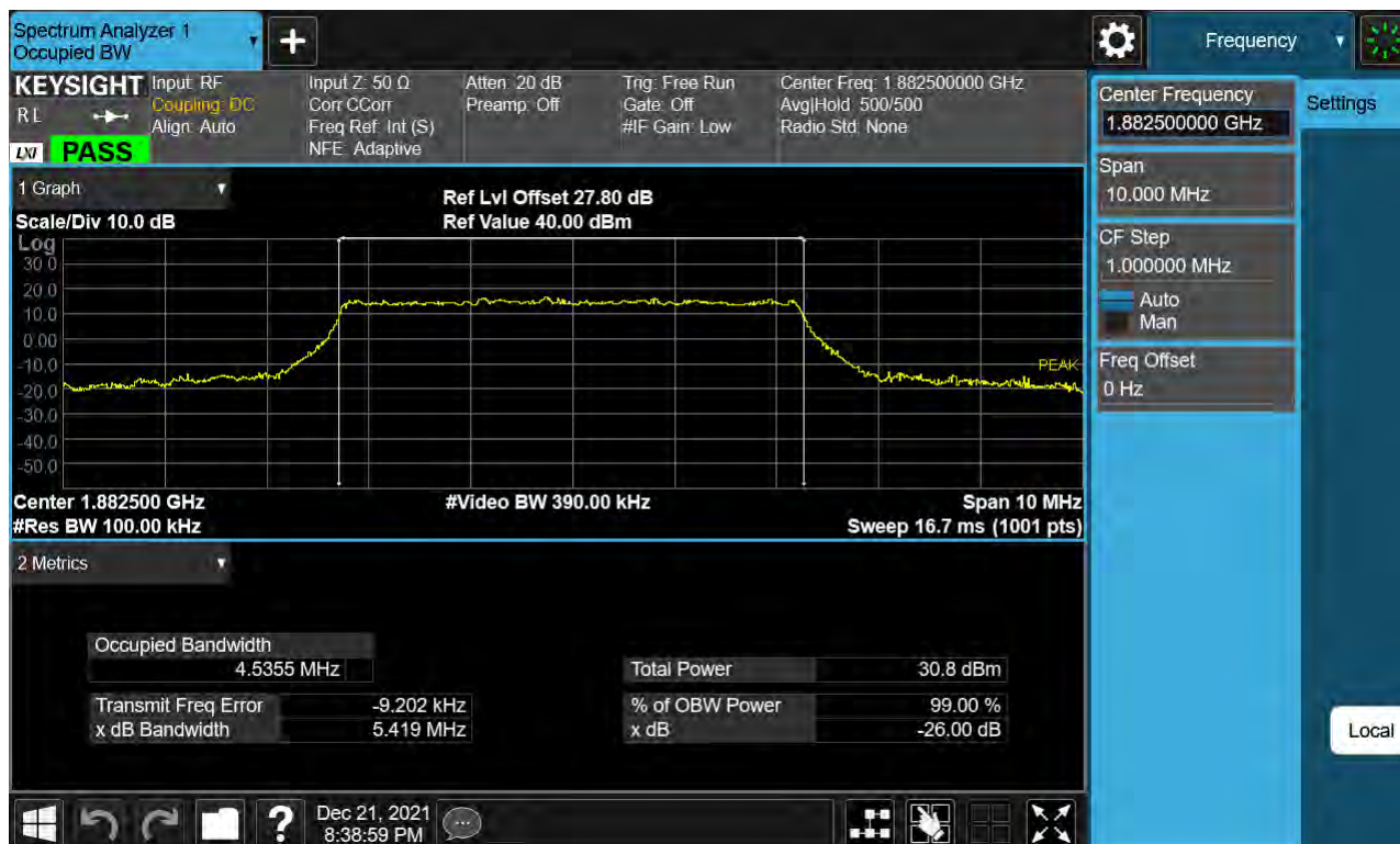
Sub6 n25(2). Occupied Bandwidth Plot (5 M BW Ch.376500 16QAM _ Full RB _0)
