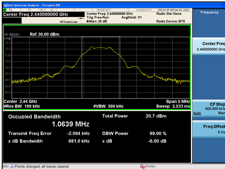
6 dB Bandwidth plot (Mid-CH 19)
