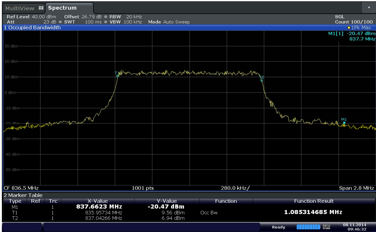
Plot 6-1. Occupied Bandwidth Plot (Band 5 – 1.4MHz QPSK - RB Size 6)
