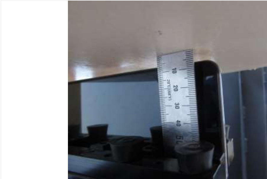
Distance of 7 mm from the EUT
