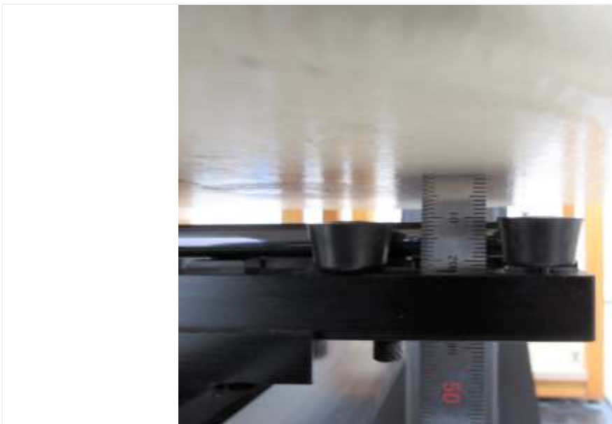
Distance of 11 mm from the EUT
