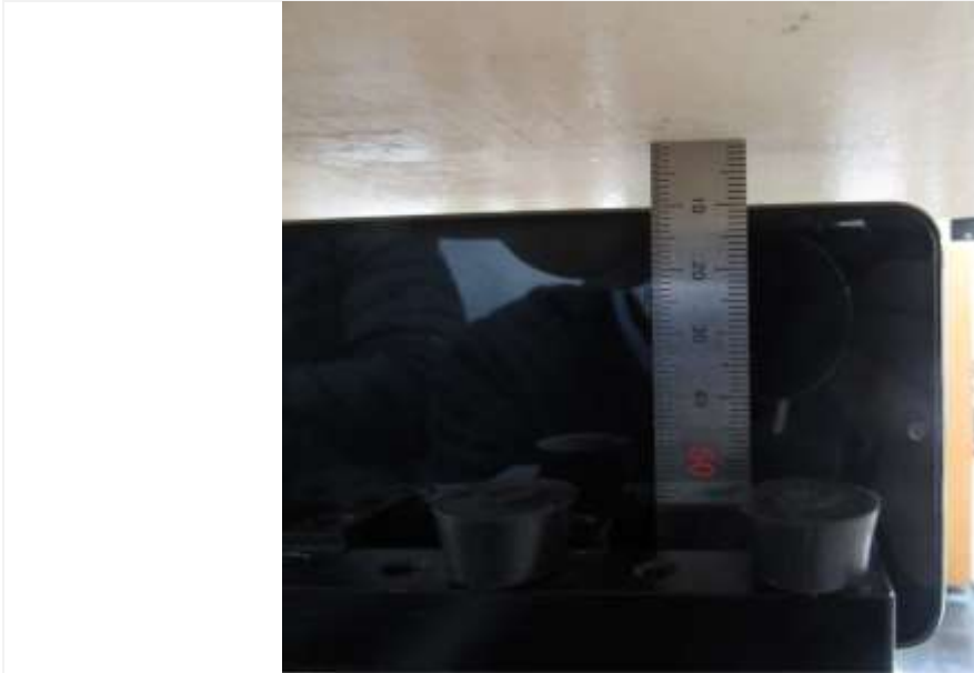
Distance of 10 mm from the EUT
