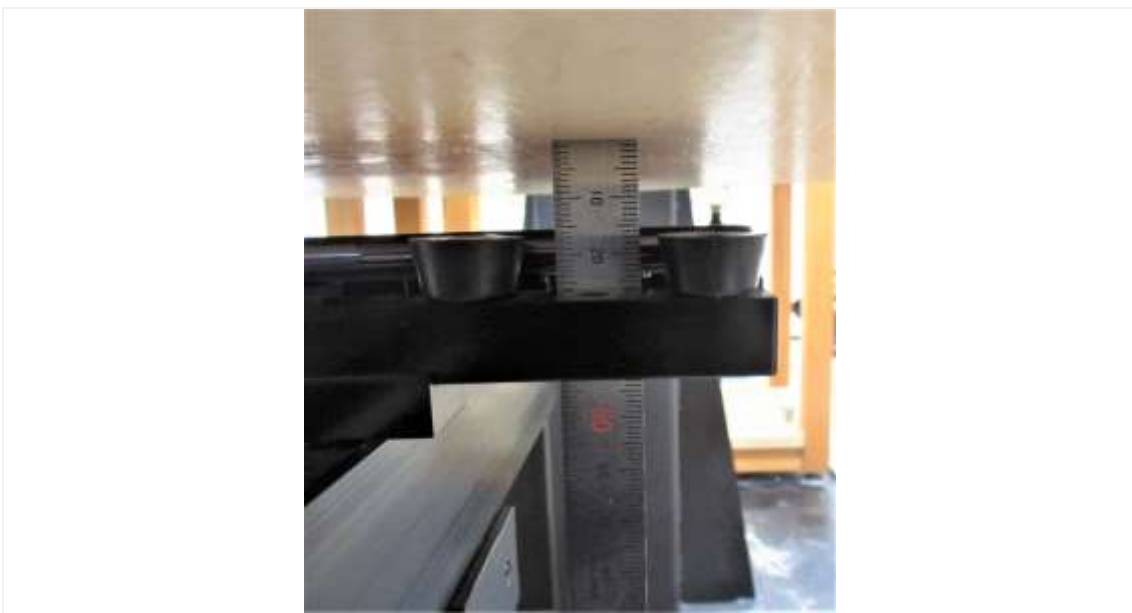
Distance of 15 mm from the EUT
