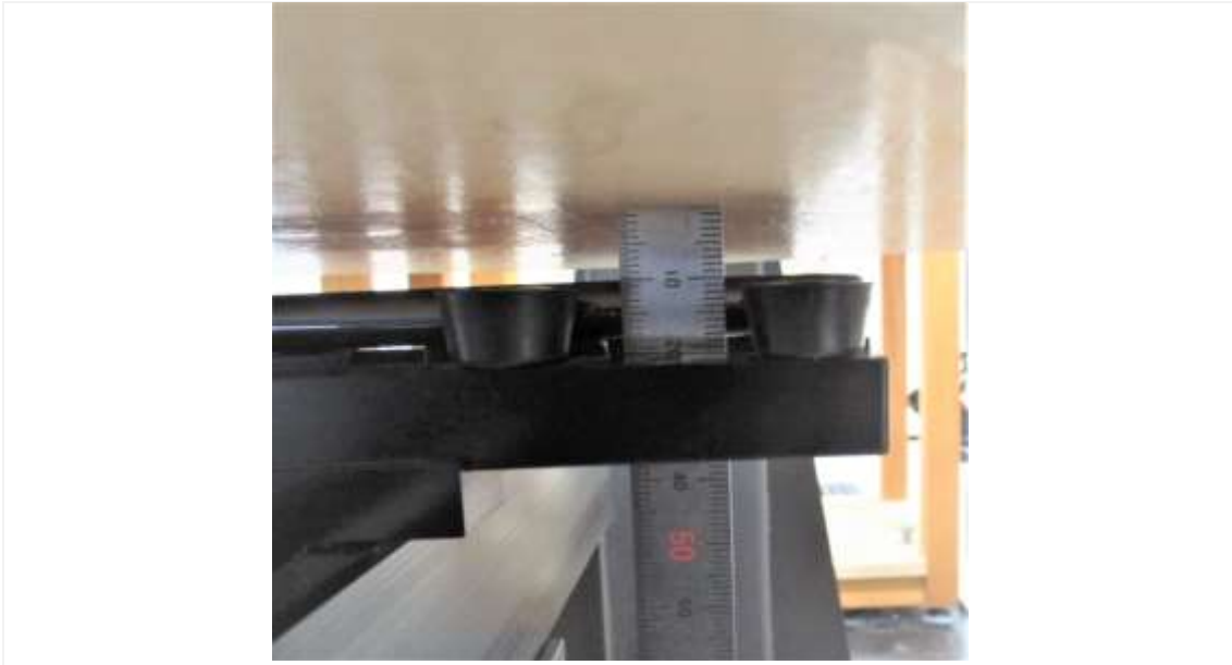
Distance of 10 mm from the EUT
