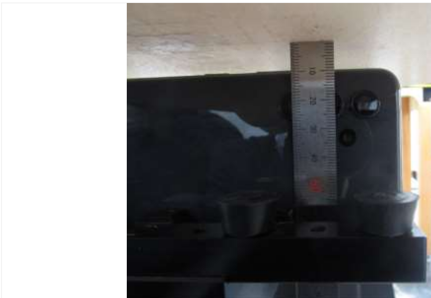
Distance of 10 mm from the EUT
