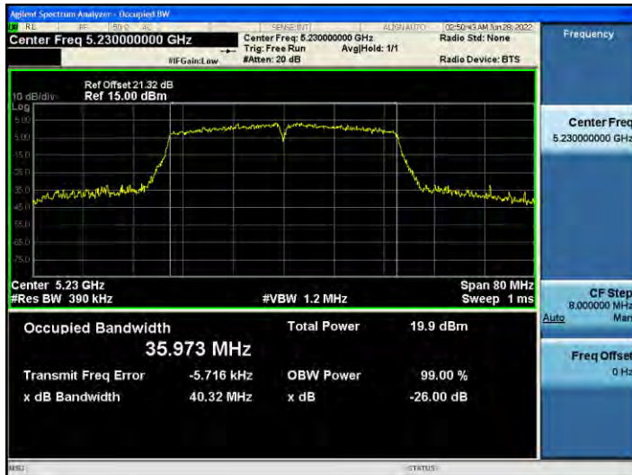
802.11ac_VHT40 UNII 2C BAND 26 dB Bandwidth(CH 118)
