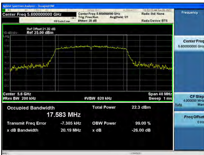
802.11ac_VHT20 UNII 2C BAND 26 dB Bandwidth(CH 120)
