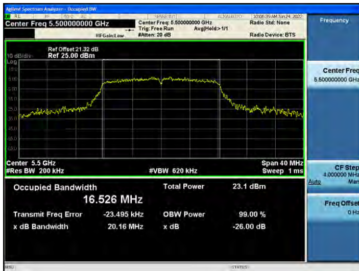
802.11a UNII 2C BAND 26 dB Bandwidth (CH 100)
