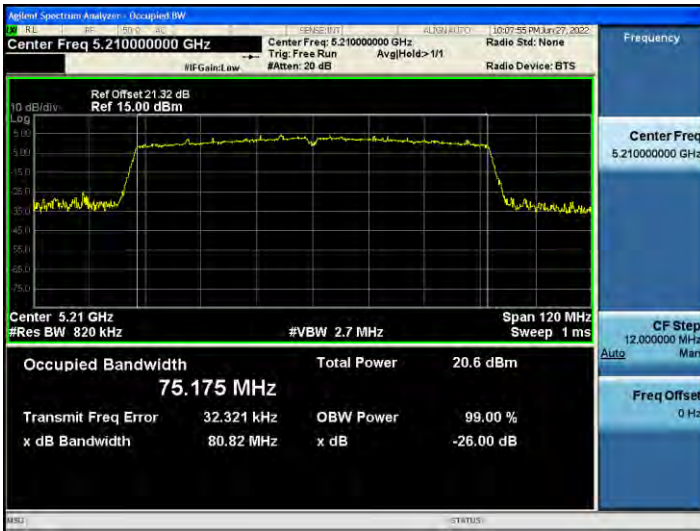
802.11ac_VHT80 UNII 2C BAND 26 dB Bandwidth(CH 122)
