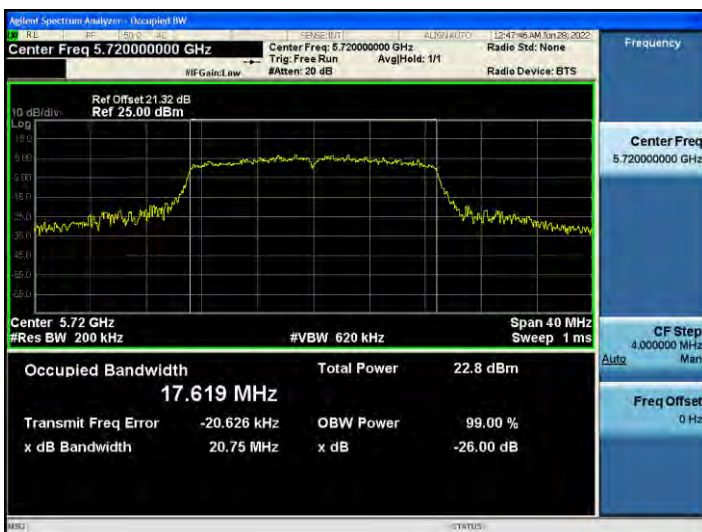
802.11n_HT20 UNII 2C BAND 26 dB Bandwidth(CH 144)
