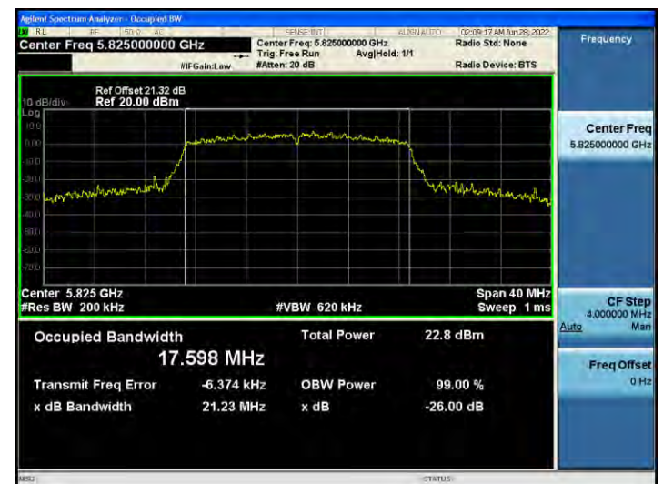
802.11ac_VHT20 UNII 3 BAND 26 dB Bandwidth(CH 165)
