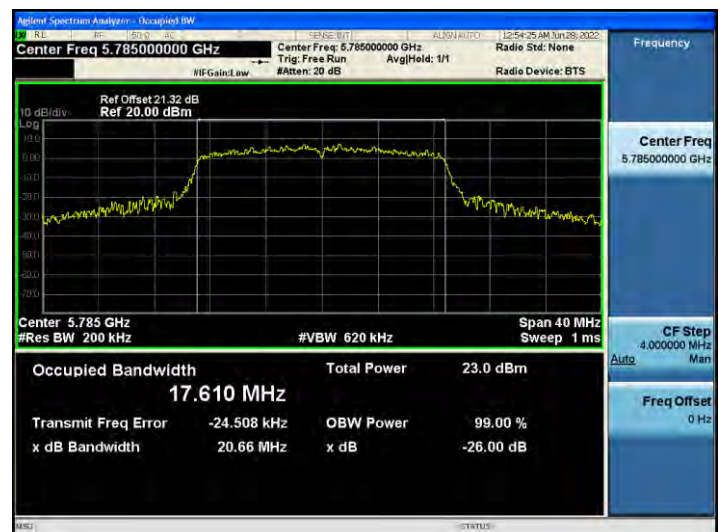
802.11n_HT20 UNII 3 BAND 26 dB Bandwidth(CH 157)
