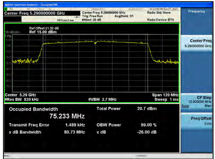
802.11ac_VHT80 UNII 3 BAND 26 dB Bandwidth (CH 155)
