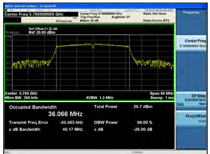
802.11n_HT40 UNII 3 BAND 26 dB Bandwidth (CH 159)
