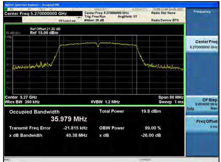
802.11ac_VHT40 UNII 3 BAND 26 dB Bandwidth (CH 159)
