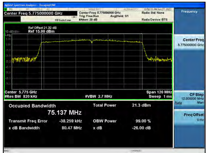
802.11ac_VHT80 UNII 3 BAND 26 dB Bandwidth (CH 155)
