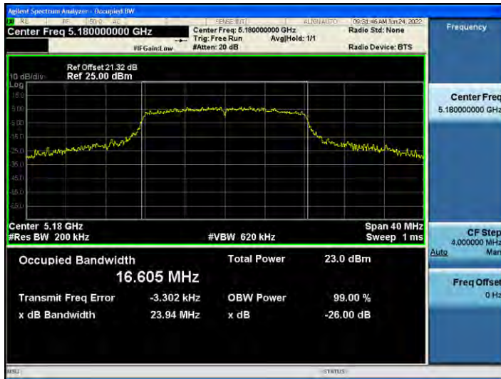
802.11a UNII 2C BAND 26 dB Bandwidth (CH 100)
