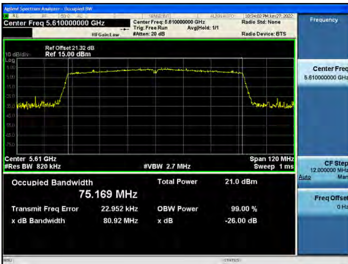
802.11ac_VHT80 UNII 2C BAND 26 dB Bandwidth(CH 122)
