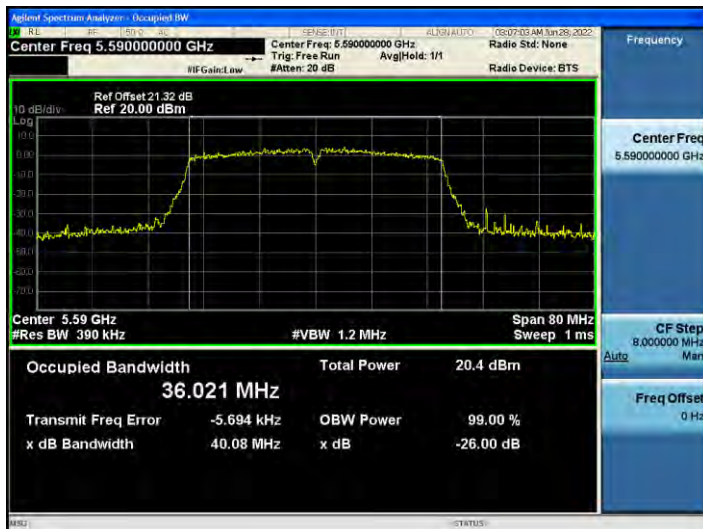
802.11ac_VHT40 UNII 2C BAND 26 dB Bandwidth(CH 118)
