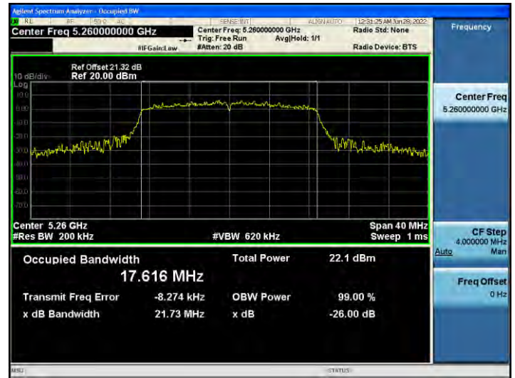
802.11n_HT20 UNII 3 BAND 26 dB Bandwidth(CH 157)
