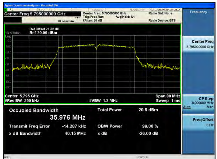
802.11ac_VHT40 UNII 3 BAND 26 dB Bandwidth (CH 159)
