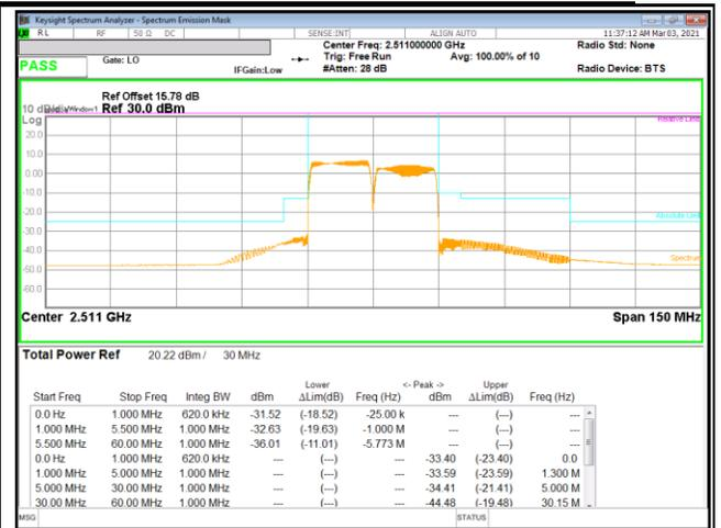
LTE B41 15MHz + 15MHz 16QAM Low Ch RB75-0 + RB75-0
