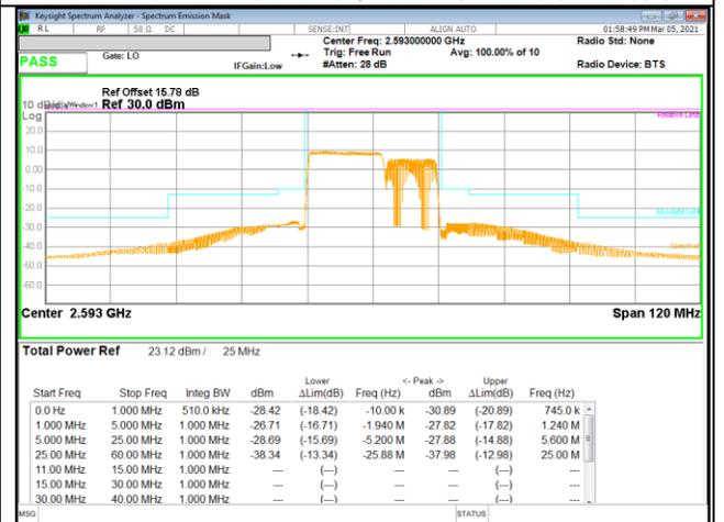
LTE B41 15MHz + 10MHz 16QAM Mid Ch RB75-0 + RB50-0
