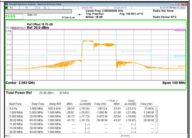
LTE B41 10MHz + 20MHz 16QAM Mid Ch RB50-0 + RB100-0
