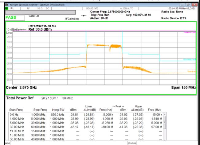
LTE B41 20MHz + 10MHz 16QAM High Ch RB100-0 + RB50-0
