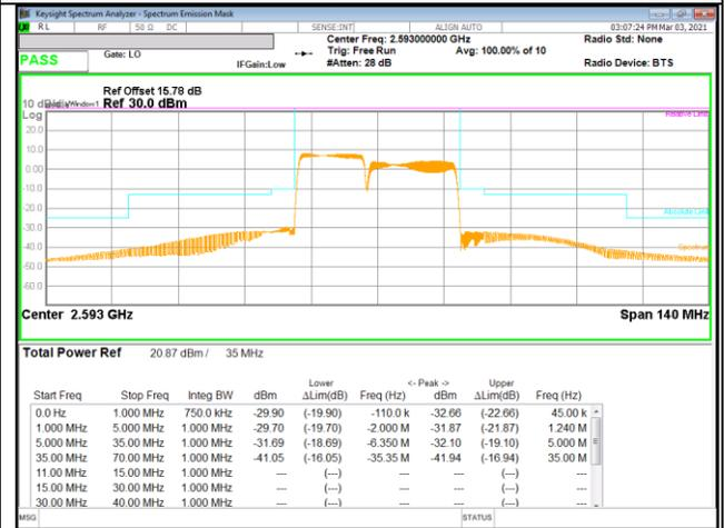
LTE B41 15MHz + 20MHz QPSK Mid Ch RB75-0 + RB100-0
