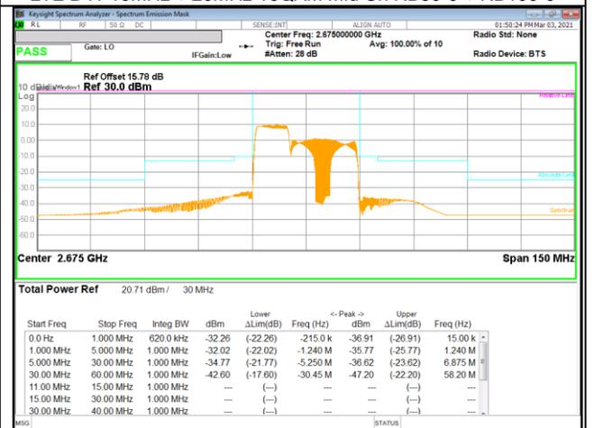
LTE B41 10MHz + 20MHz 16QAM High Ch RB50-0 + RB100-0
