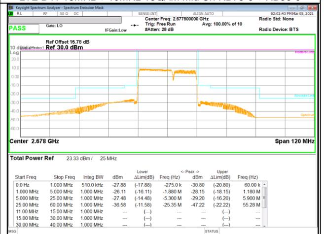
LTE B41 15MHz + 10MHz 16QAM High Ch RB75-0 + RB50-0
