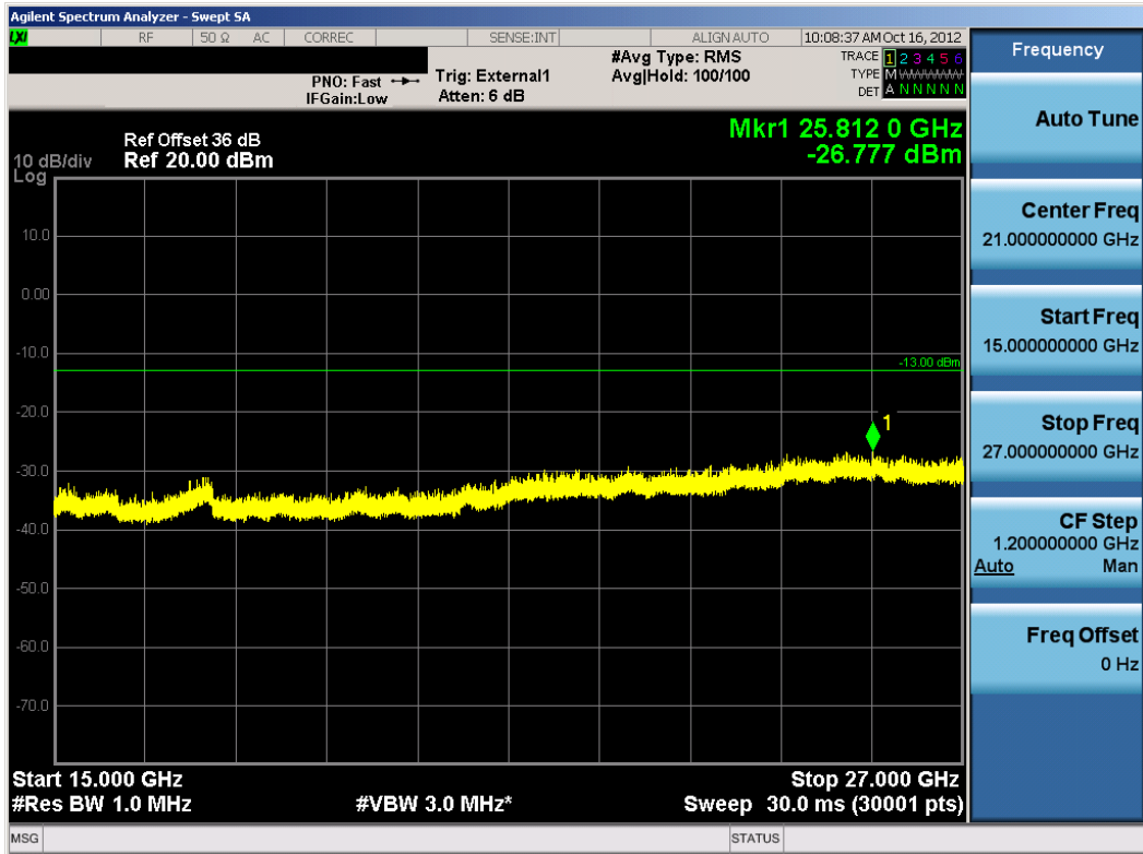
Plot 8-146. Conducted Spurious Plot (TD-LTE Mode – Low Channel)
