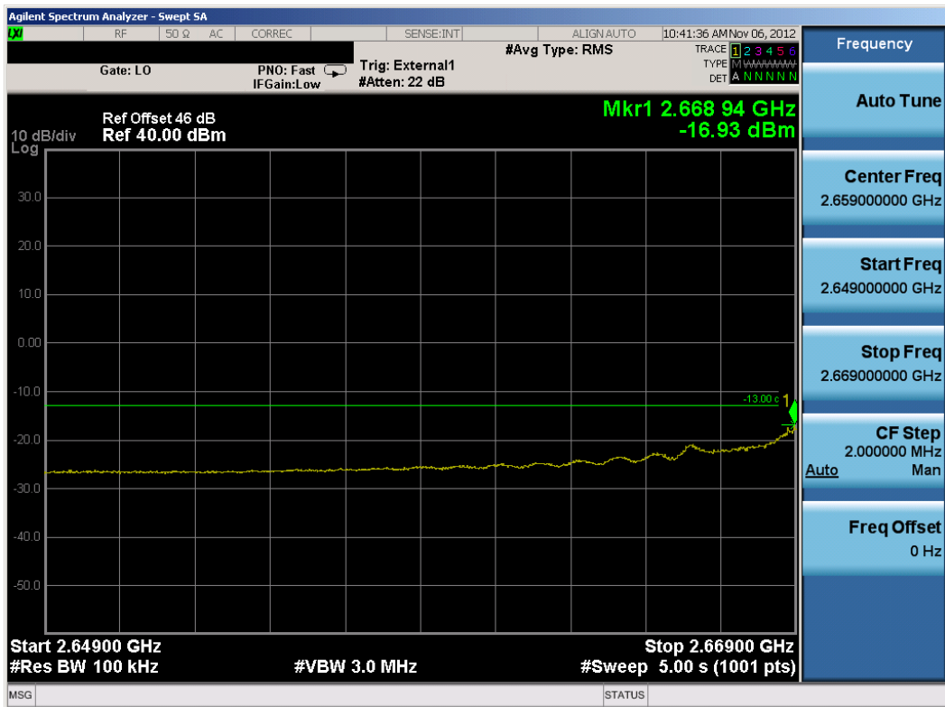
Plot 8-111. Lower Extended Channel Edge Plot (TD-LTE Mode – High Channel)
