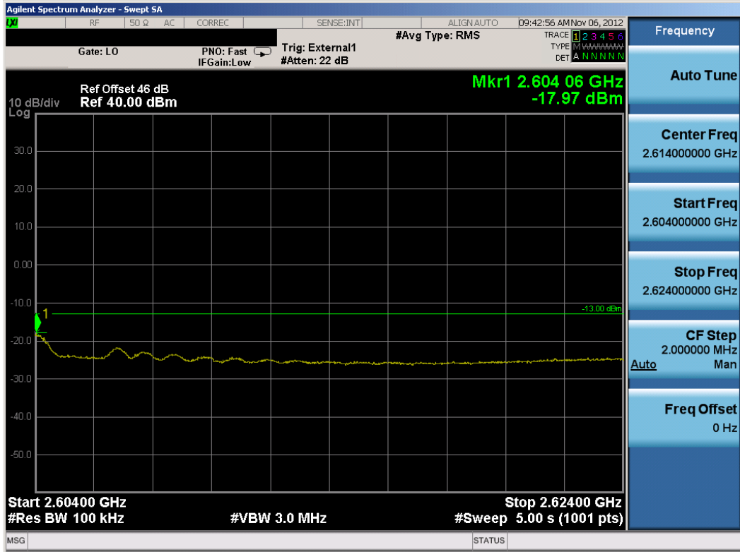
Plot 8-154. Upper Extended Channel Edge Plot (TD-LTE Mode – Mid Channel)
