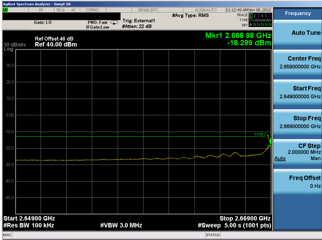
Plot 8-31. Lower Extended Channel Edge Plot (TD-LTE Mode – High Channel)
