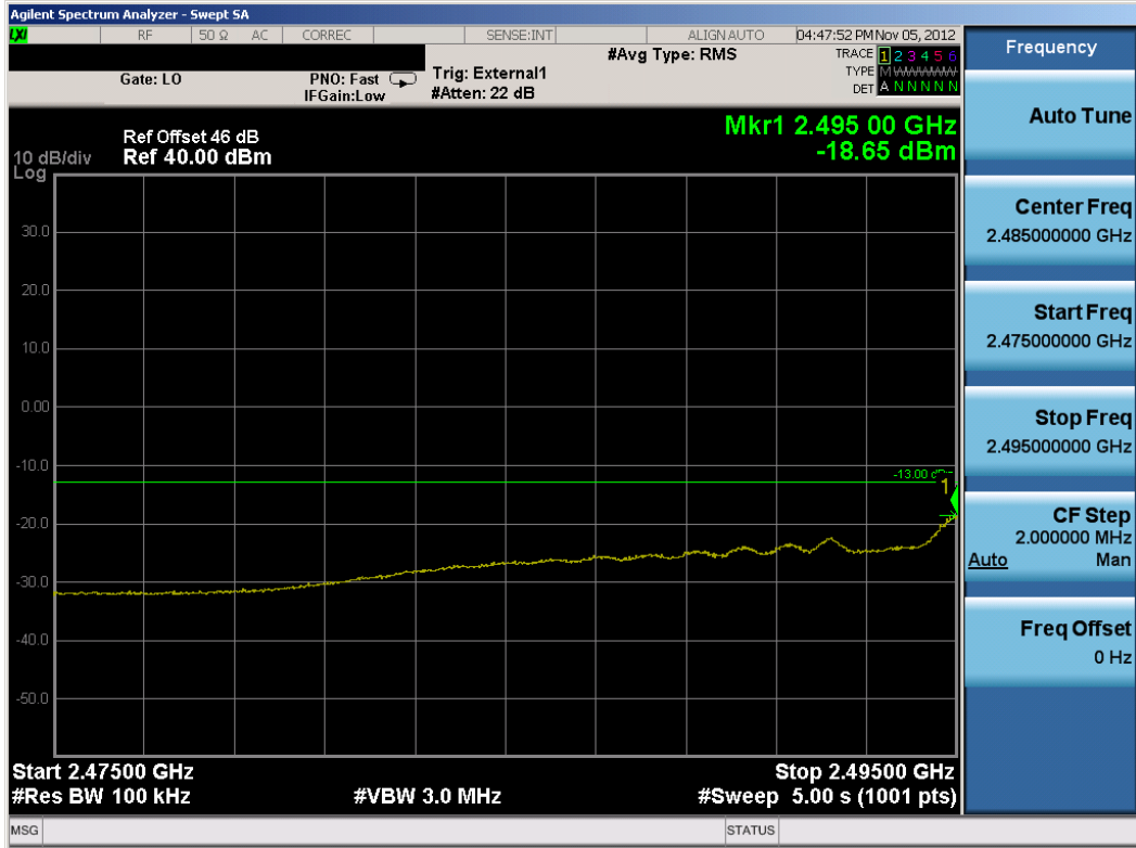
Plot 8-52. Lower Extended Channel Edge Plot (TD-LTE Mode – Low Channel)
