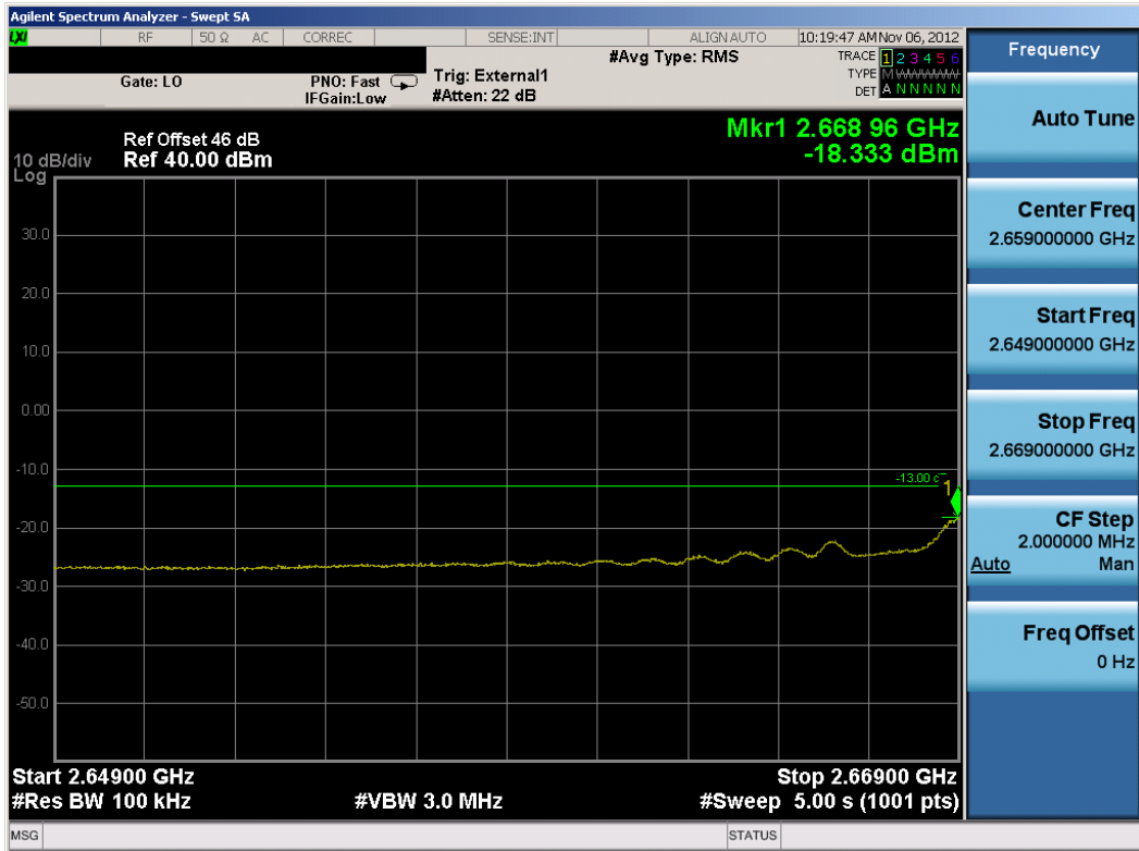
Plot 8-191. Lower Extended Channel Edge Plot (TD-LTE Mode – High Channel)
