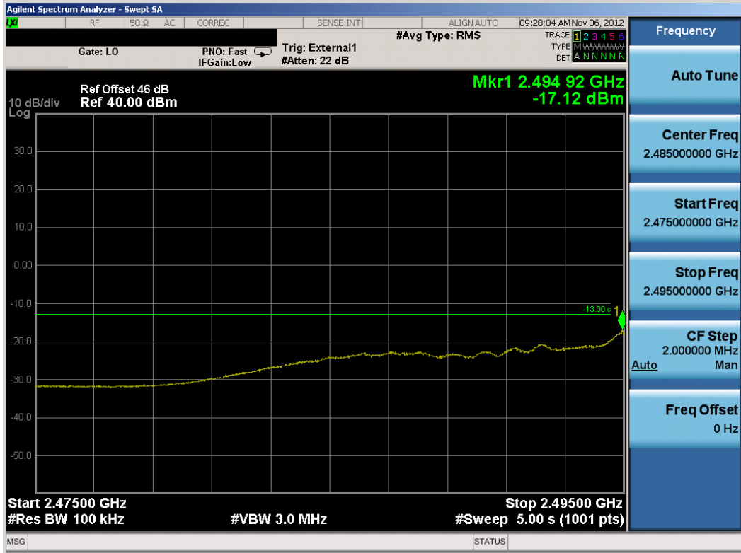
Plot 8-148. Lower Extended Channel Edge Plot (TD-LTE Mode – Low Channel)
