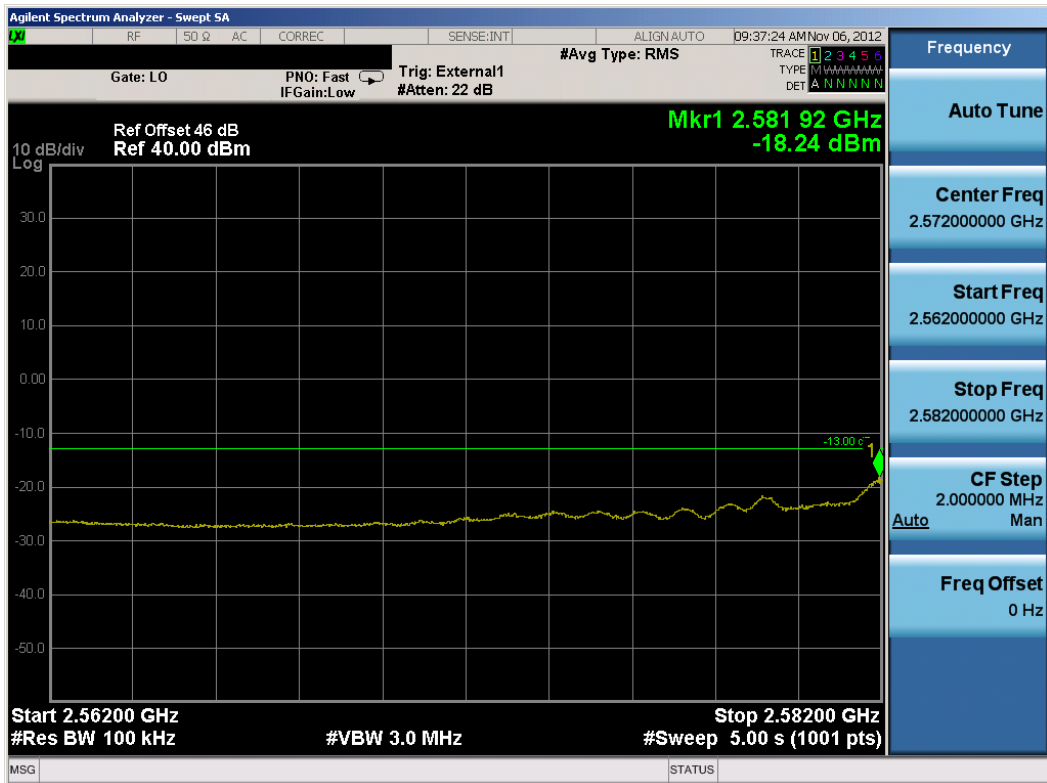
Plot 8-153. Lower Extended Channel Edge Plot (TD-LTE Mode – Mid Channel)
