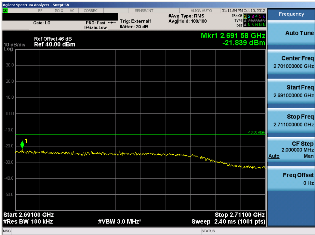
Plot 7-198. Upper Extended Channel Edge Plot (WiMAX Mode – High Channel)
