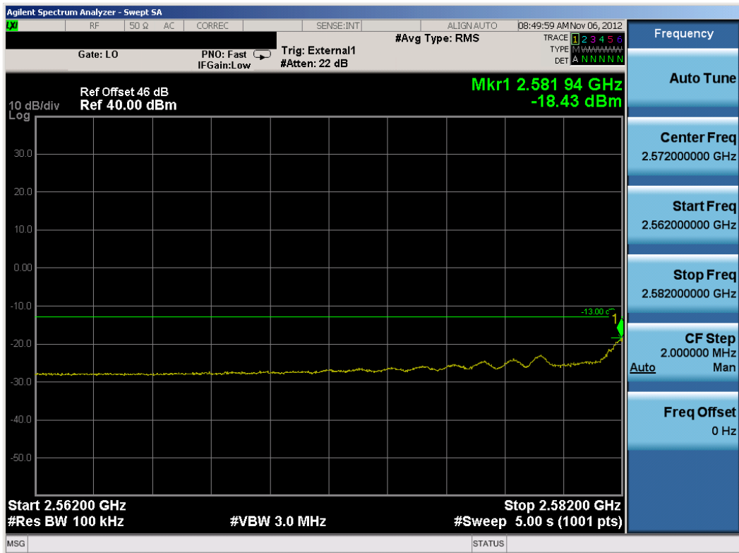
Plot 8-9. Lower Extended Channel Edge Plot (TD-LTE Mode – Mid Channel)
