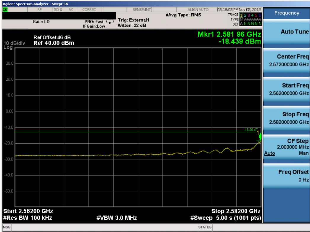
Plot 8-73. Lower Extended Channel Edge Plot (TD-LTE Mode – Mid Channel)
