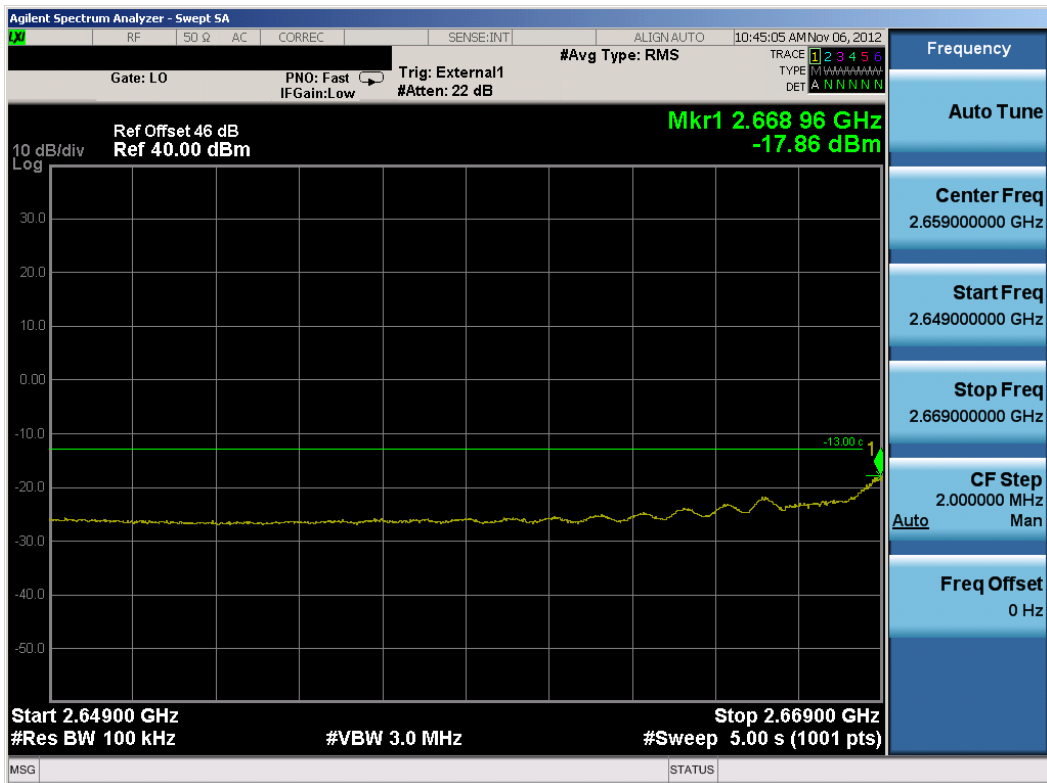
Plot 8-63. Lower Extended Channel Edge Plot (TD-LTE Mode – High Channel)
