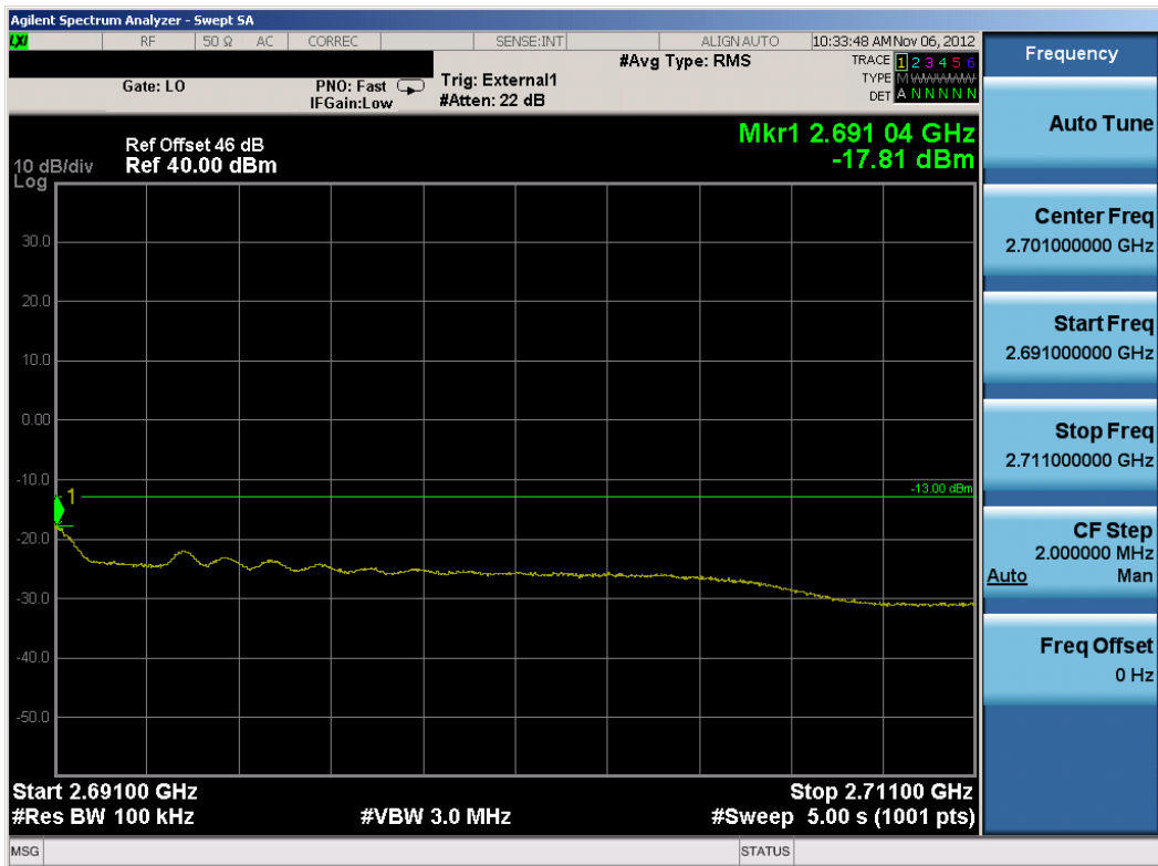
Plot 8-144. Upper Extended Channel Edge Plot (TD-LTE Mode – High Channel)
