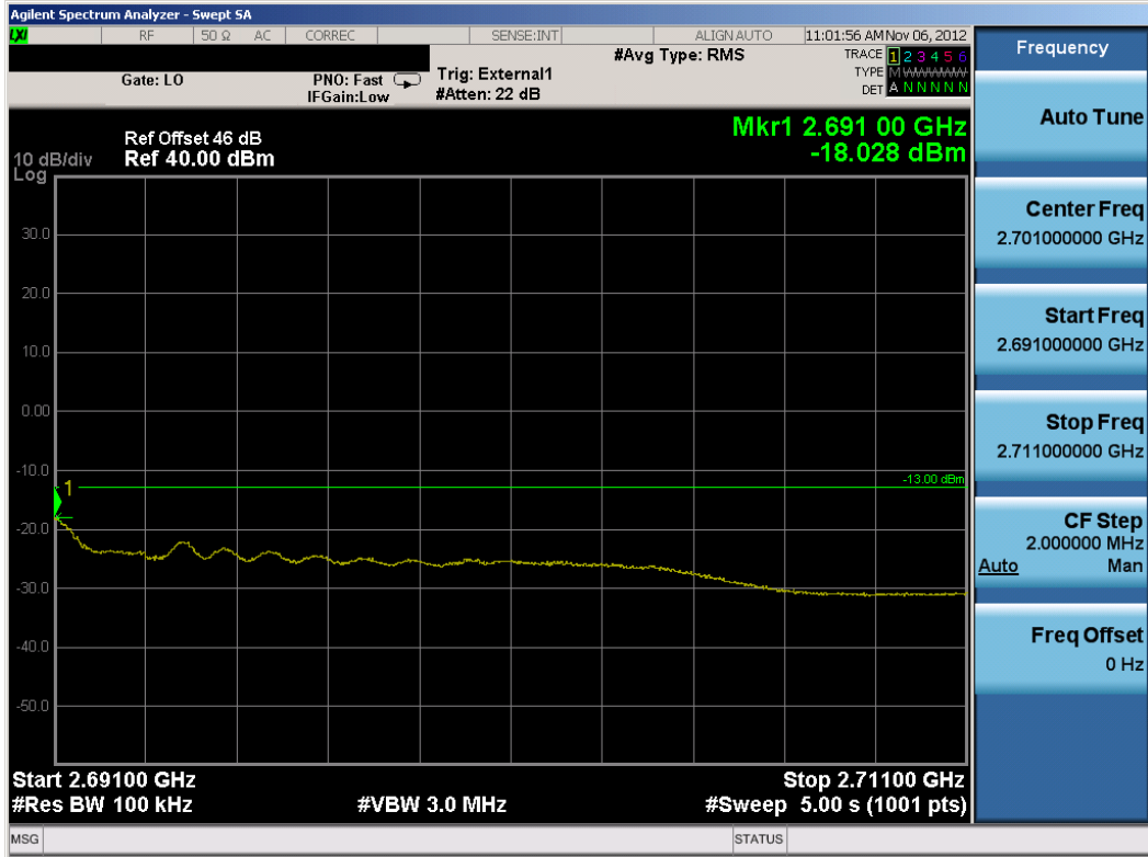
Plot 8-16. Upper Extended Channel Edge Plot (TD-LTE Mode – High Channel)
