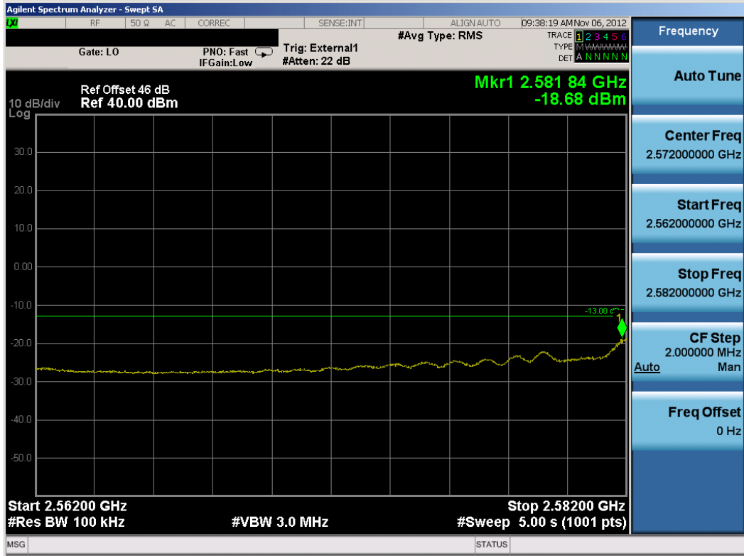
Plot 8-169. Lower Extended Channel Edge Plot (TD-LTE Mode – Mid Channel)
