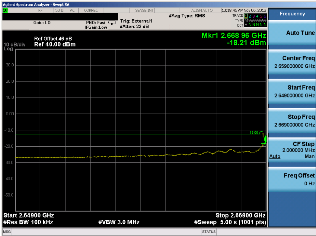
Plot 8-175. Lower Extended Channel Edge Plot (TD-LTE Mode – High Channel)
