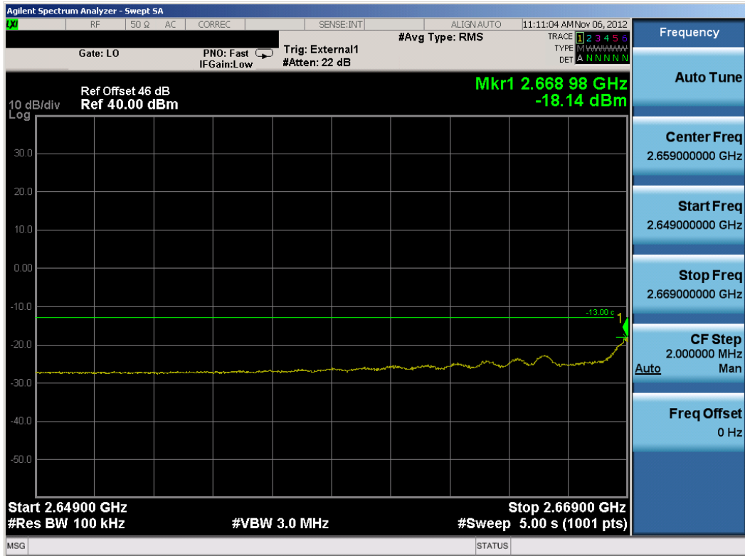
Plot 8-47. Lower Extended Channel Edge Plot (TD-LTE Mode – High Channel)
