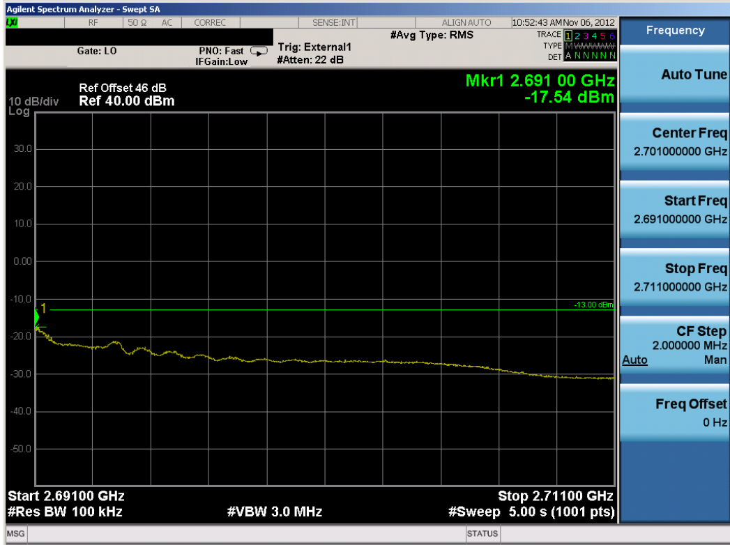
Plot 8-64. Upper Extended Channel Edge Plot (TD-LTE Mode – High Channel)
