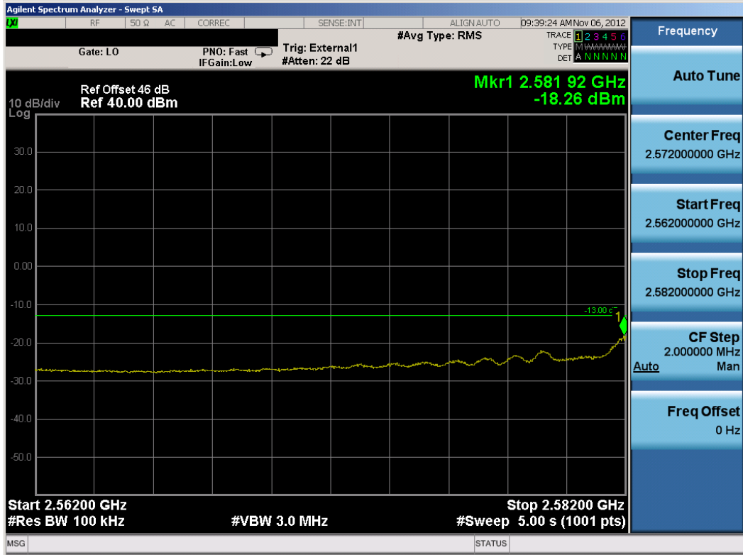
Plot 8-185. Lower Extended Channel Edge Plot (TD-LTE Mode – Mid Channel)
