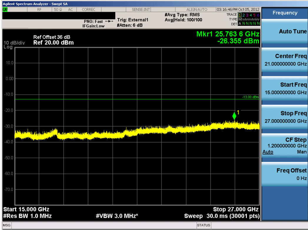
Plot 7-79. Conducted Spurious Plot (WiMAX Mode – Mid Channel)
