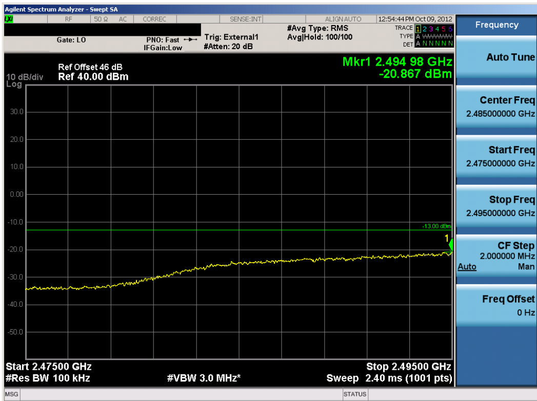
Plot 7-130. Lower Extended Channel Edge Plot (WiMAX Mode – Low Channel)
