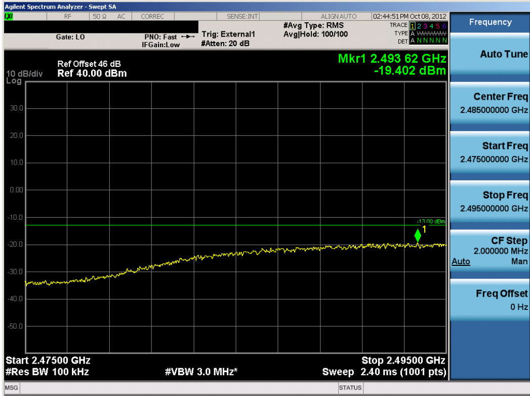
Plot 7-4. Lower Extended Channel Edge Plot (WiMAX Mode – Low Channel)
