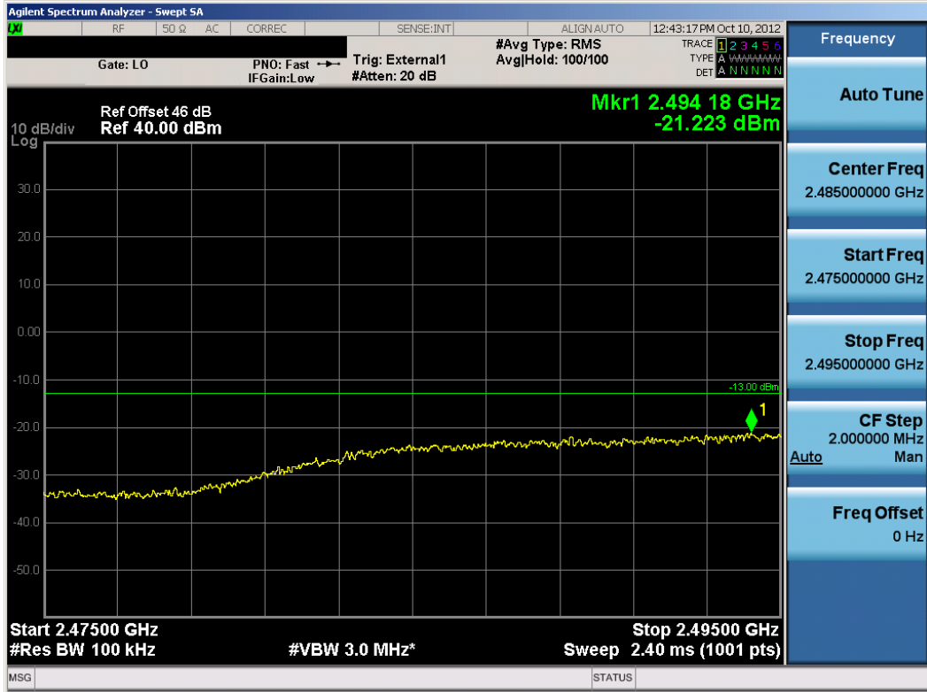
Plot 7-166. Lower Extended Channel Edge Plot (WiMAX Mode – Low Channel)
