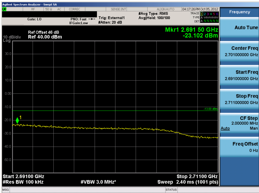
Plot 7-108. Upper Extended Channel Edge Plot (WiMAX Mode – High Channel)
