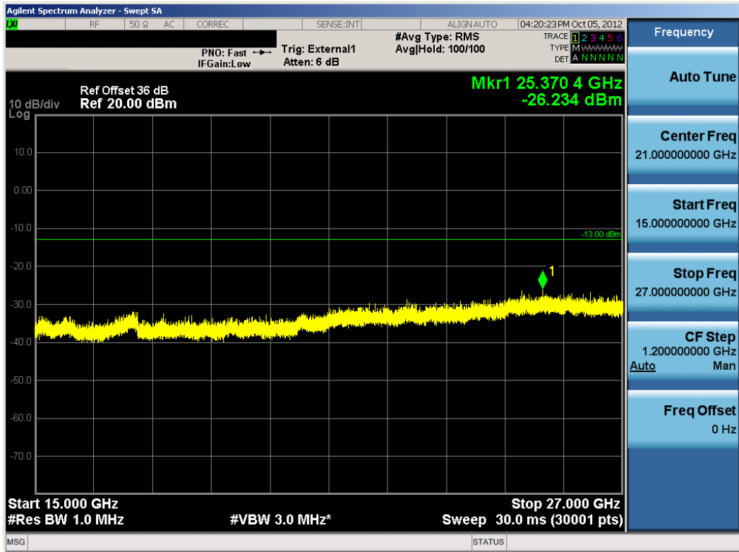
Plot 7-105. Conducted Spurious Plot (WiMAX Mode – High Channel)
