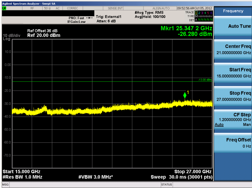
Plot 7-56. Conducted Spurious Plot (WiMAX Mode – Low Channel)
