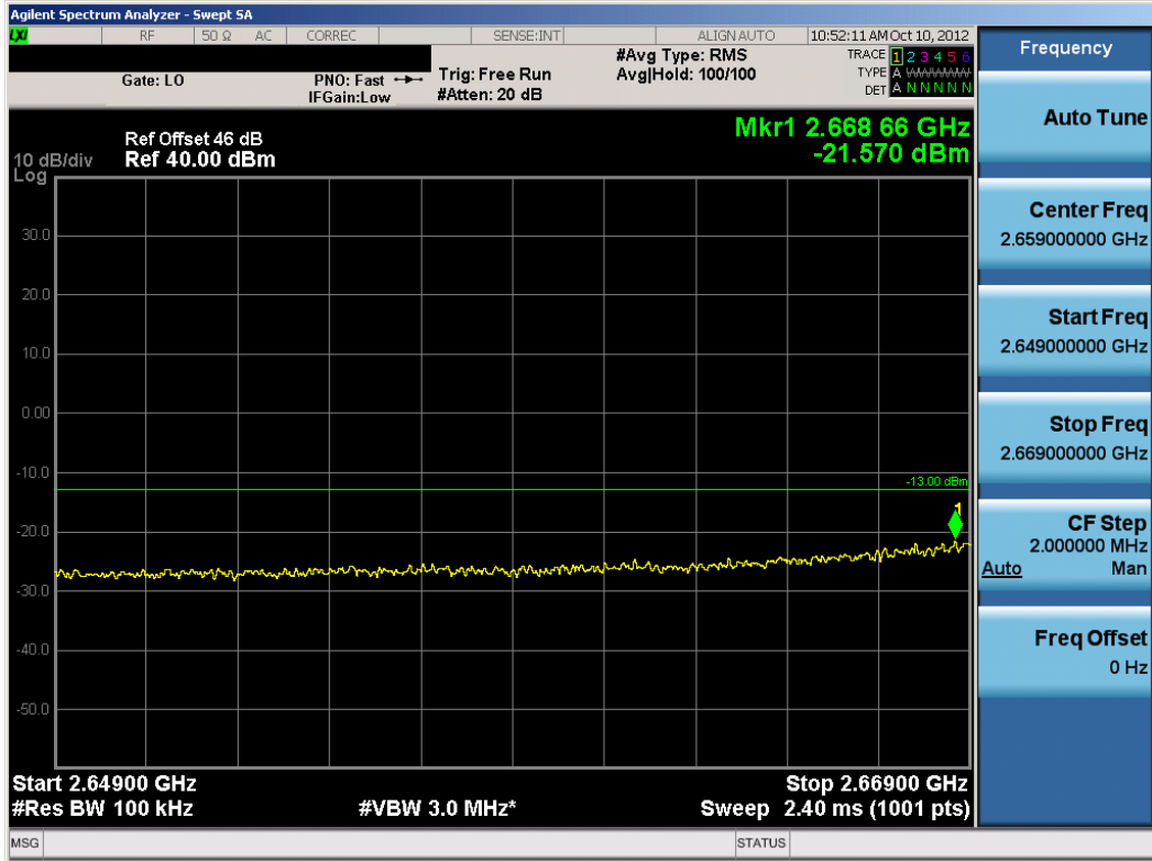
Plot 7-143. Lower Extended Channel Edge Plot (WiMAX Mode – High Channel)
