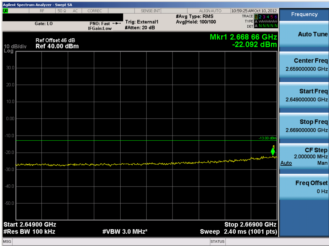
Plot 7-161. Lower Extended Channel Edge Plot (WiMAX Mode – High Channel)
