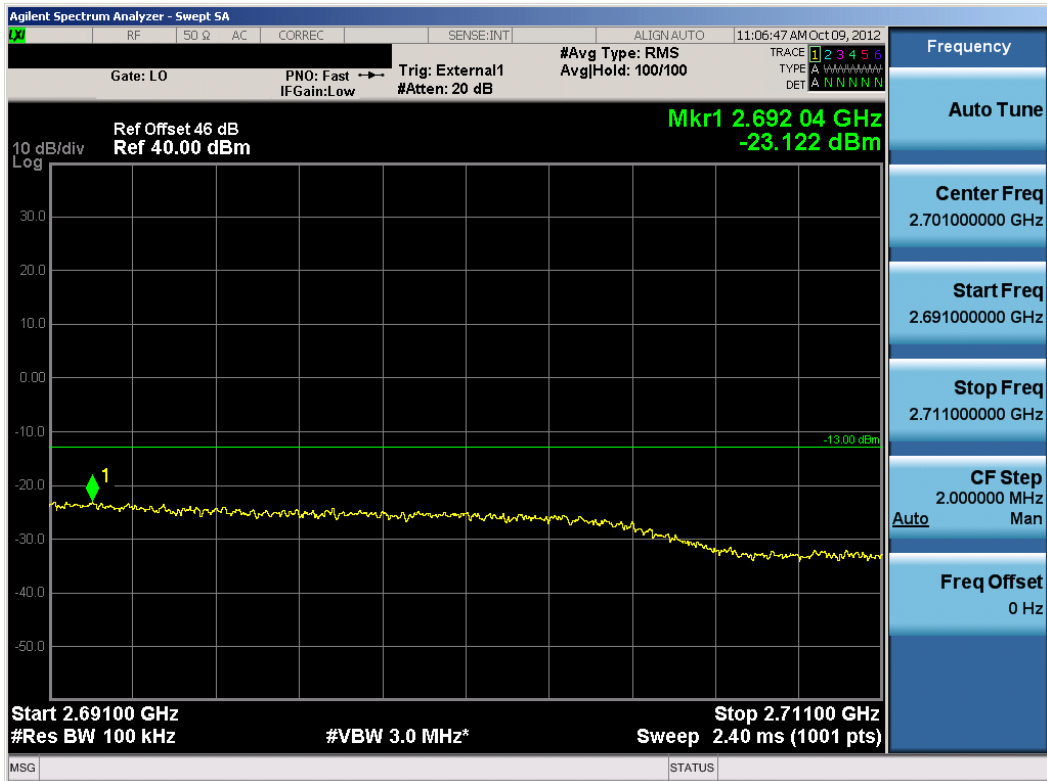
Plot 7-36. Upper Extended Channel Edge Plot (WiMAX Mode – High Channel)
