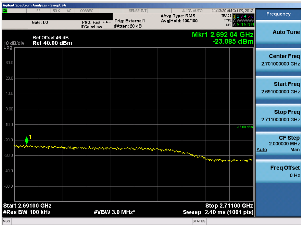
Plot 7-54. Upper Extended Channel Edge Plot (WiMAX Mode – High Channel)
