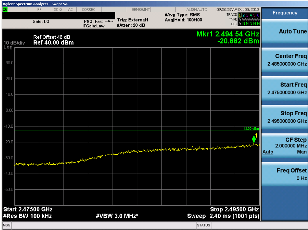
Plot 7-58. Lower Extended Channel Edge Plot (WiMAX Mode - Low Channel)
