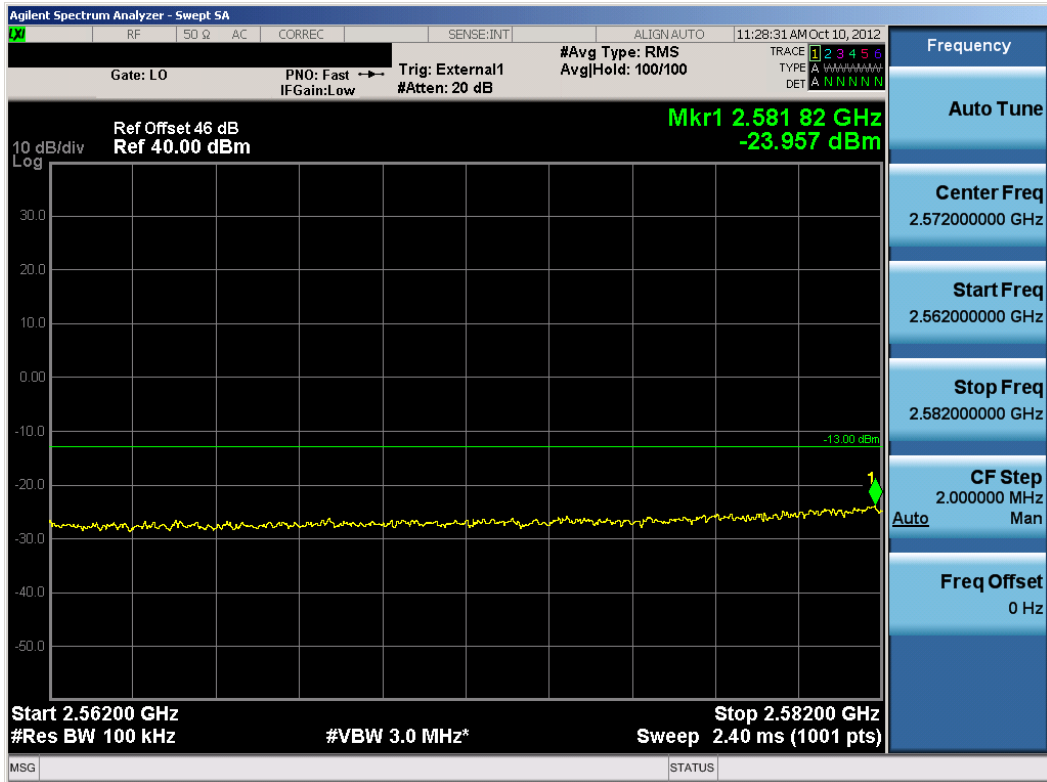
Plot 7-135. Lower Extended Channel Edge Plot (WiMAX Mode – Mid Channel)
