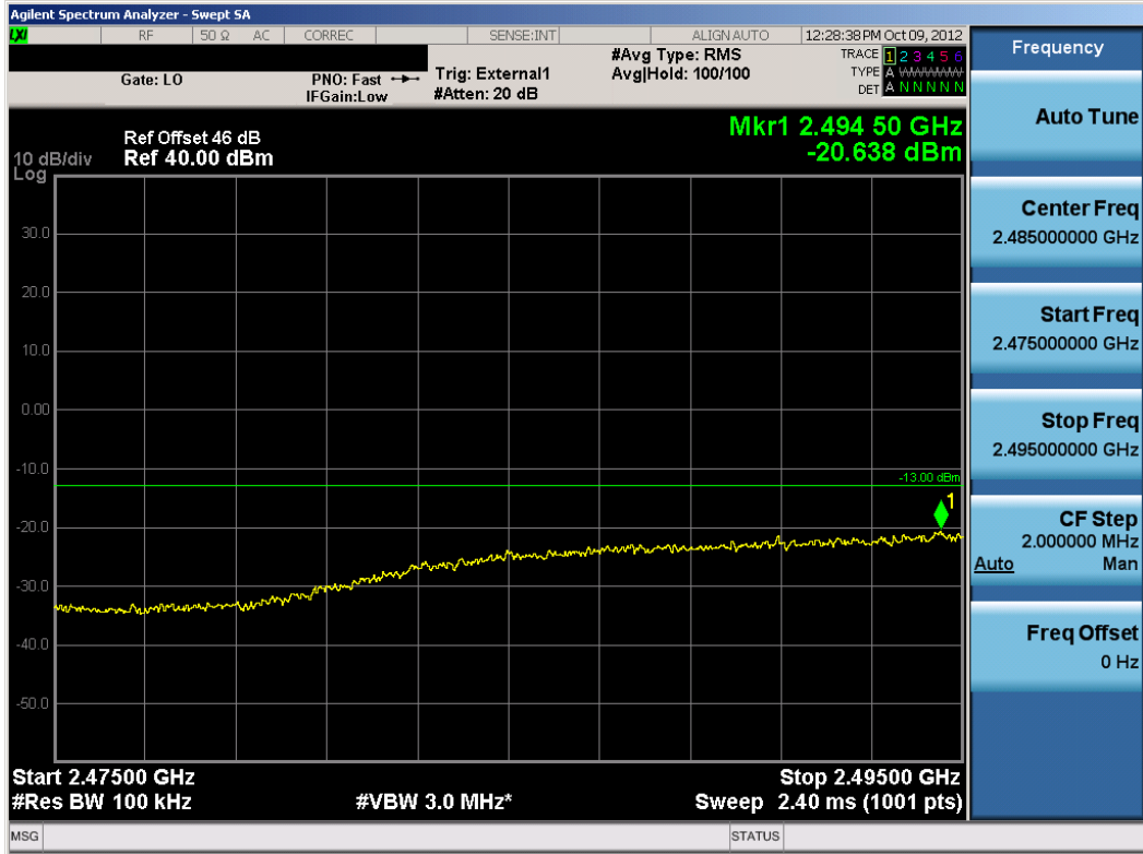
Plot 7-112. Lower Extended Channel Edge Plot (WiMAX Mode – Low Channel)
