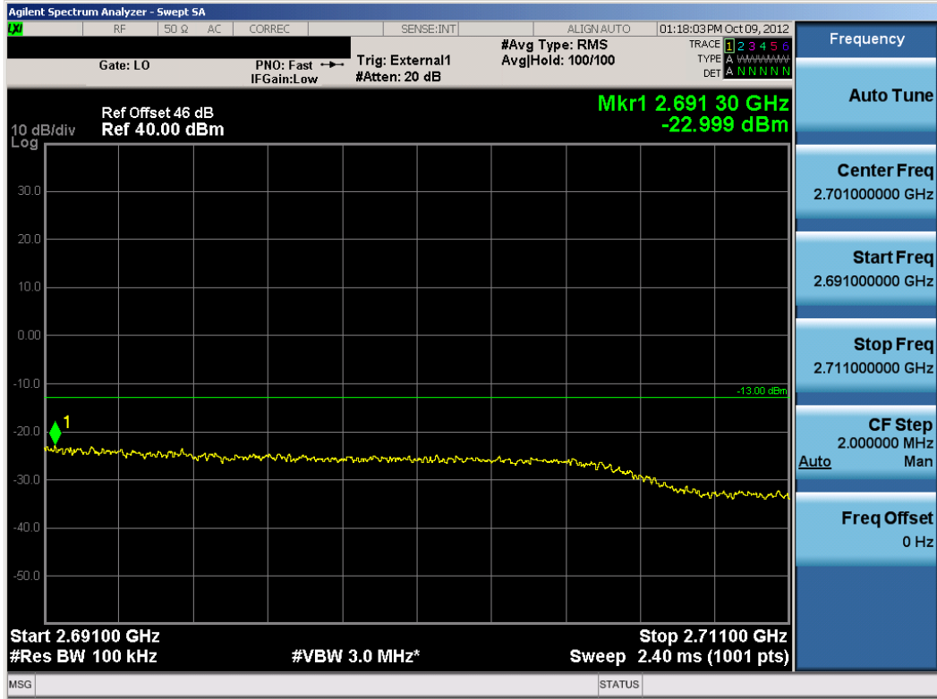
Plot 7-126. Upper Extended Channel Edge Plot (WiMAX Mode – High Channel)
