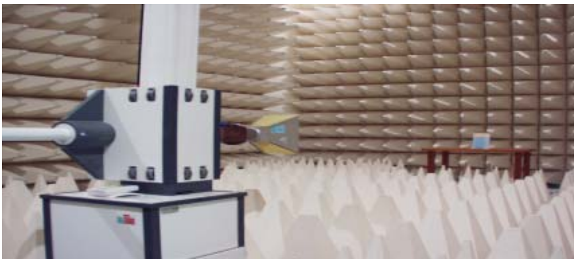
Figure2. Photograph of 3m Fully Anechoic Chamber
