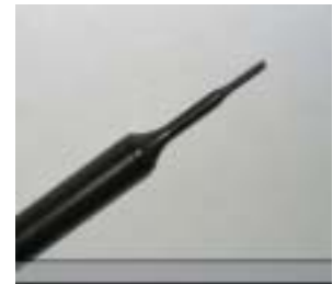
Figure 3.4 Probe Thick-Film Technique
