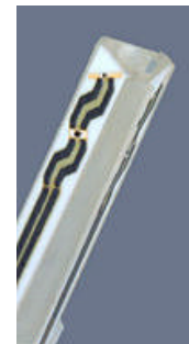
Figure 3.4 Probe Thick-Film Technique
