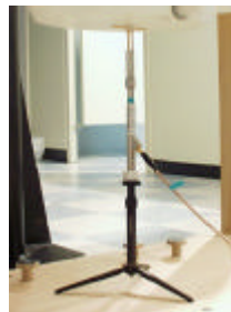
Figure 7.1 Dipole Validation Test Setup
