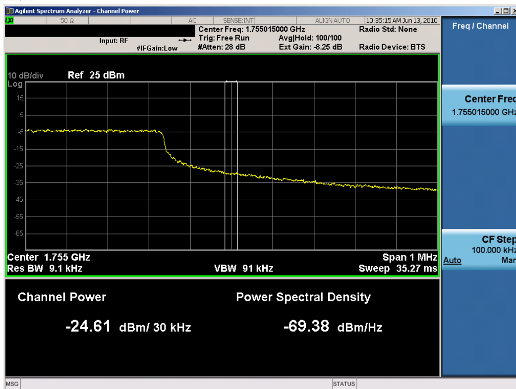
Plot 7-27. Band Edge Plot (3MHz BW, QPSK, AWS Band – High Channel)
