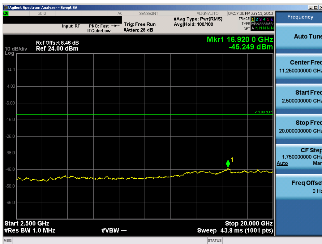
Plot 8-6. Conducted Spurious Plot (3MHz BW, QPSK, PCS Band – Mid Channel)
