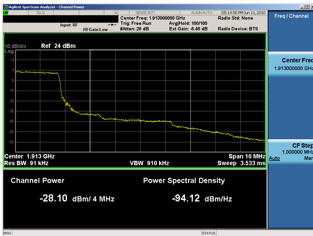
Plot 8-42. 4MHz Span Plot (5MHz BW, QPSK, PCS Band – High Channel)
