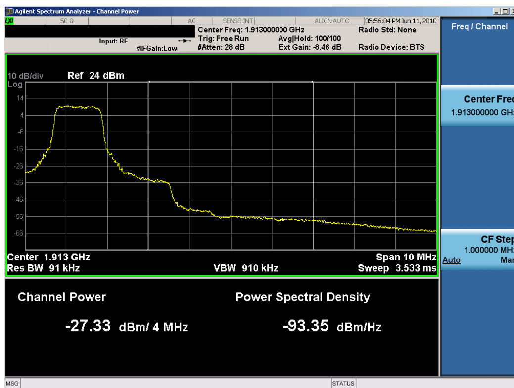
Plot 8-14. 4MHz Span Plot (1.4MHz BW, QPSK, PCS Band – High Channel)
