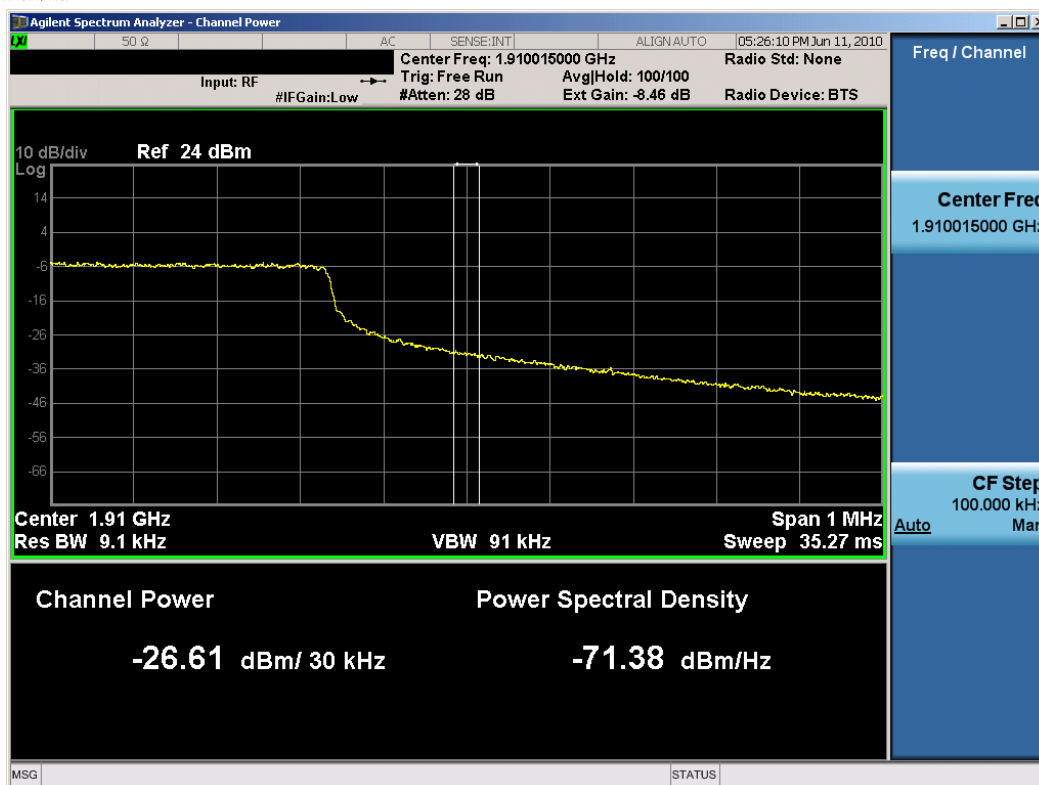
Plot 8-27. Band Edge Plot (3MHz BW, QPSK, PCS Band – High Channel)
