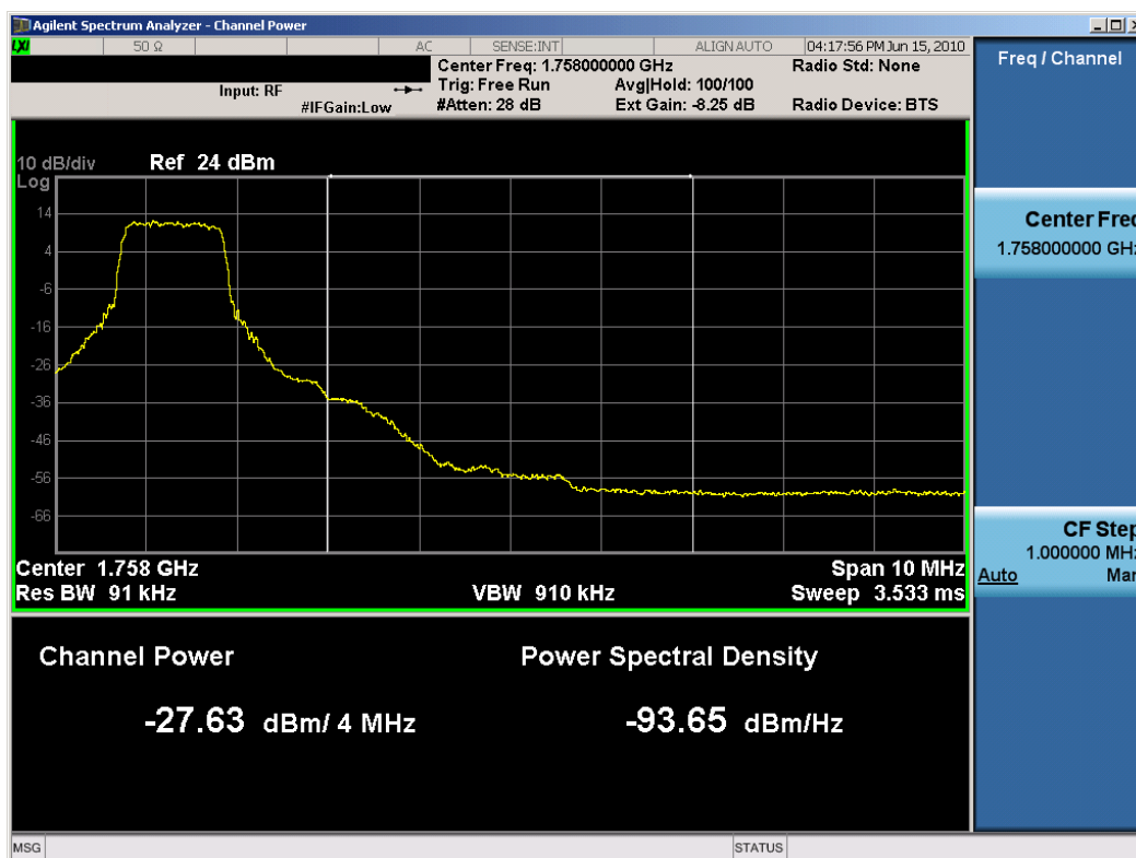
Plot 7-14. 4MHz Span Plot (1.4MHz BW, QPSK, AWS Band – High Channel)
