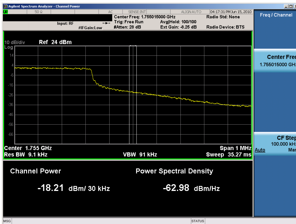
Plot 7-13. Band Edge Plot (1.4MHz BW, QPSK, AWS Band – High Channel)
