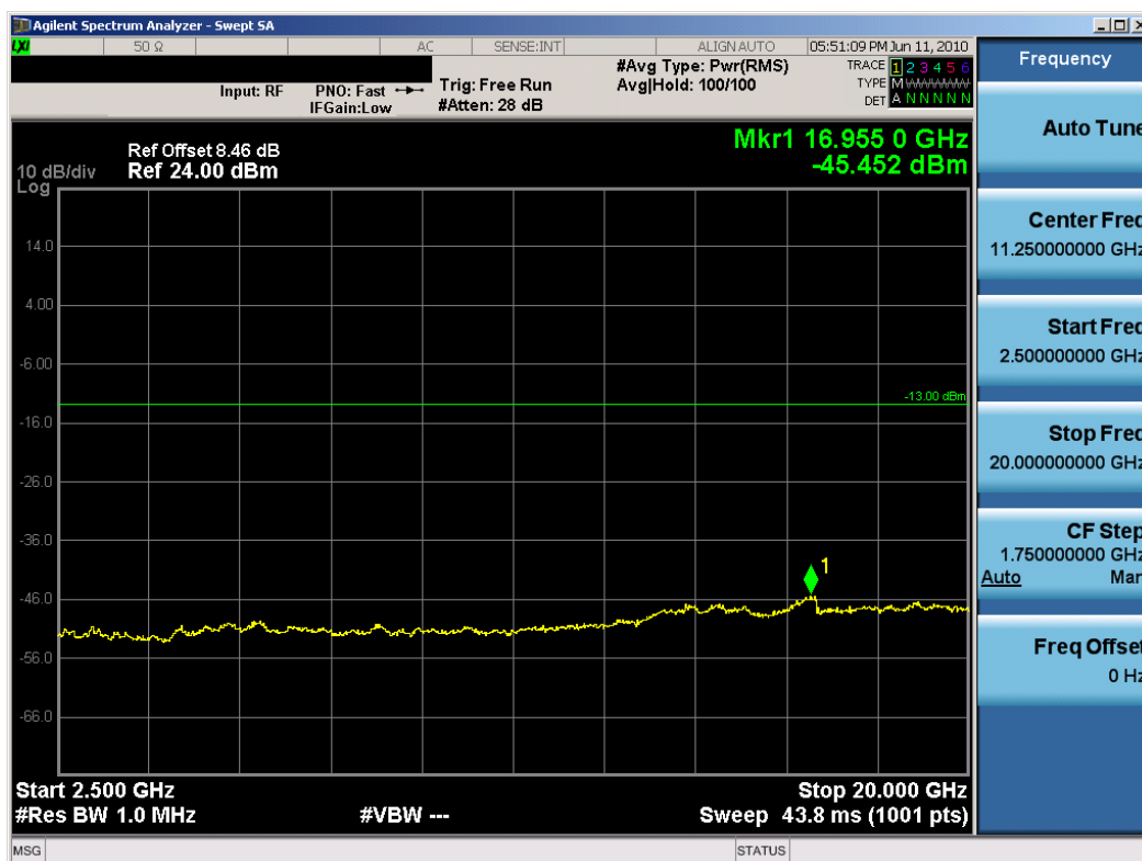
Plot 8-12. Conducted Spurious Plot (1.4MHz BW, QPSK, PCS Band – High Channel)
