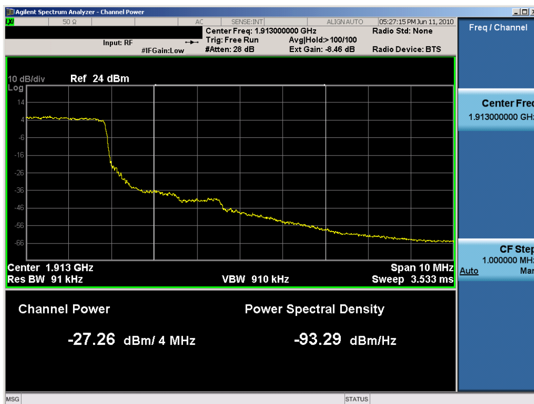
Plot 8-28. 4MHz Span Plot (3MHz BW, QPSK, PCS Band – High Channel)
