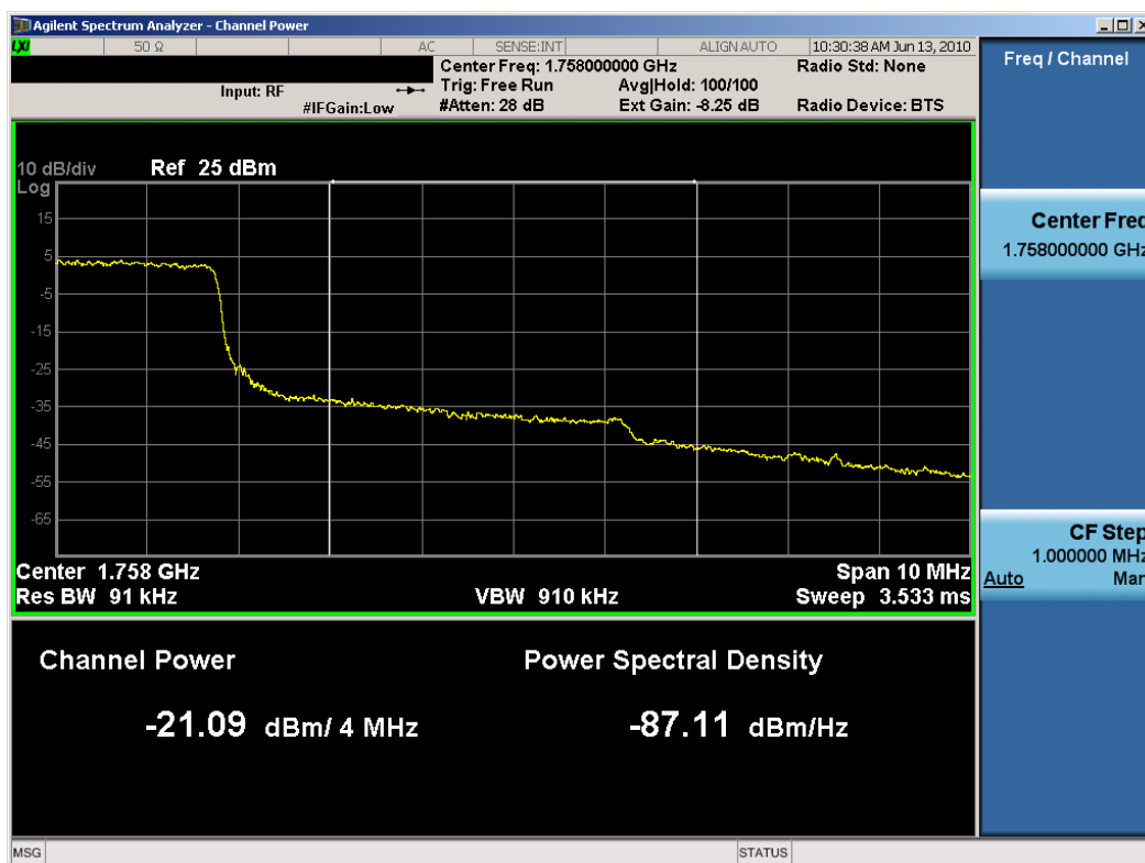
Plot 7-42. 4MHz Span Plot (5MHz BW, QPSK, AWS Band – High Channel)
