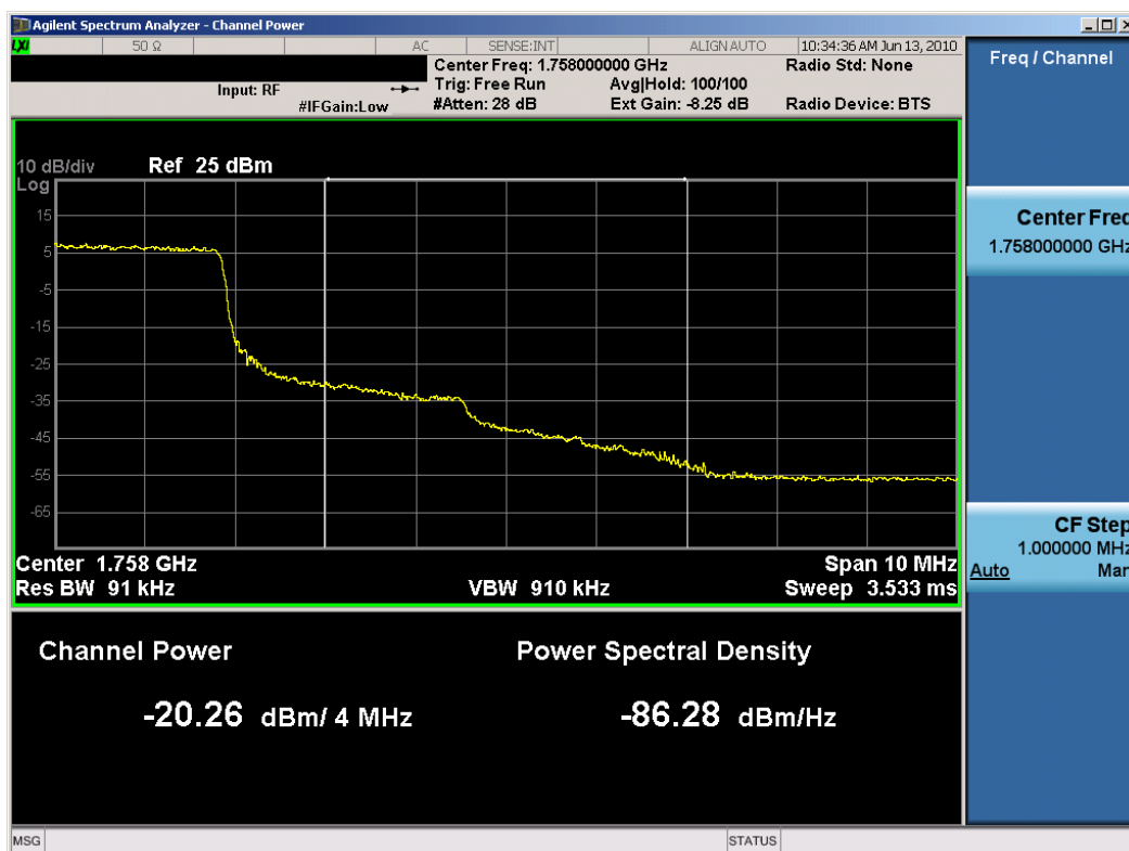
Plot 7-28. 4MHz Span Plot (3MHz BW, QPSK, AWS Band – High Channel)
