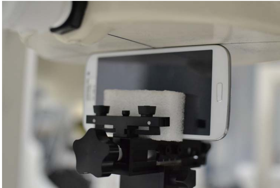
SAR Test Setup Photo 9 – Right Edge at 0.0 cm
