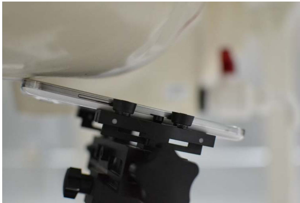
SAR Test Setup Photo 2 – Right Tilt
