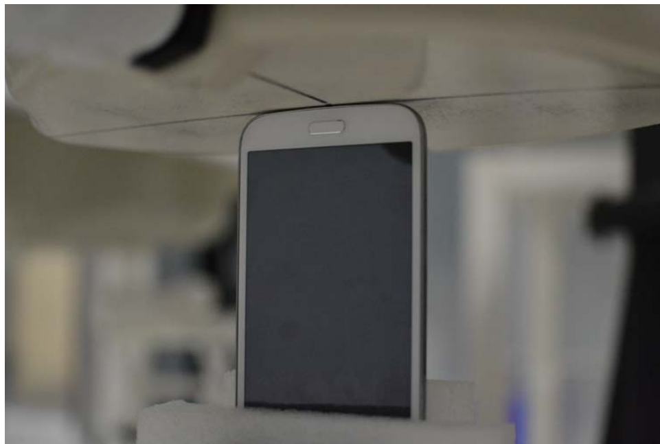
SAR Test Setup Photo 8 –Bottom Edge at 0.0 cm
