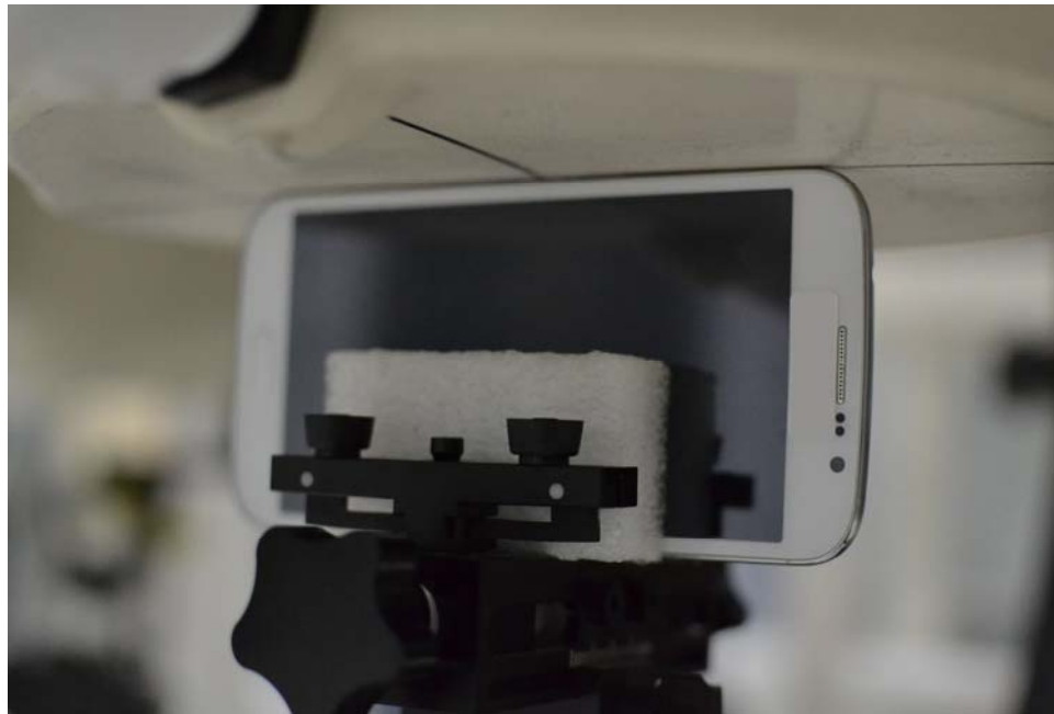
SAR Test Setup Photo 10 – Left Edge at 0.0 cm
