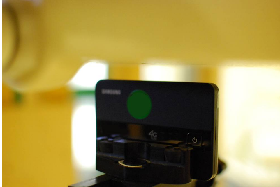
SAR Test Setup Photo 3: Top at 1.0 cm
