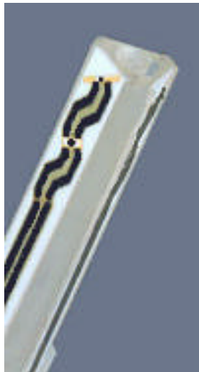
Fig. 5. ET3DV5 E-field Probe
