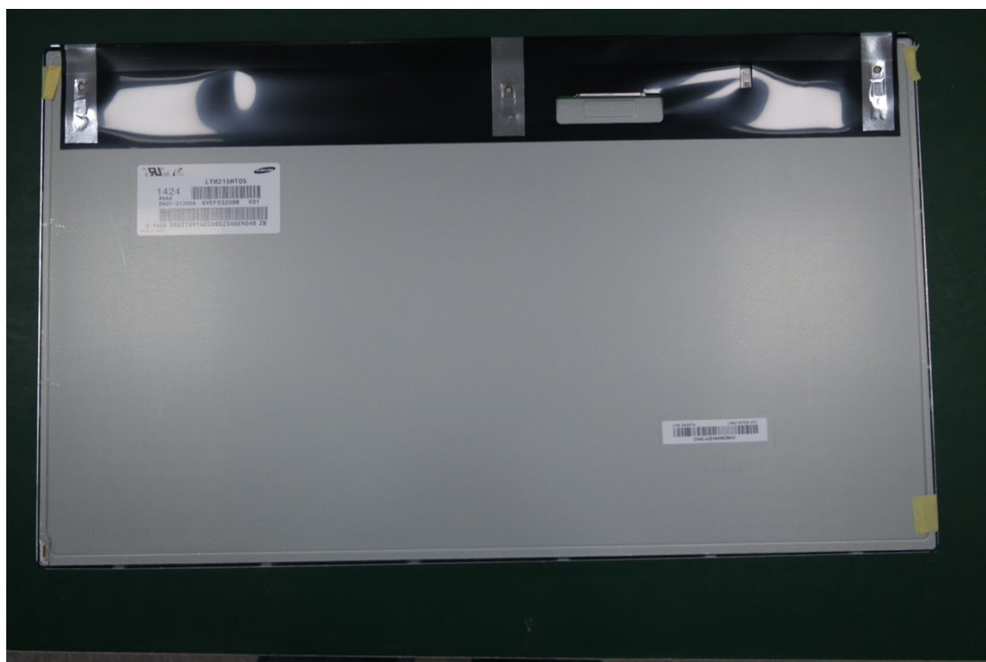
Before change LTM215HT05 rear view
