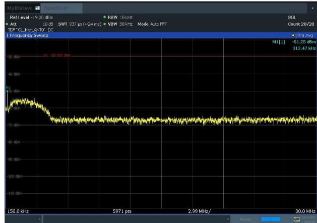
Plot 8-18. Conducted Spurious Emission Plot 150 kHz to 30 MHz (n26_1C_5M+n29_1C_5M+n71_1C_5M_QPSK – Mid, Port 0)
