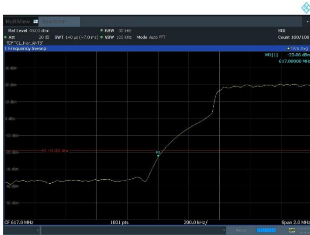
Plot 8-9. Band Edge Emission Plot (n71_1C_15M_64QAM - Low Channel, Port 3)
