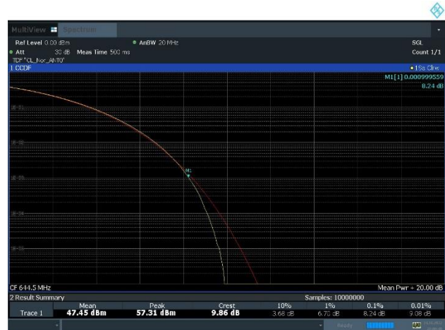
Plot 8-8. Peak To Average Power Ratio Plot (n71_1C_15M_16QAM - High Channel, Port 0)
