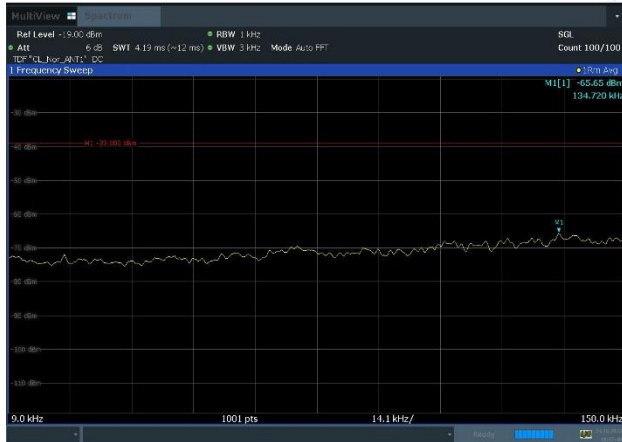
Plot 8-11. Conducted Spurious Emission Plot 9 kHz to 150 kHz (n71_1C_15M_QPSK - Low Channel, Port 1)
