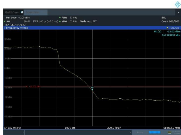
Plot 8-10. Band Edge Emission Plot (n71_1C_15M_16QAM - High Channel, Port 3)
