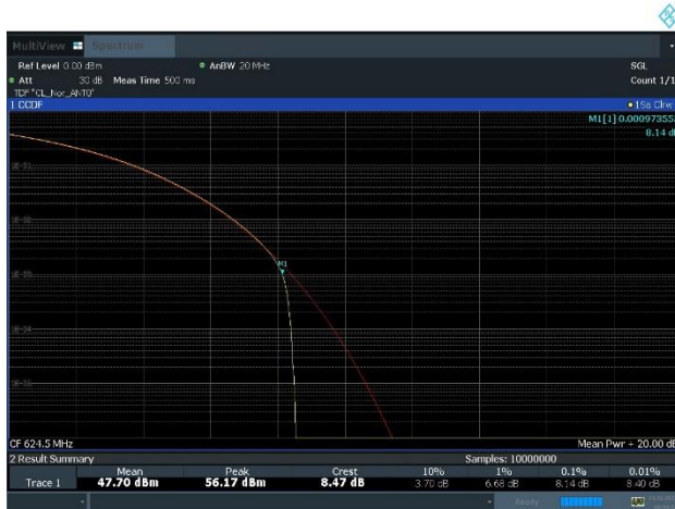
Plot 8-7. Peak To Average Power Ratio Plot (n71_1C_15M_QPSK - Low Channel, Port 0)
