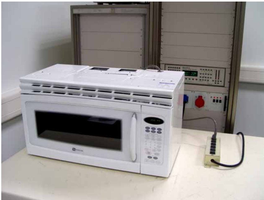
Fig. 2 Test Setup for Input power
