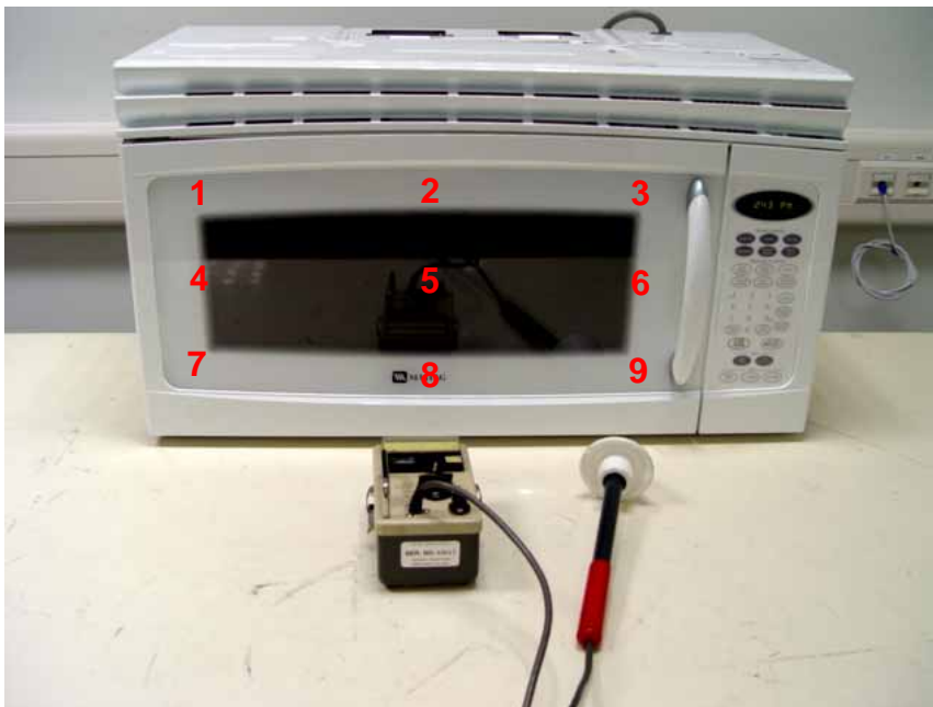
Fig. 1 Test Setup for Radiation Hazard Measurement
