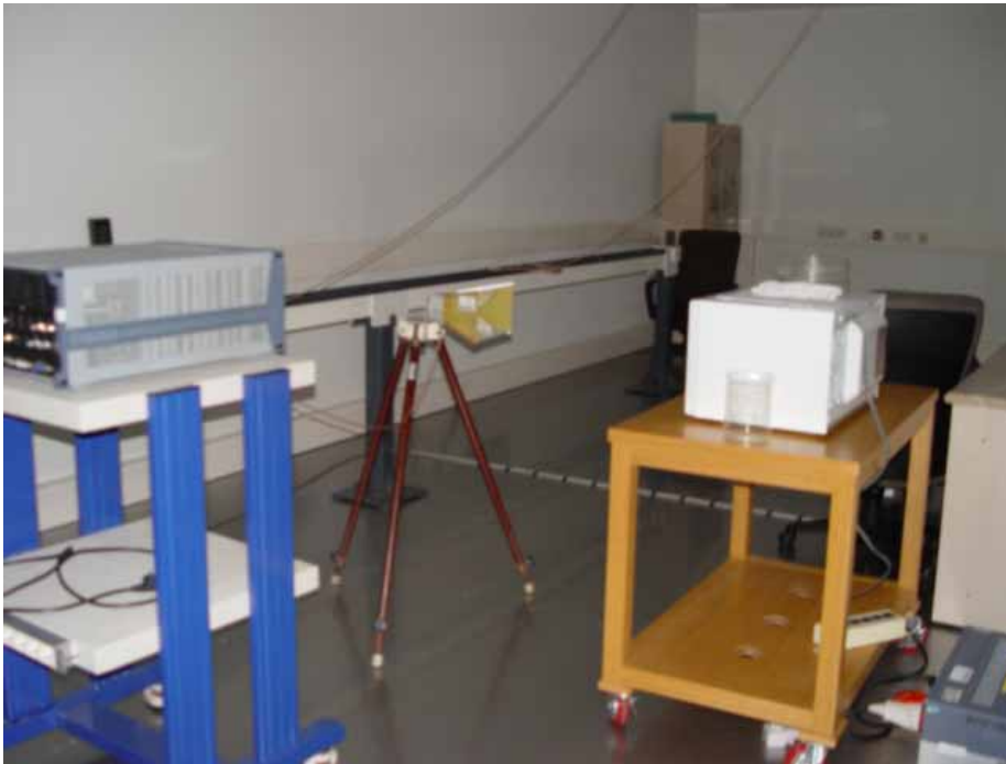
Fig. 4 Operating Frequency Measurements Configuration
