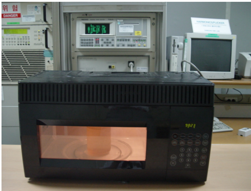
Fig.3 Test Setup for RF output power
