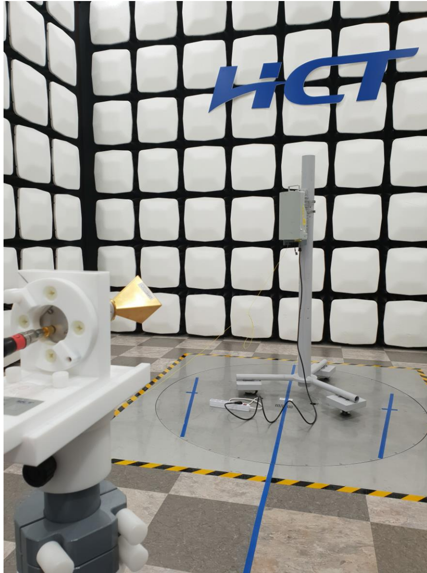
Radiated Test Setup Photo – Spurious (WR-19 Horn Antenna, Lower)
