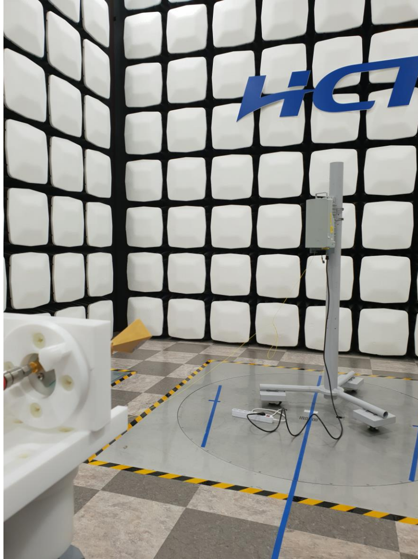
Radiated Test Setup Photo – Spurious (WR-12 Horn Antenna, Upper)
