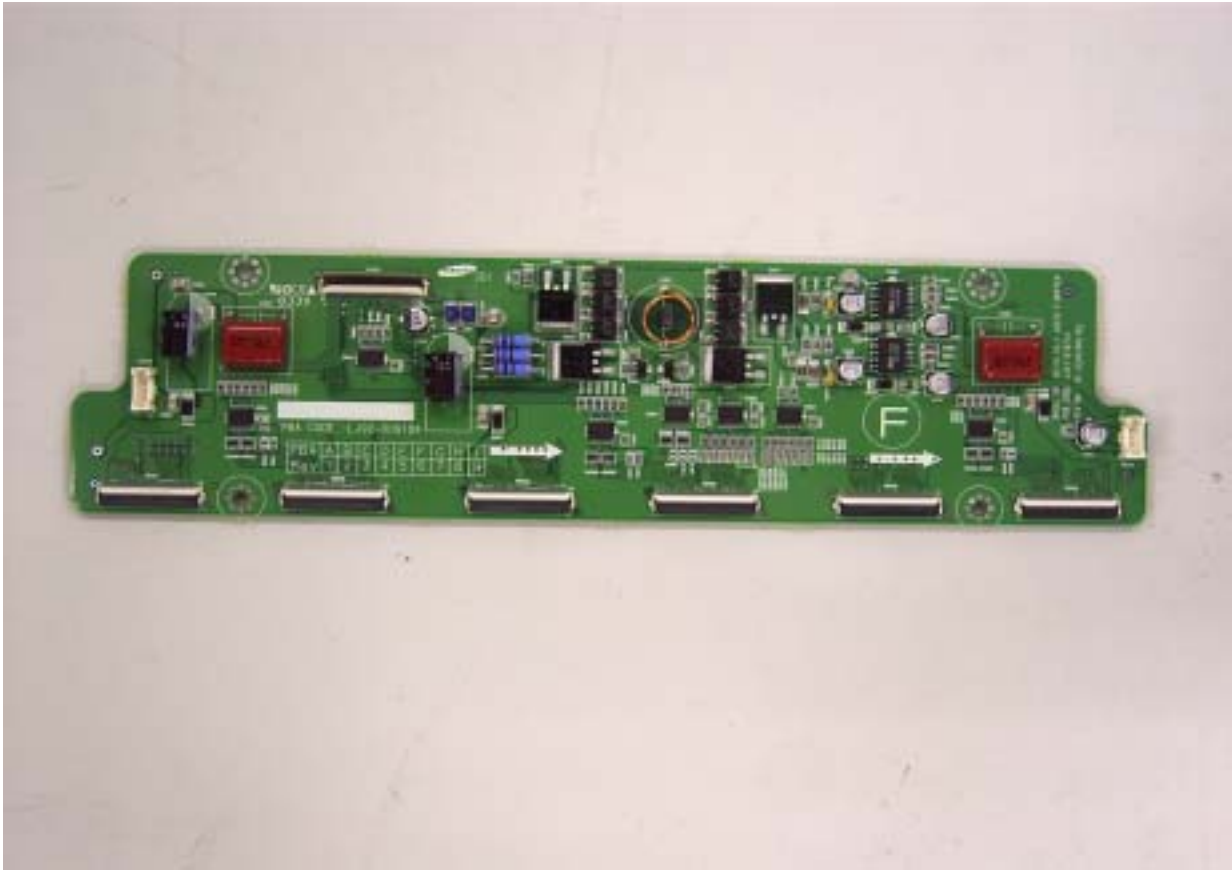
F buffer board top view
