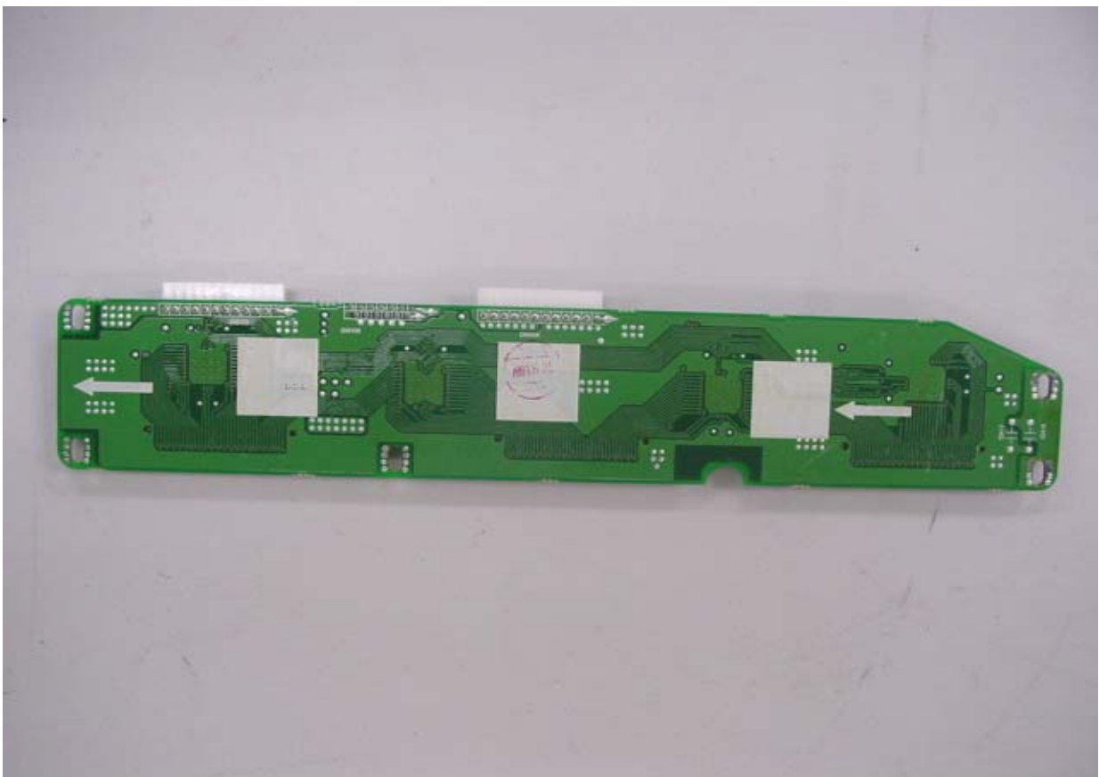
YB upper board bottom view
