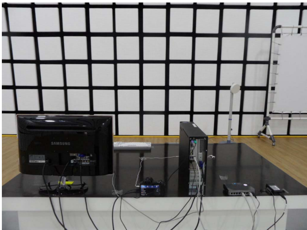
[ Radiated Disturbance for Below 1 GHz – Rear ]
