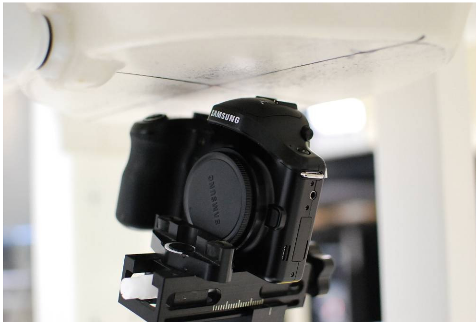
SAR Test Setup Photo 6: Top Edge at 1.0 cm
