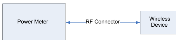
Figure 8-3 Power Measurement Setup
