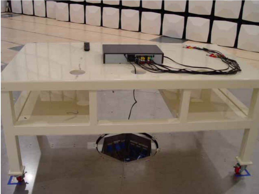
Picture 3. Radiated emission (Rear)
