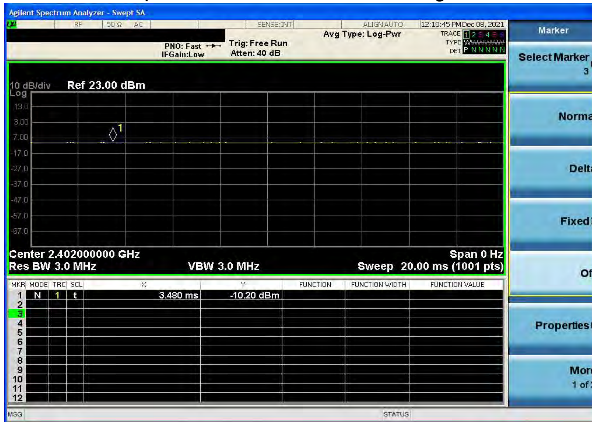
Time-domain plot for Bluetooth transmission signal
