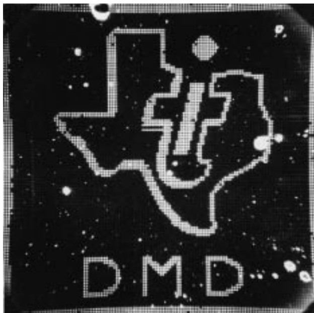
Figure 36. 128 x 128 membrane DMD (first projected image, 1981). Blemishes are examples of “tenting.”
