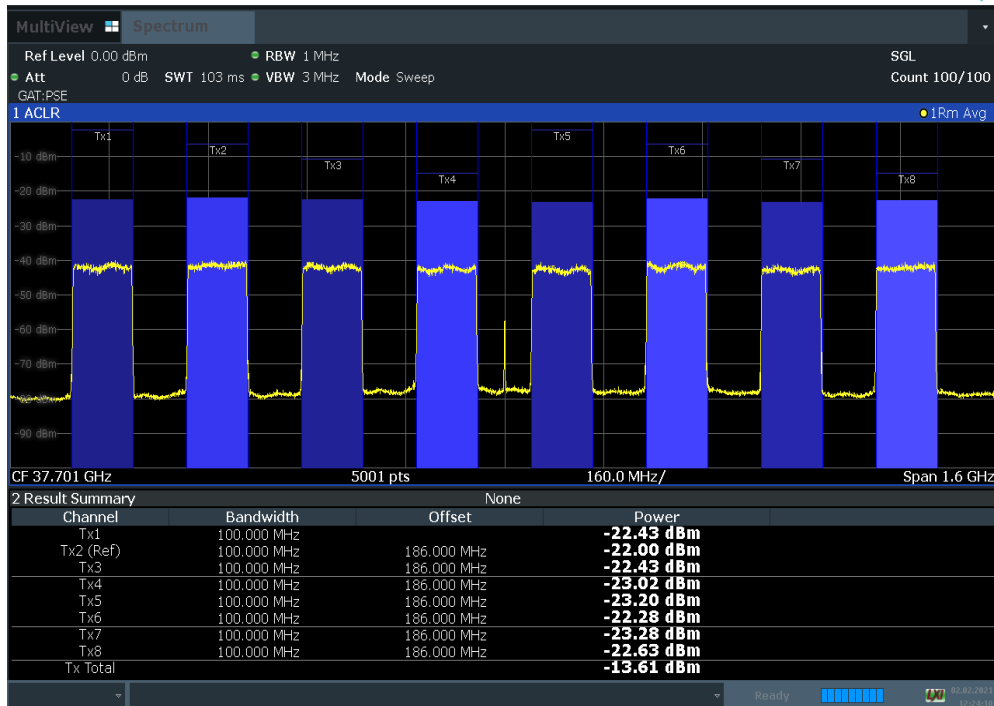
Plot 7-86. Antenna C EIRP Density Plot (100 MHz BW 8CC NC 16QAM Low Channel)
