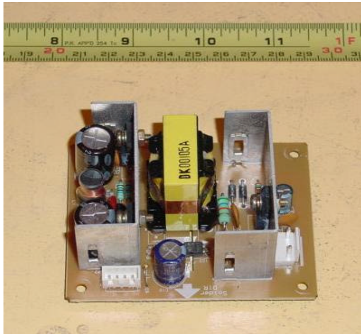
Front of Sub Power Board
