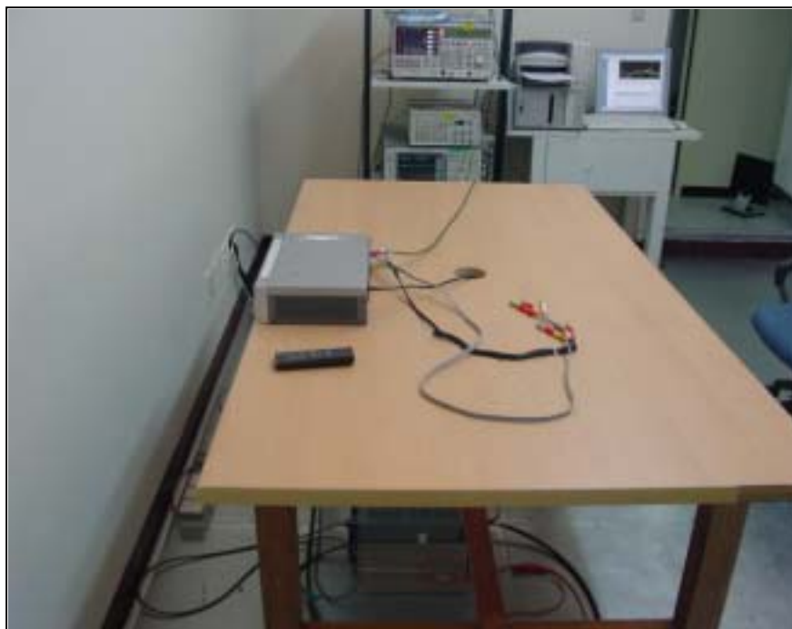
Pic. 2 AC Powerline Conducted Emission [Rear]
