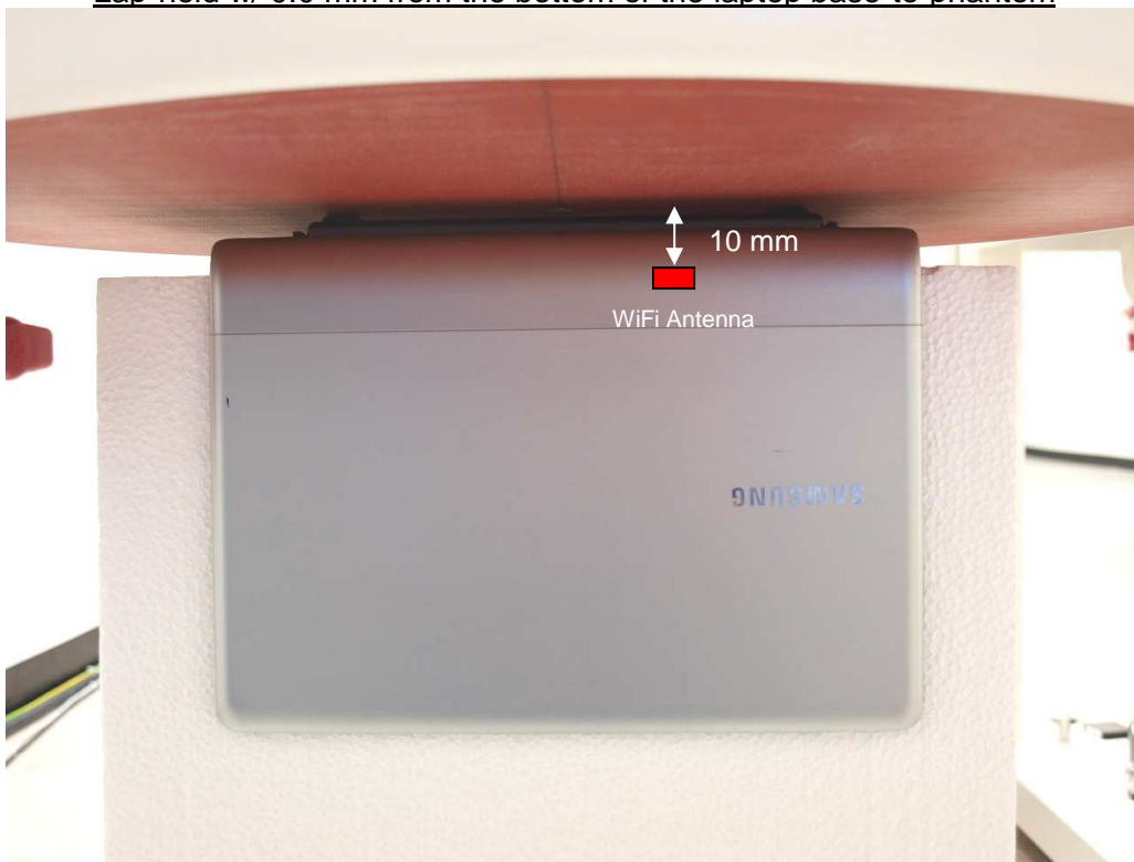
Lap-held w/ 0.0 mm from the bottom of the laptop base-to-phantom
