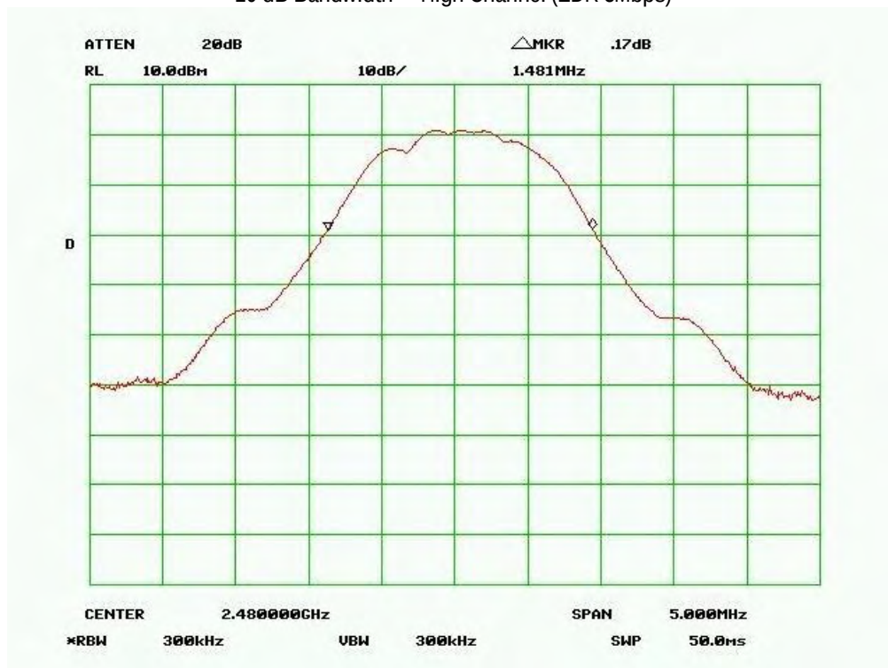
20 dB Bandwidth - High Channel (EDR 3Mbps)
